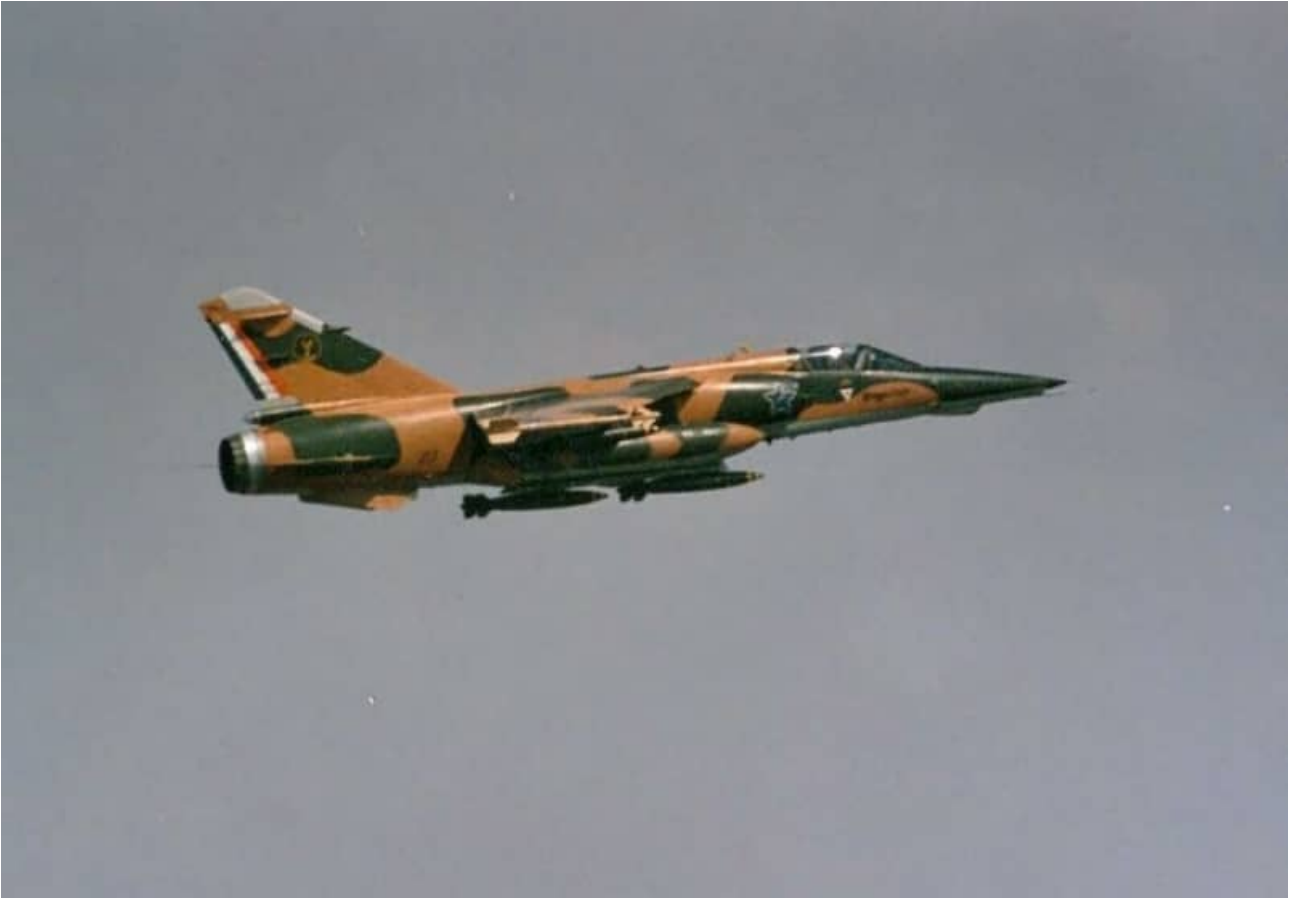
Above : AZ departing on a combat mission carrying six Mk.82 bombs, two V3B missiles and two RP35 external fuel tanks. A heavy load for sure.
