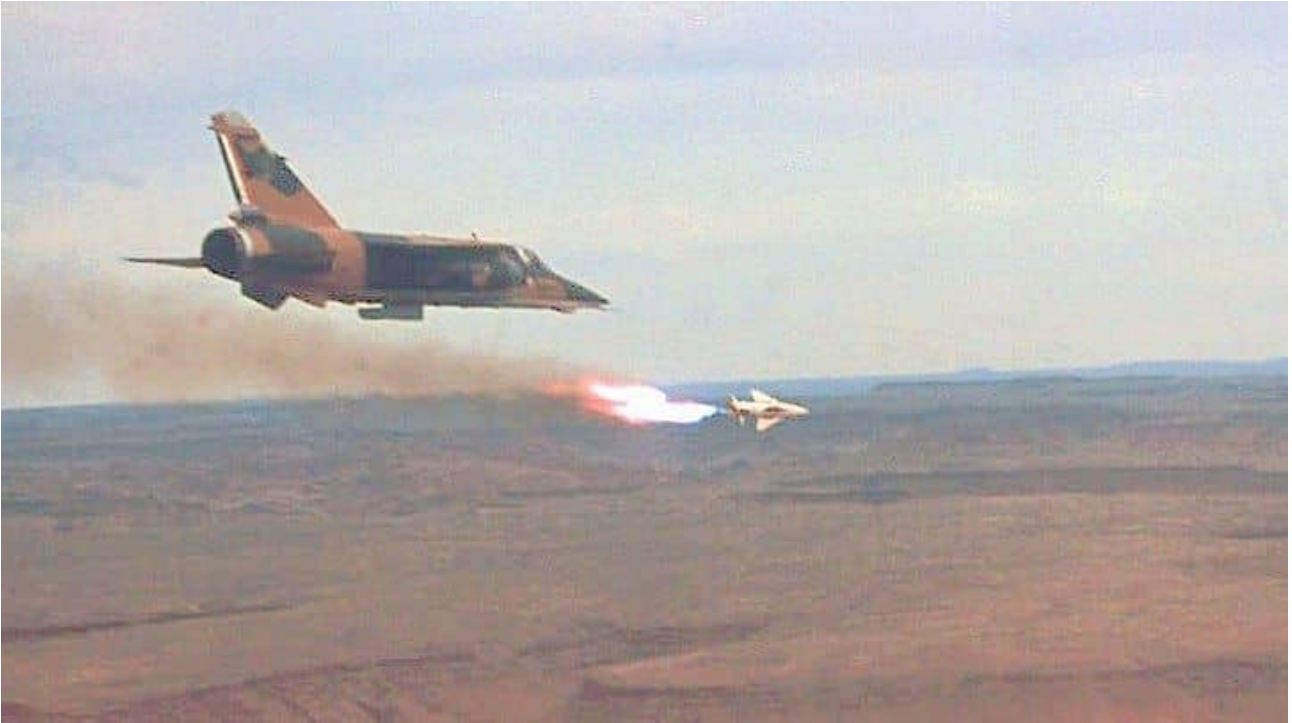
The AZ could carry a single AS30 command guided air-to-ground missile on the fuselage centerline station. Here we see an AS30 departing for its final destination.
