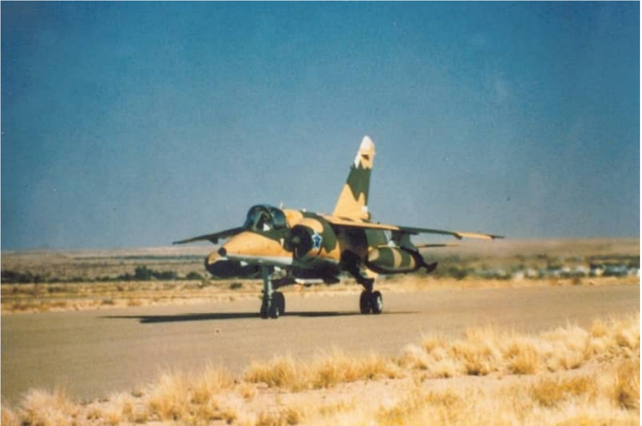
AZ carrying two RP35 external fuel tanks and an empty CLB4 4-bomb carrier on the fuselage centerline station. The tank on the port wing appears to have been painted in the interim colours of dark earth/green – note the tonal difference between the buff and the dark earth.
