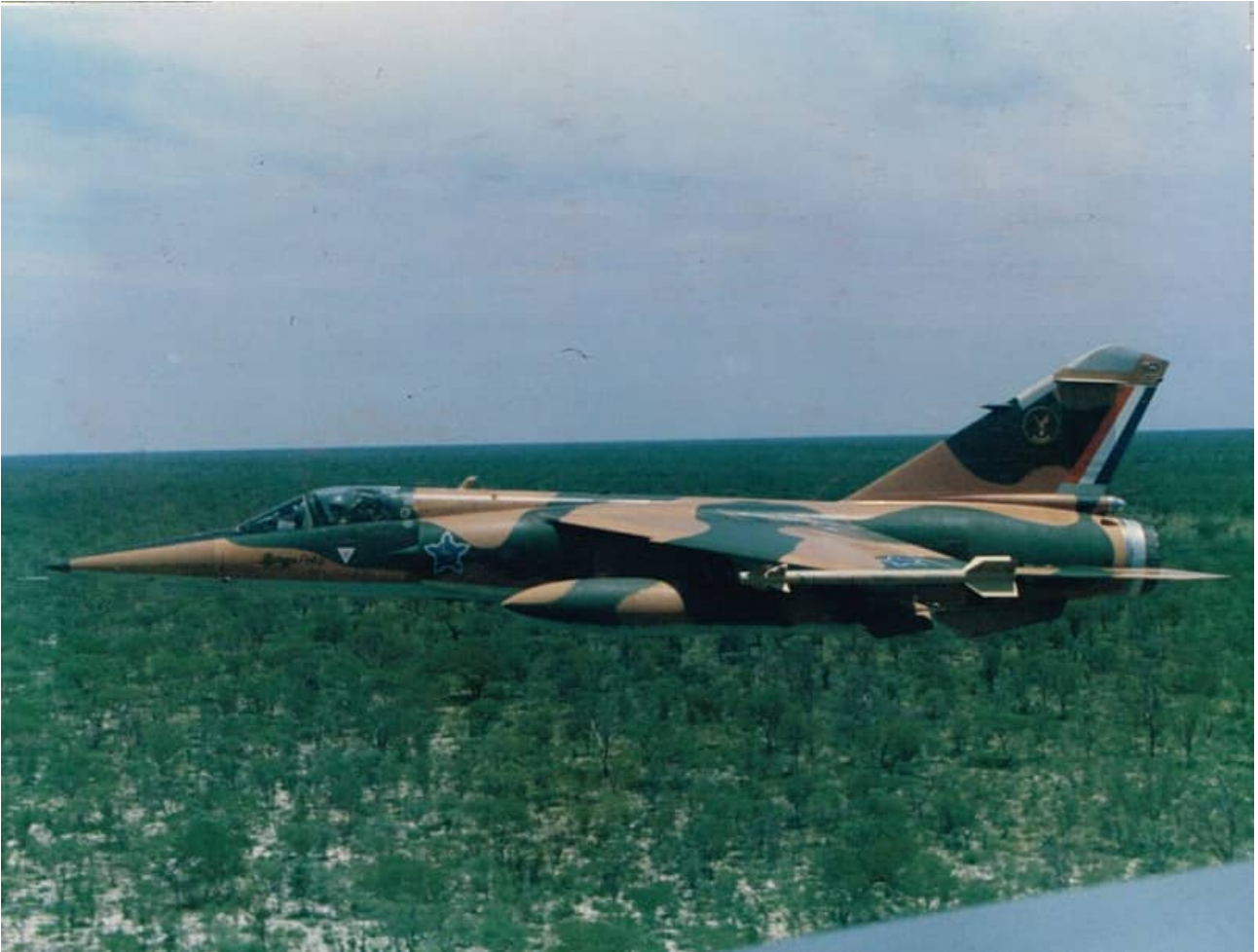
AZ carrying two RP35 external fuel tanks and two V3B missiles.
