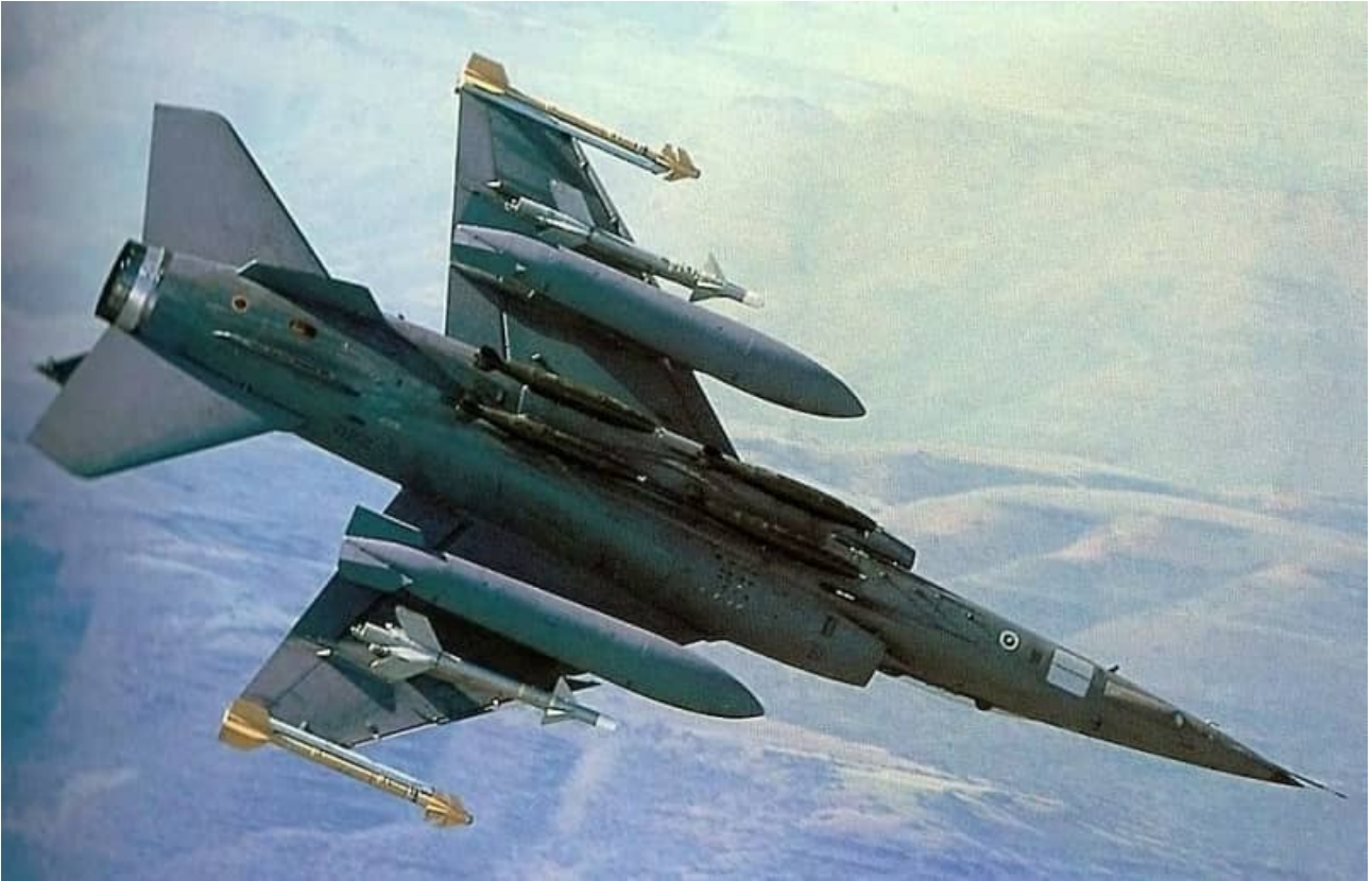
Great image of an AZ showing off a full combat load of four Mk.82 bombs on the centerline bomb carrier, two RP35 external fuel tanks, two V3S Snake IR missiles on outboard wing stations and two V3B IR missiles on the wingtips. Note the RIMS chaff/flare dispensers located integral to the ventral fins.
