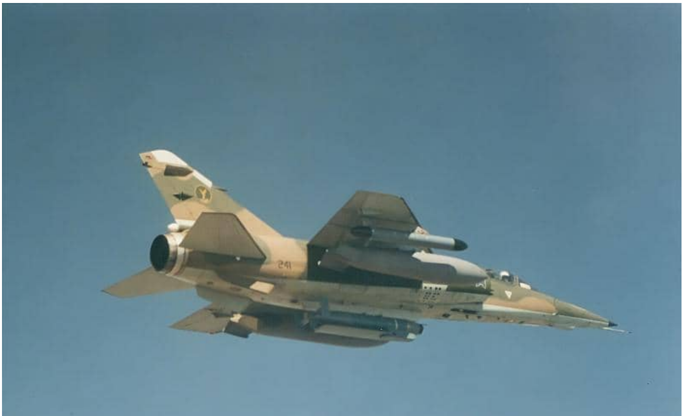
Two images of AZ #241 carrying the H2 bomb and the command pod. It also carries two RP35 external fuel tanks, the starboard one painted in an overall medium grey colour.
