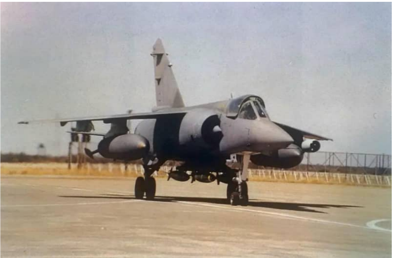
AZ #244 in the three-tone low visibility blue/grey camouflage scheme. #244 carries four Mk. 82 bombs on the centerline CLB4 bomb carrier, two RP35 external fuel tanks and an ACS pod on the port outboard wing pylon. The starboard outboard wing station is empty. Note the downward angle of the rear bombs when carried on the CLB4.
