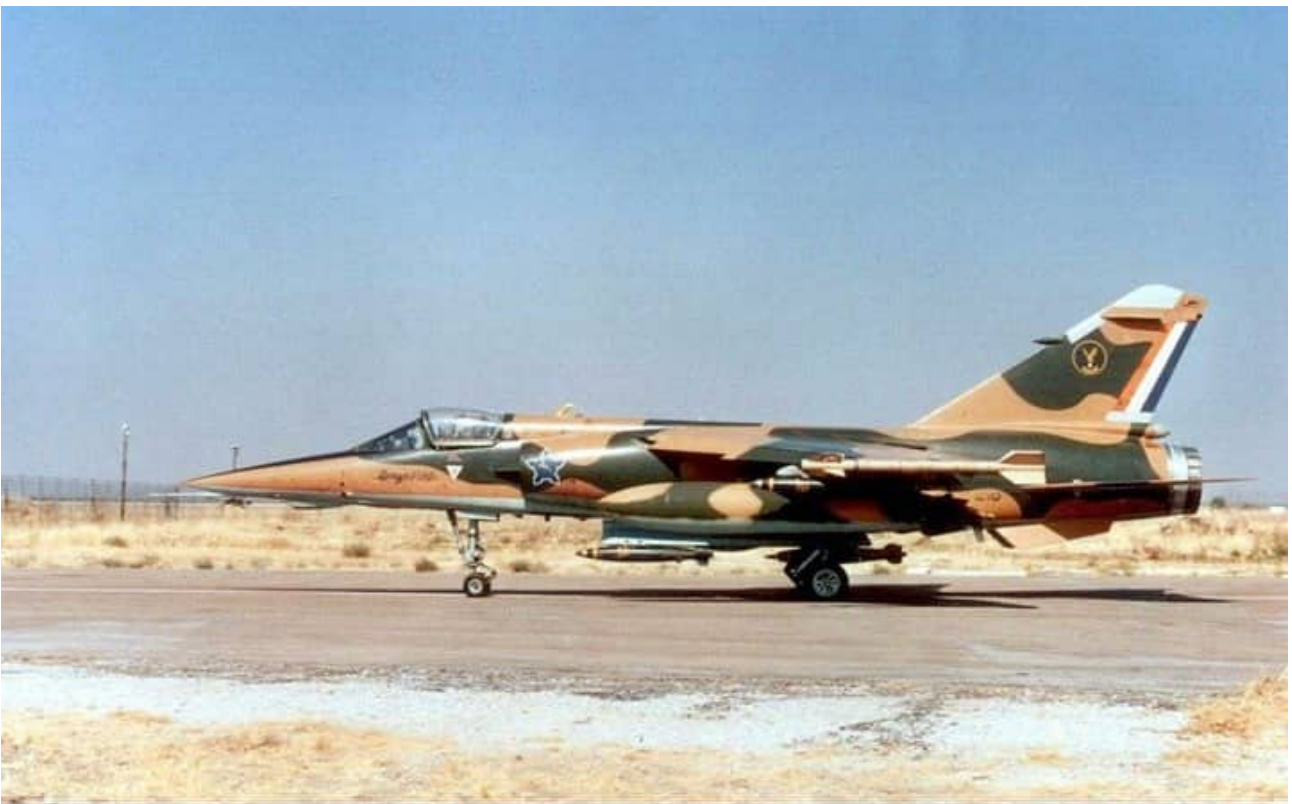
Below: AZ carrying a similar load, but these appear to be smaller Mk. 81 bombs – note the space between the front and rear bombs on the CLB4 bomb carrier compared to the image above. The Mk. 82 was a 250 kg bomb whereas the Mk. 81 was a 125 kg bomb (slimmer in profile and shorter). Note the absence of the black tip of the AZ's nose possibly indicating that the ranging radar is not installed.
