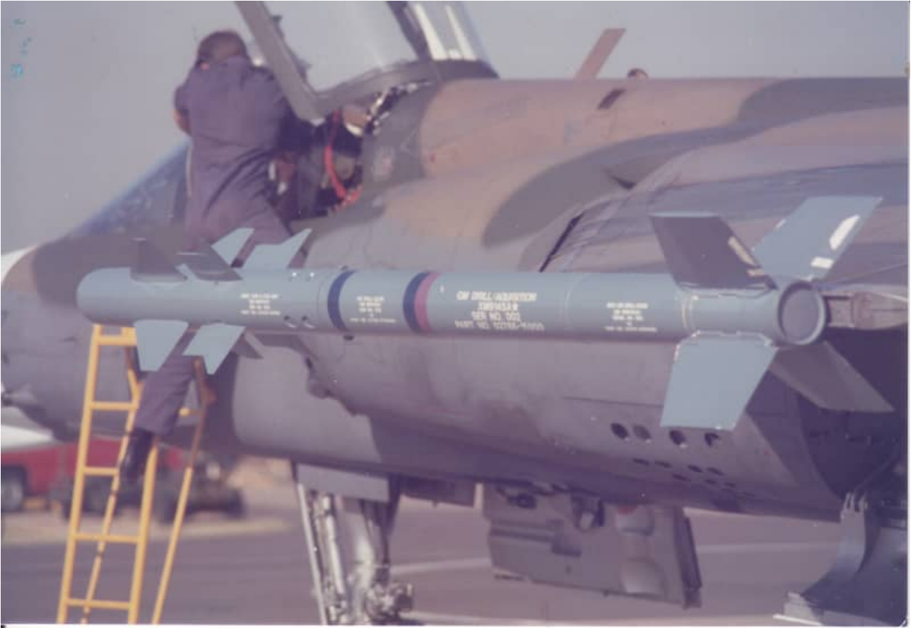
V3C missile on the wingtip launch rail of an AZ. The V3C looks similar to the R550 but has a different seeker head and proximity fuse arrangement – note the circular recesses aft of the canard fins on the missile.
