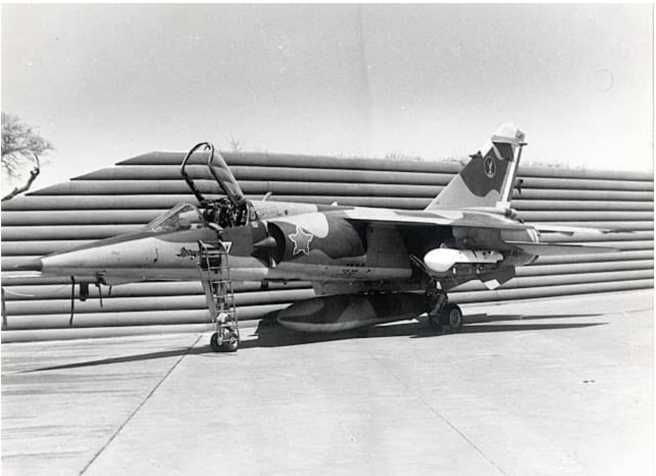
Two images of AZs (#226 above) with RP35 external fuel tank and practice bomb dispensers on the inboard wing stations. Note the fins and endplates at the rear of the RP35. The practice bomb dispenser could carry 4 inert small bombs designed to have the same ballistic properties as a standard Mk.81/82 bomb. The configuration of the inboard and outboard pylons was the same for all external stores carried.
