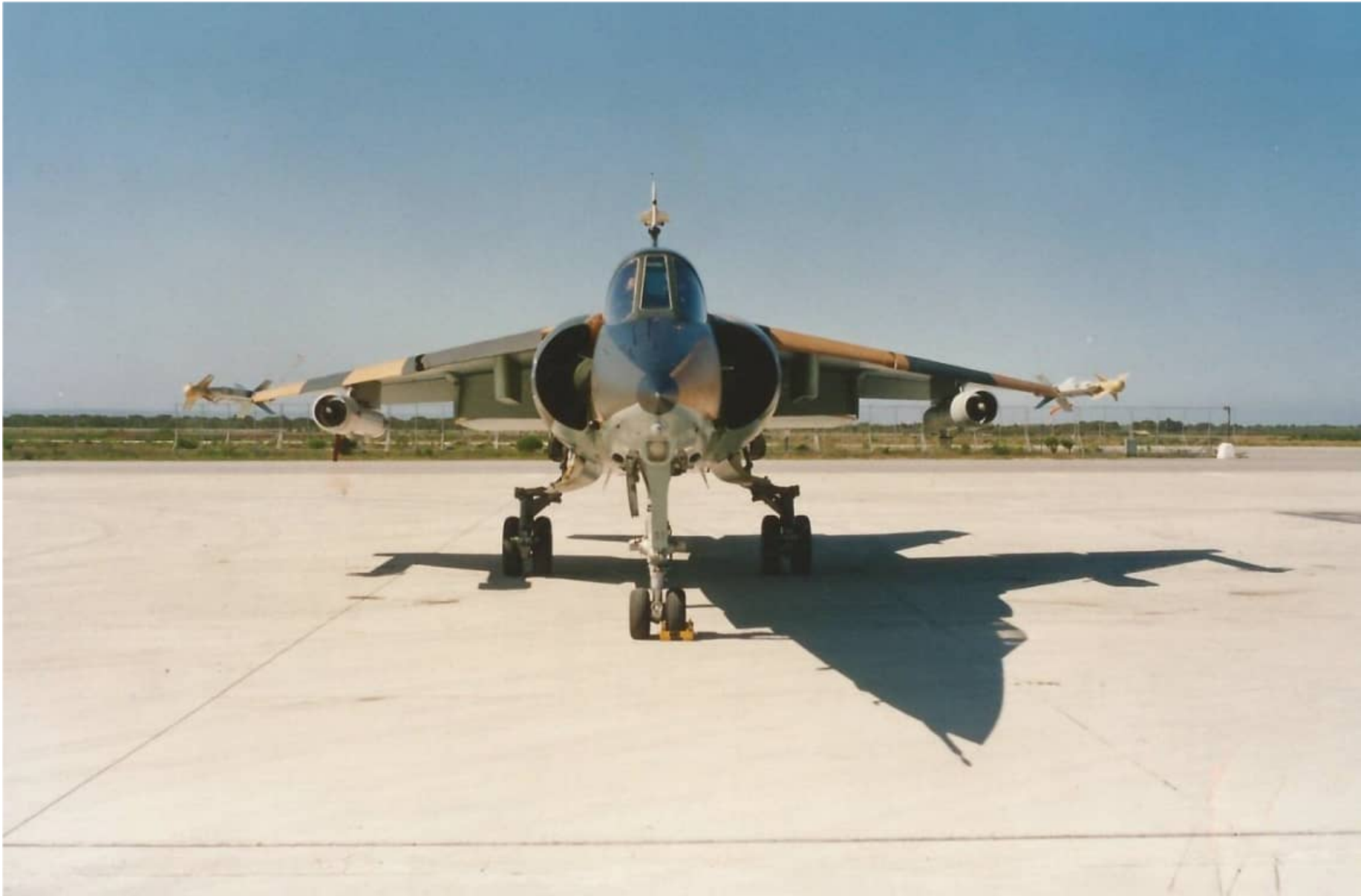
AZ #231 at TFDC Overberg in the southern Cape. It is carrying two ACS pods and two V3B missiles. #231 is also carrying two chaff/flare dispenser pods on the inboard wing station 0 just next to the fuselage. The AZ usually carried only one ACS pod as standard during combat operations in Southern Angola. Equally, the carriage of these particular chaff/flare pods on combat operations was also unlikely.
