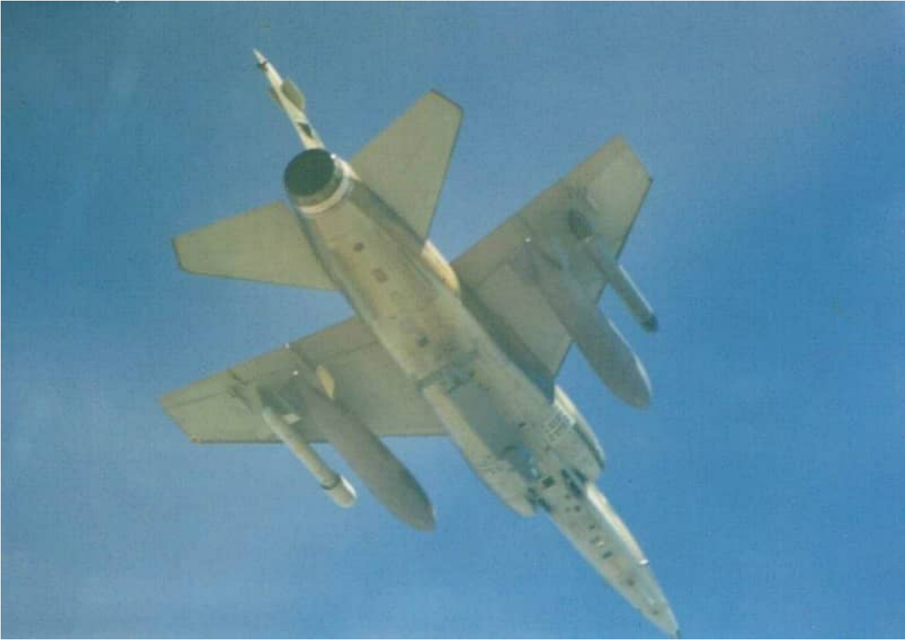
AZ #241 carrying two RP35 fuel tanks, H2 bomb on the fuselage centerline, H2 command pod on starboard wing and ACS pod on port wing.
