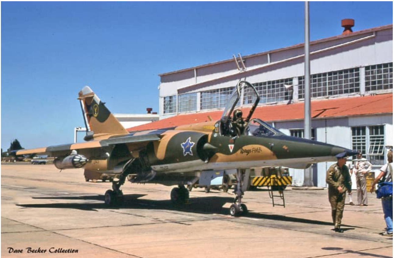
AZ carrying two Matra 155 rocket pods on outboard wing stations.
