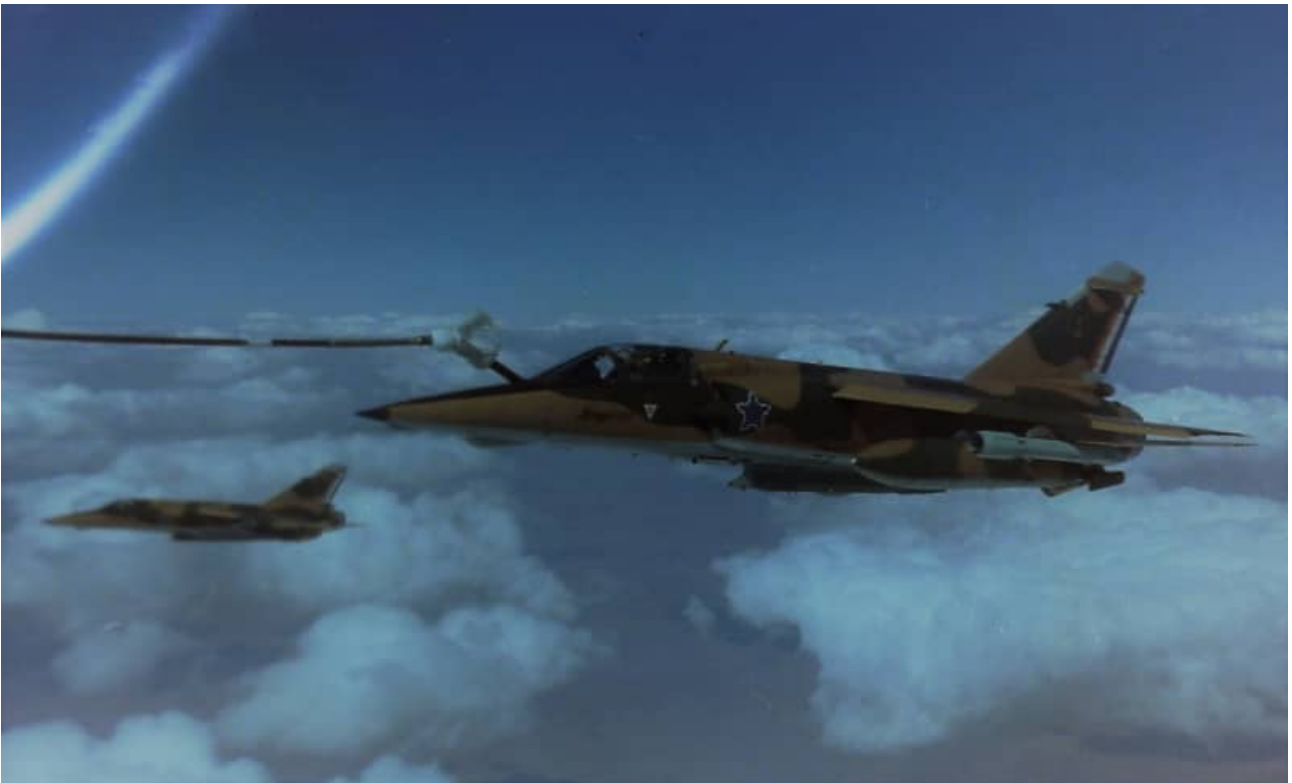
AZ carries an empty CLB4 bomb rack, two RP35 external fuel tanks and an ACS pod on the port outboard wing pylon.
