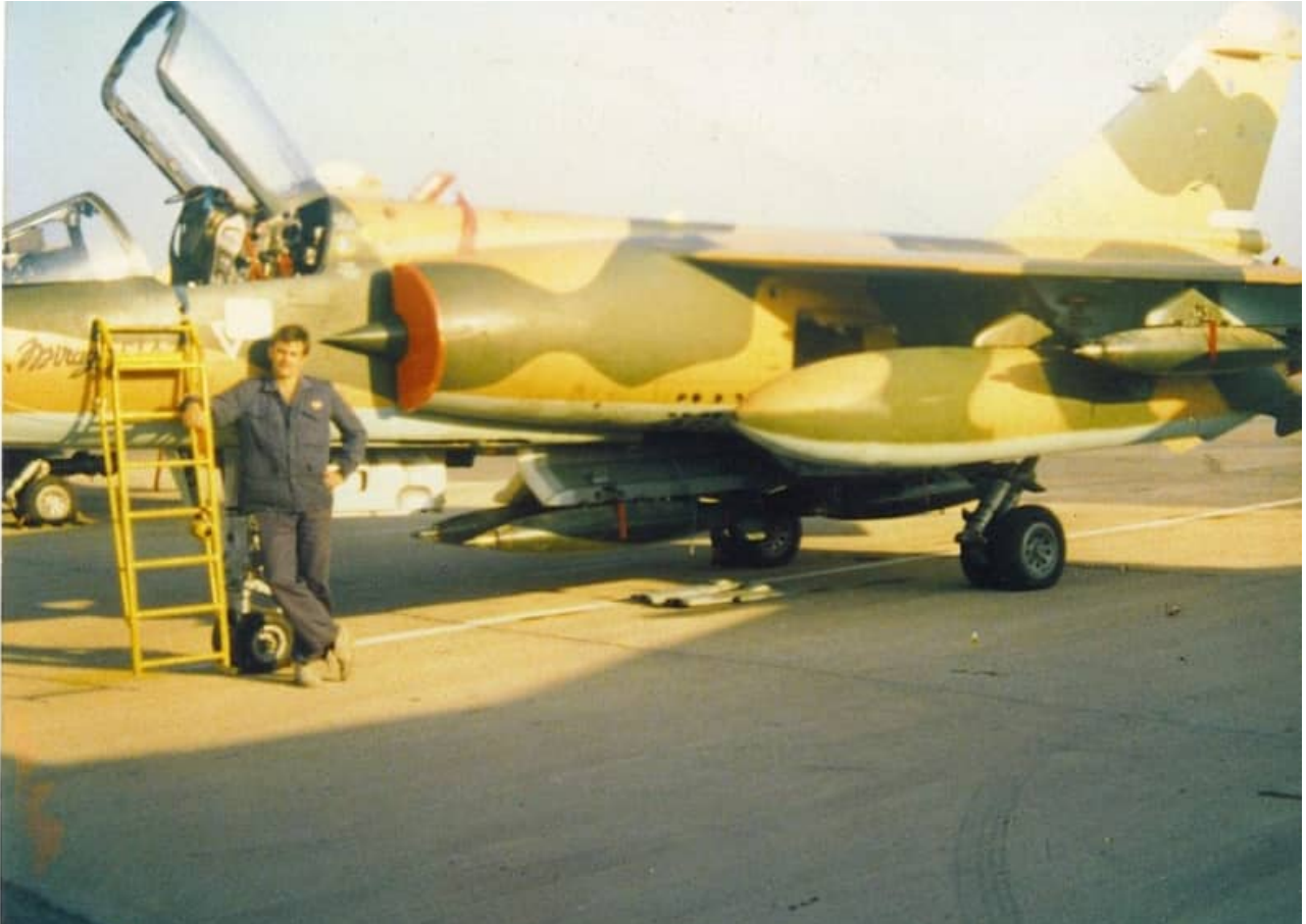
Two images of AZs being fitted with four Mk.82 GP bombs on the centerline CLB4 bomb carrier, RP35 external fuel tanks on the wing inboard station and a Mk. 82 bomb on each of the outboard wing stations. This would be considered a common offensive load on combat operations in Southern Angola. V3B missiles were also carried on the wingtips to provide some form of self-defense if intercepted. The AZ in the image above is devoid of Castles on the intakes, tri-colour rudder and 1 Squadron badge on the vertical stabilizer. In both images, the AZs are painted in the hard-edge buff/dark green camouflage. Note that the tanks are painted in a soft edge camouflage pattern.
