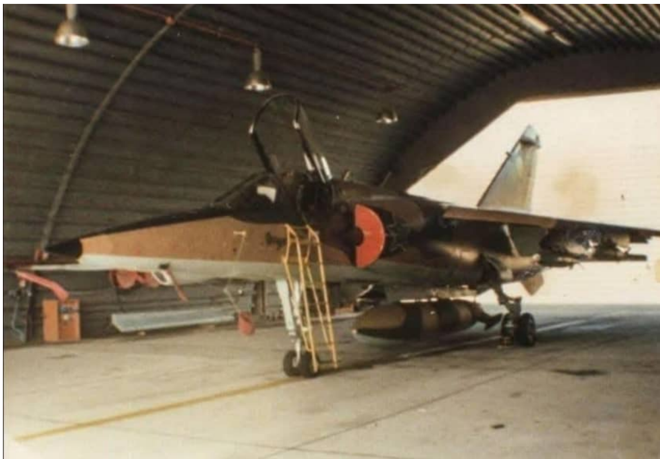
Two images of an AZ in a revetment / hardened aircraft shelter carrying a centerline RP35 fuel tank and what appear to be 4 Mk.81 GP bombs, one each on the wing station.
