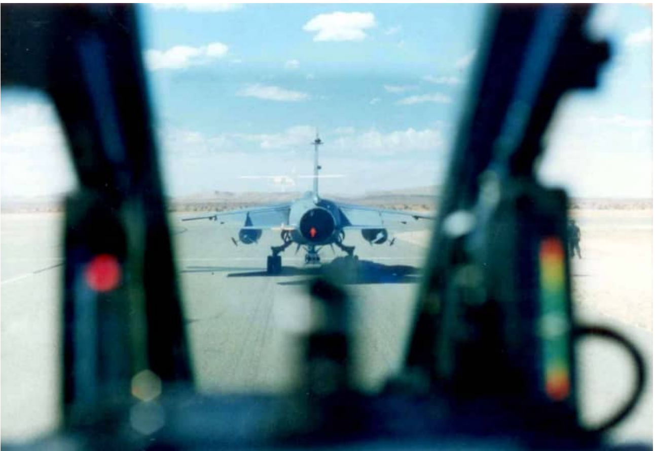
AZ #244 in the 3-colour low visibility camouflage, carrying two RP35 external fuel tanks on the wing inboard stations and a single AS30 on the fuselage centerline station.
