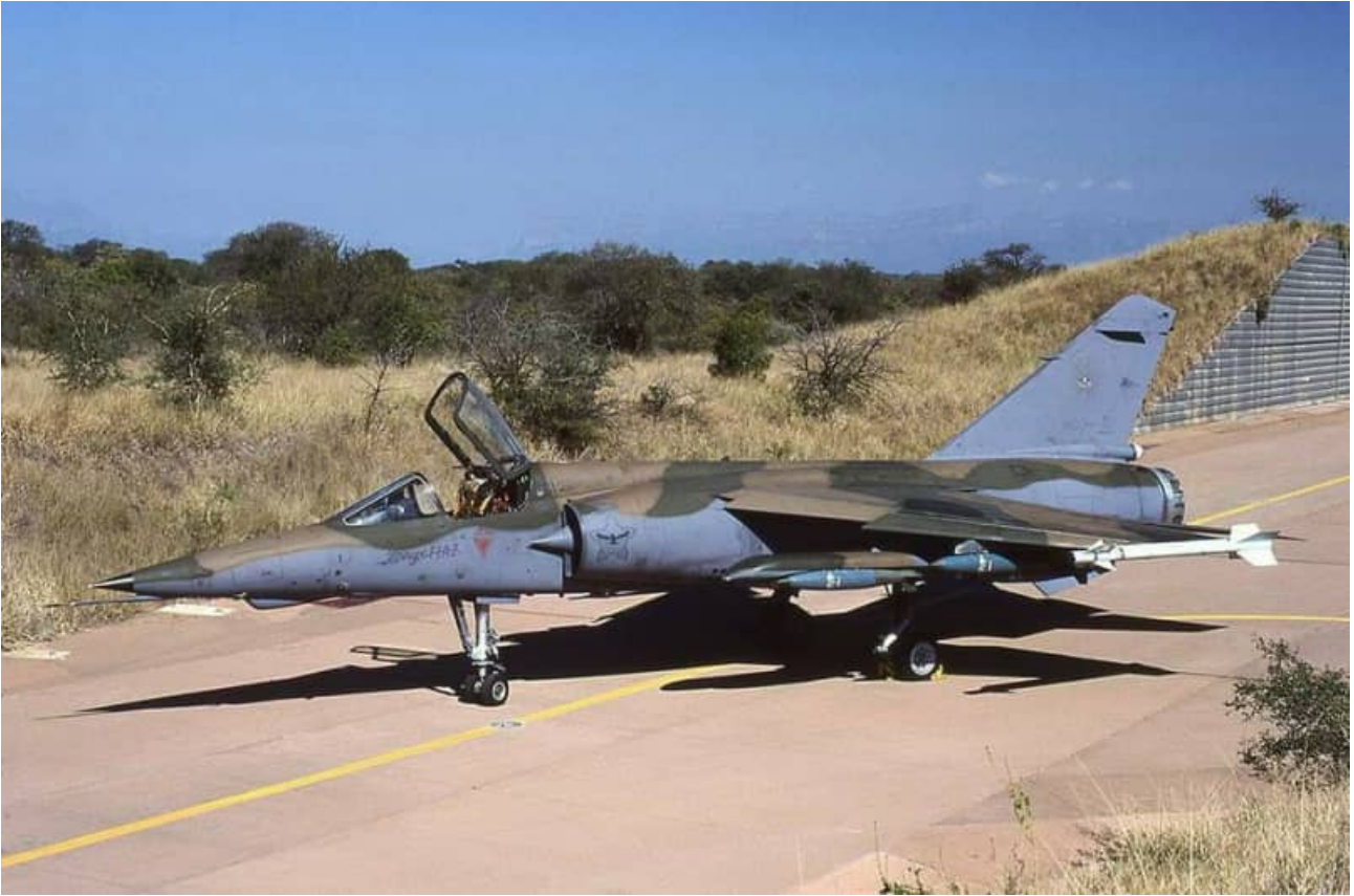
AZ in final camouflage scheme of matt soft edge dark/earth/green/medium blue grey scheme with toned down markings. It is carrying 10 Mk. 81 bombs and V3B missiles.
