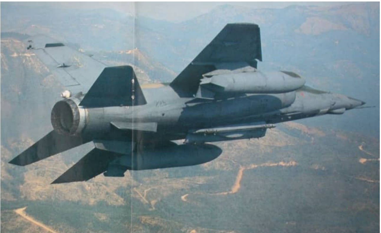
AZ #225 late in its career (final dark earth/green/medium blue grey camouflage) carrying two RP35 fuel tanks and an empty CLB4 4-bomb carrier.
