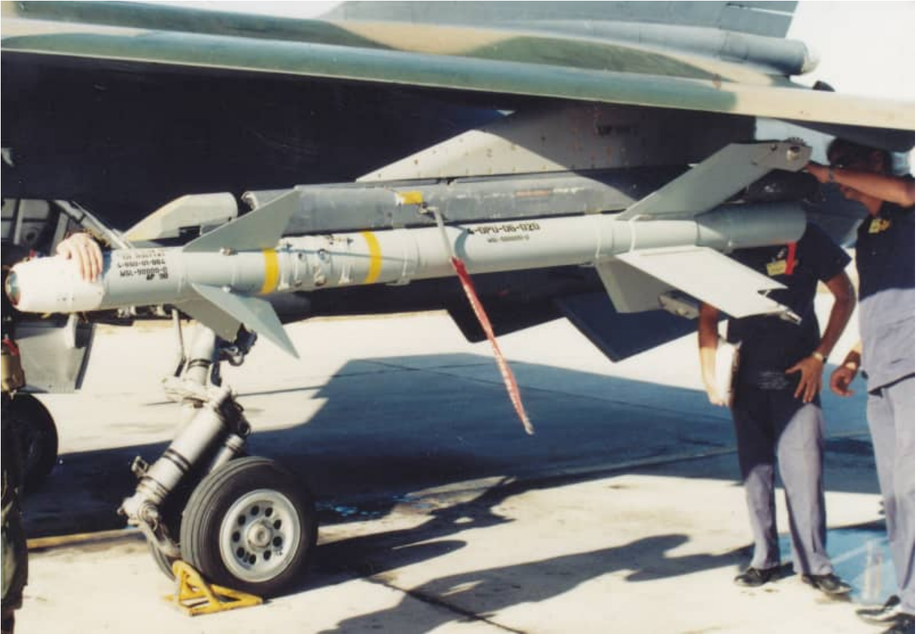
V3S IR missile on an AZ. Note the details of the V3S launcher rail. It is mounted on a pylon specially designed for the V3S in the early 1990s and was unique to the AZ.
