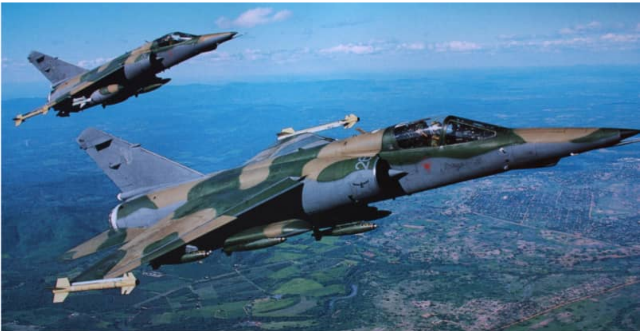
The AZ in the foreground is carrying 14 Mk.81 bombs and two V3B missiles, whereas the second AZ is carrying 4 Mk. 82 bombs on the CLB4 carrier, two RP35 external fuel tanks, two V35 Snake IR missiles on the wing outboard stations and two V3Bs on the wingtips.
