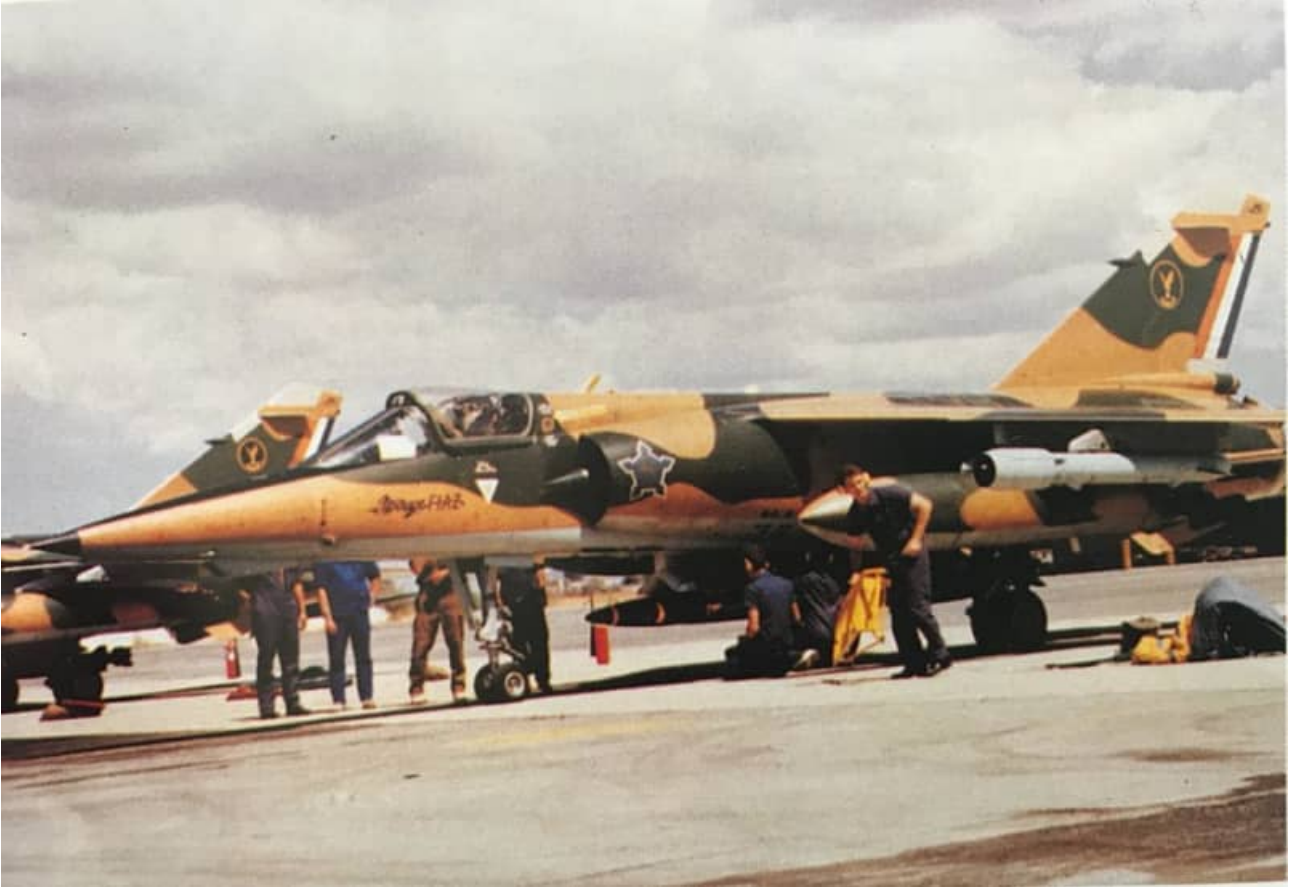
AZ at AFB Grootfontein with an interesting mix of four Mk.82 bombs on the centerline bomb carrier, two RP35 external fuel tanks and an ACS pod on the port outboard wing pylon. The aircraft has the RWS installed but not the RIMS ventral fins.
