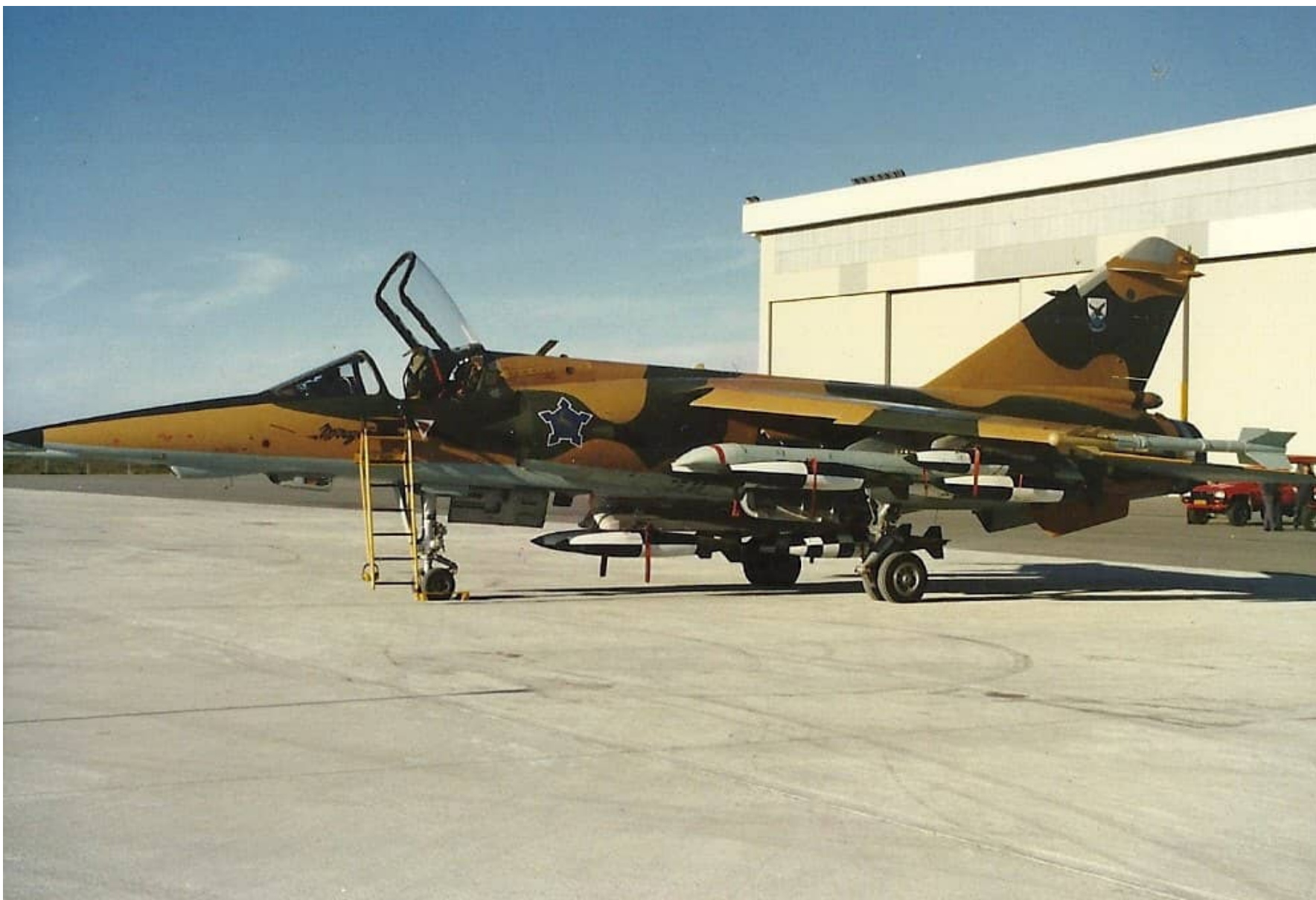
TFDC's AZ #233 is seen carrying 14 x Mk. 82 bombs. The bombs were carried as follows: four on the fuselage CLB4 bomb carrier, four each on the inboard wing stations using the CLB8/A26 bomb carriers and two each on the outboard wing stations (although, on close inspection of the image, the latter appear to be smaller Mk.81s). V3B missiles are also carried on the wingtips. That's 7,000lb or approximately 3 tons of bombs ! AZ would have struggled to get going in this configuration. A more reasonable load would have been 14 x Mk. 81 bombs (3,500lb/1,600kg). This configuration never saw combat operations.
