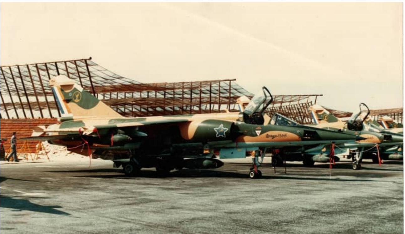
Two great images of AZs being prepared for a bombing sortie at Ondangwa Air Base in northern Namibia. The load out includes four 450kg bombs on the centerline bomb carrier and two 450kg bombs on each outboard wing station. V3B IR missiles are carried on the wingtips. The RP35 1,200 liter external fuel tank was not carried in this configuration and this would've been a short range sortie.
