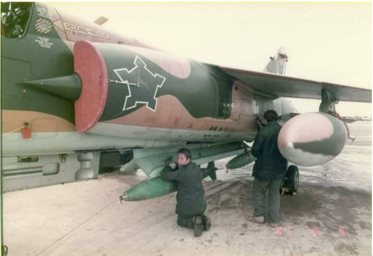
Two images of AZs being fitted with four Mk.82 GP bombs on the centerline CLB4 bomb carrier, RP35 external fuel tanks on the wing inboard station and a Mk. 82 bomb on each of the outboard wing stations. This would be considered a common offensive load on combat operations in Southern Angola. V3B missiles were also carried on the wingtips to provide some form of self-defense if intercepted. The AZ in the image above is devoid of Castles on the intakes, tri-colour rudder and 1 Squadron badge on the vertical stabilizer. In both images, the AZs are painted in the hard-edge buff/dark green camouflage. Note that the tanks are painted in a soft edge camouflage pattern.
