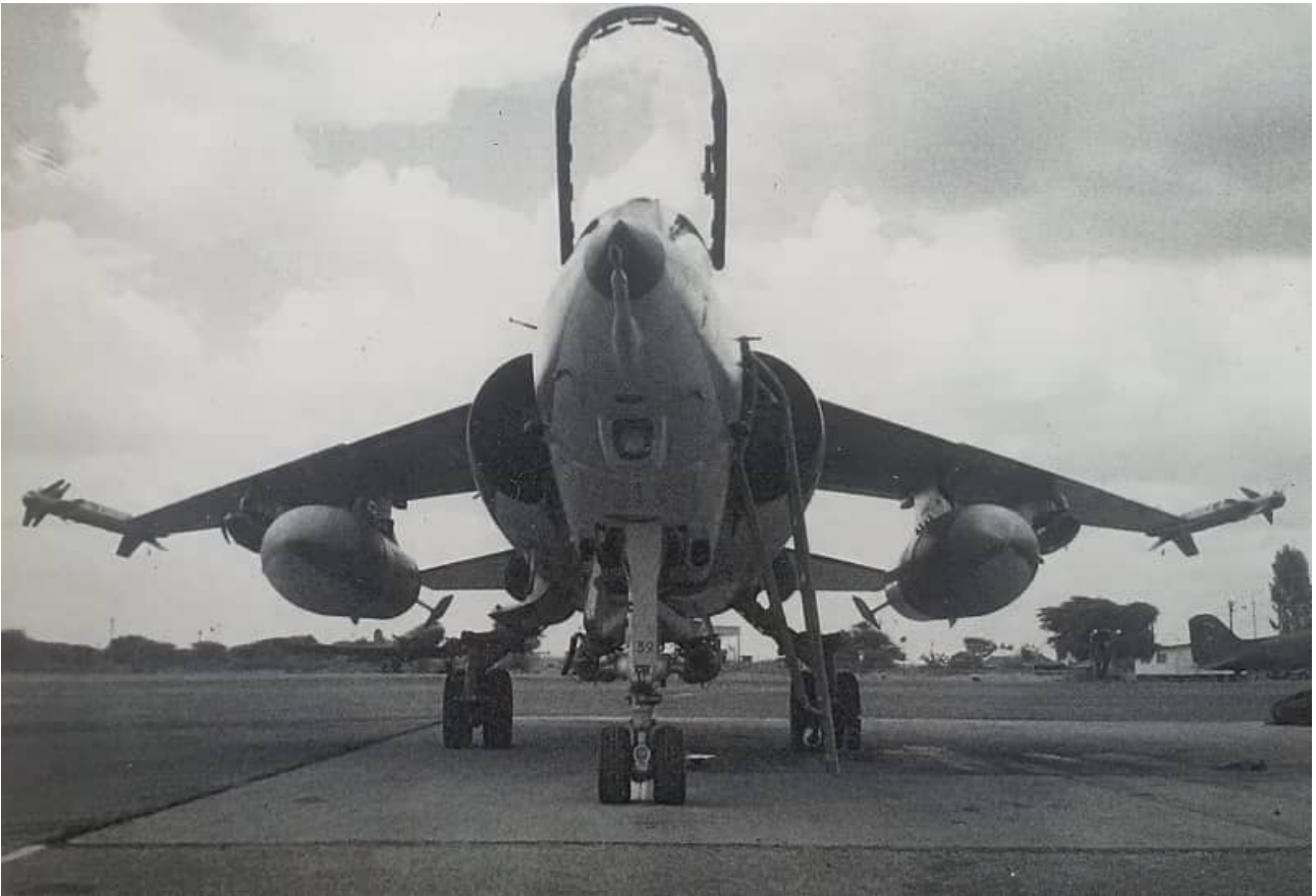
Head on view of an AZ carrying six Mk.82 bombs, two V3B missiles and two RP35 external fuel tanks.
