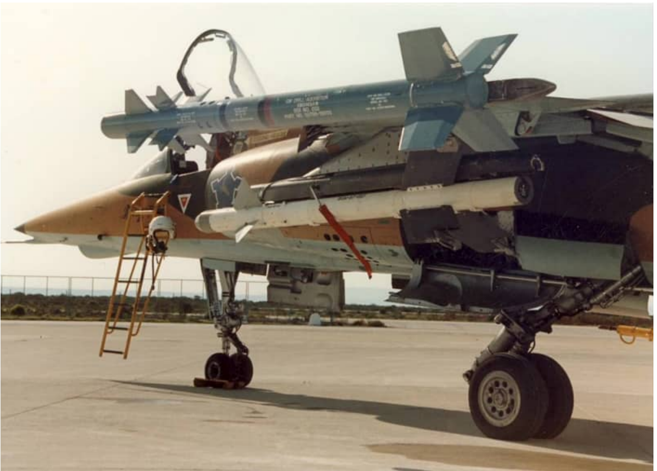
AZ at TFDC with a V3C IR missile on the wingtip launcher and a V3S Snake IR missile on the outboard wing station.
