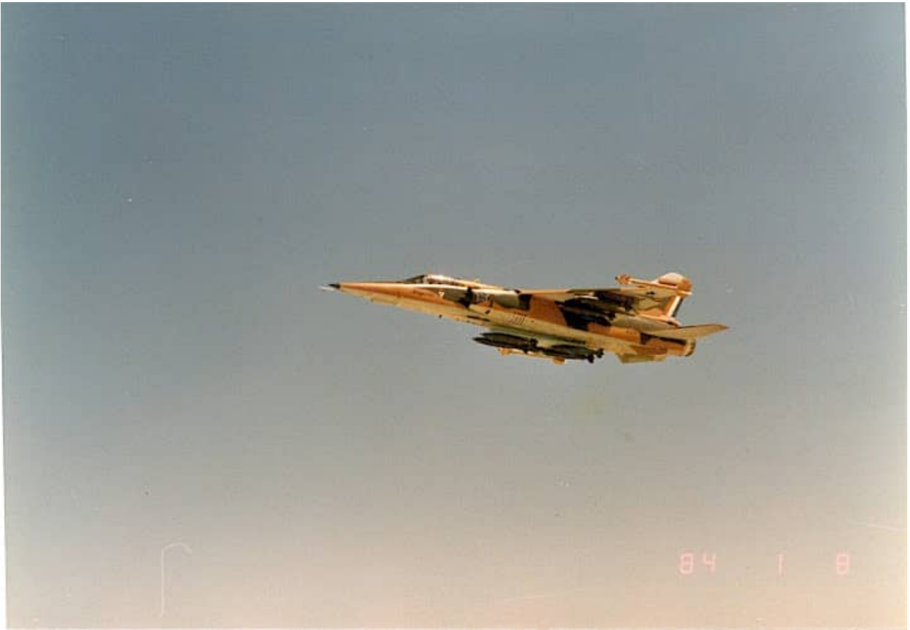
Two images of AZs on combat operations carrying eight Mk.82 bombs, four on the CLB4 bomb carrier and one on each of the wing pylons, and two V3B missiles. This would represent a relatively short range close air support mission as no external fuel tanks are carried.
