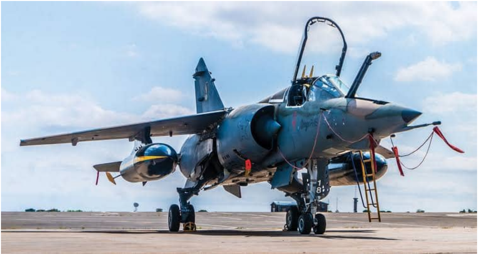
AZ #218 carrying two composite (non-metallic) 1,200 liter external fuel tanks developed by CSIR. These were not productionized.
