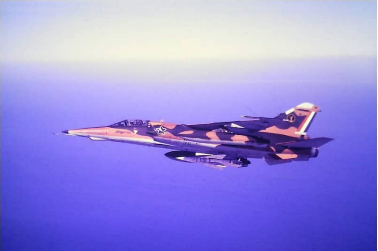
AZ carrying two RP35 external fuel tanks on the wing inboard stations and a single AS30 on the fuselage centerline station.
