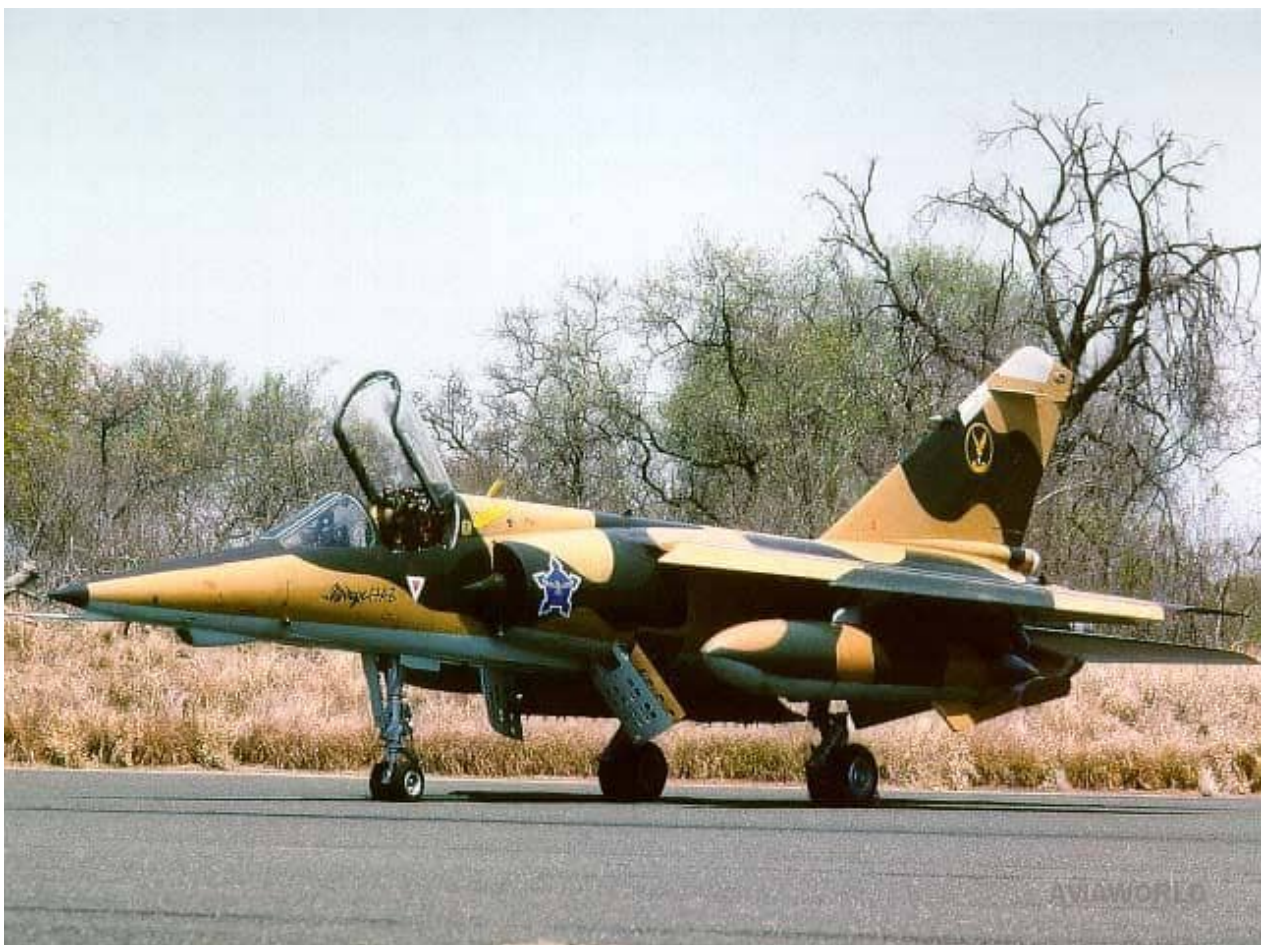
AZ with two RP35 1,200 liter external fuel tanks located on the inboard pylons. The RP35 is camouflaged to match the aircraft.
