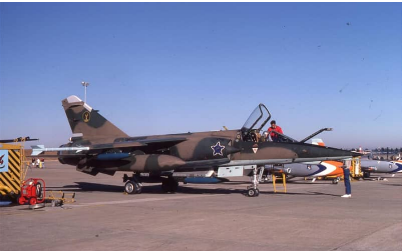
The AZ in the image above is carrying six Mk.82 bombs, two RP35 external fuel tanks and two V3B missiles. The AZ is painted in the interim colour scheme of matt soft-edge dark earth/green upper surfaces with pale blue lower surfaces and full high visibility markings (with the exception of the tri-colour rudder). The fuel tank is painted in a wraparound dark earth/green soft edge pattern. Note the hard-edge demarcation between the upper and lower surface colours.
