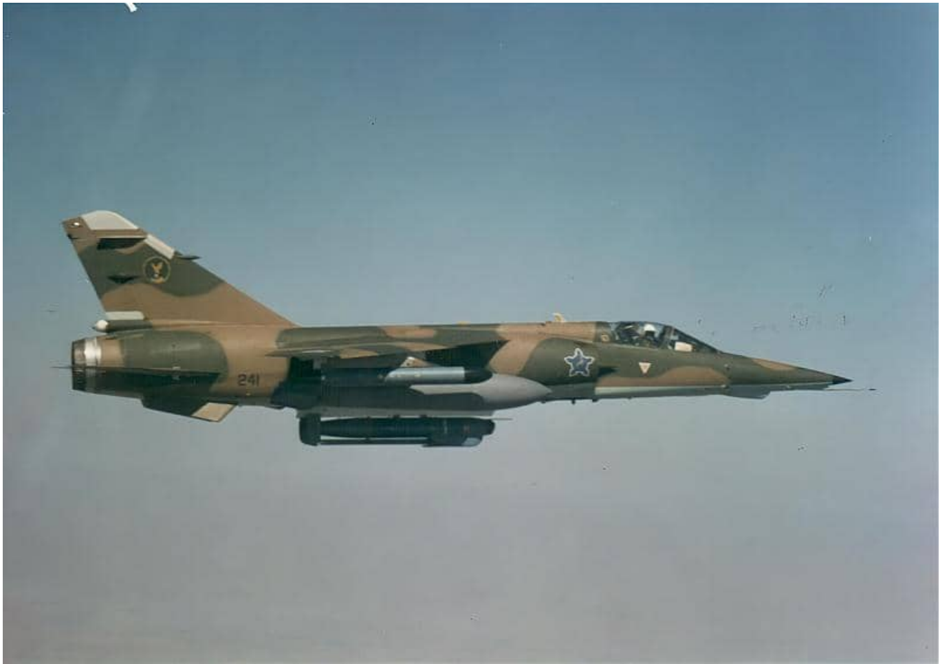
Two images of AZ #241 carrying the H2 bomb and the command pod. It also carries two RP35 external fuel tanks, the starboard one painted in an overall medium grey colour.
