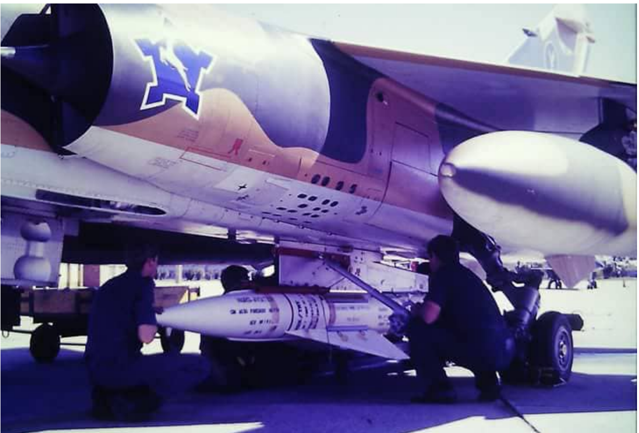
Two images of an AZ carrying an AS30 missile and two RP35 external fuel tanks. Note that, although the AZ is painted in the hard-edge buff/dark green camouflage scheme, the tanks have soft edges between the camouflage colours. The configuration of the centerline pylon for the AS30 is very different to that used to carry the RP35 external fuel tank.
