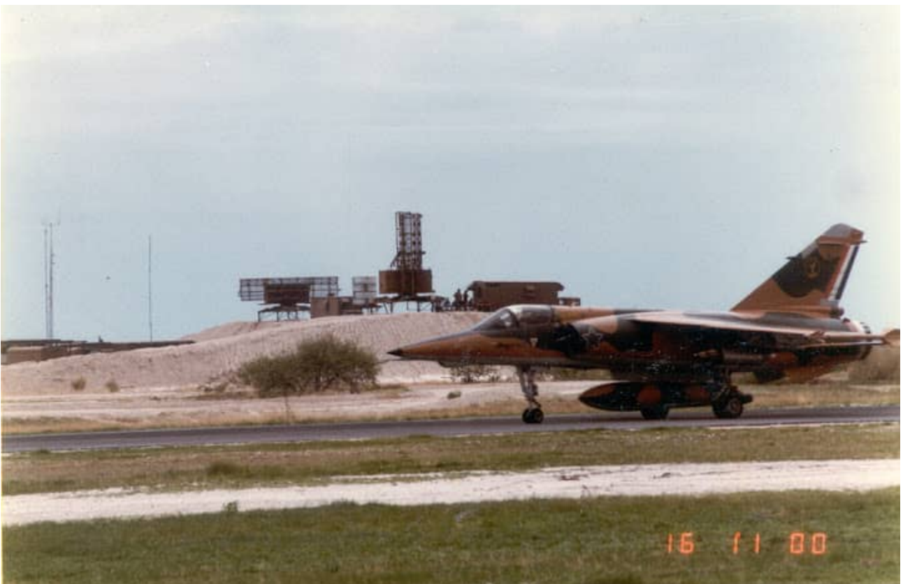
AZ in the operational area during the Border War, most likely Ondangwa Air Base. It is loaded with a centerline RP35 fuel tank, two Matra 155 rocket pods and two V3B missiles.
