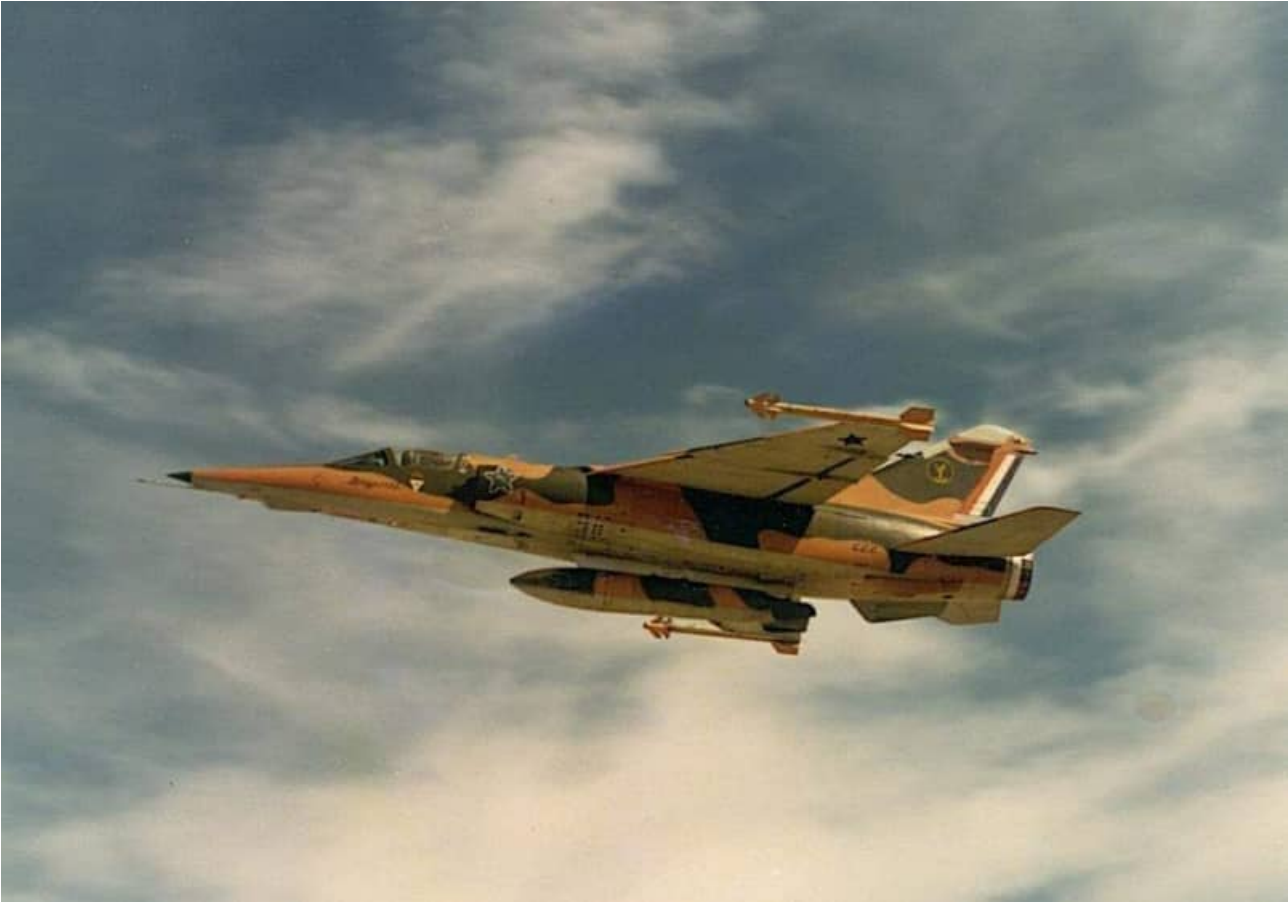
Images of AZ #222 above and AZ #230 below carrying a single RP35 fuel tank and two V3B missiles on the wingtips. This would be a typical air defence load, more the domain of the CZ. #222 is in the original buff/dark green/pale blue camouflage whereas #230 is in the final dark earth/green/medium blue-grey camouflage
