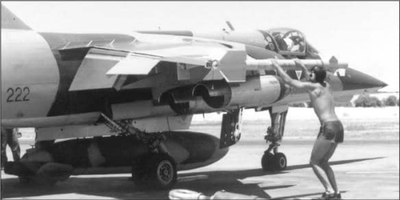
AZ #222 in hard edge buff/dark green camouflage. Note that the fuel tank has a feathered edge between the camouflage colours. The Matra 155 rocket pods were unpainted and were in various metallic colours. The frangible covers were an off yellow colour. Note the asymmetric canard fin arrangement on the wingtip V3B missile.
