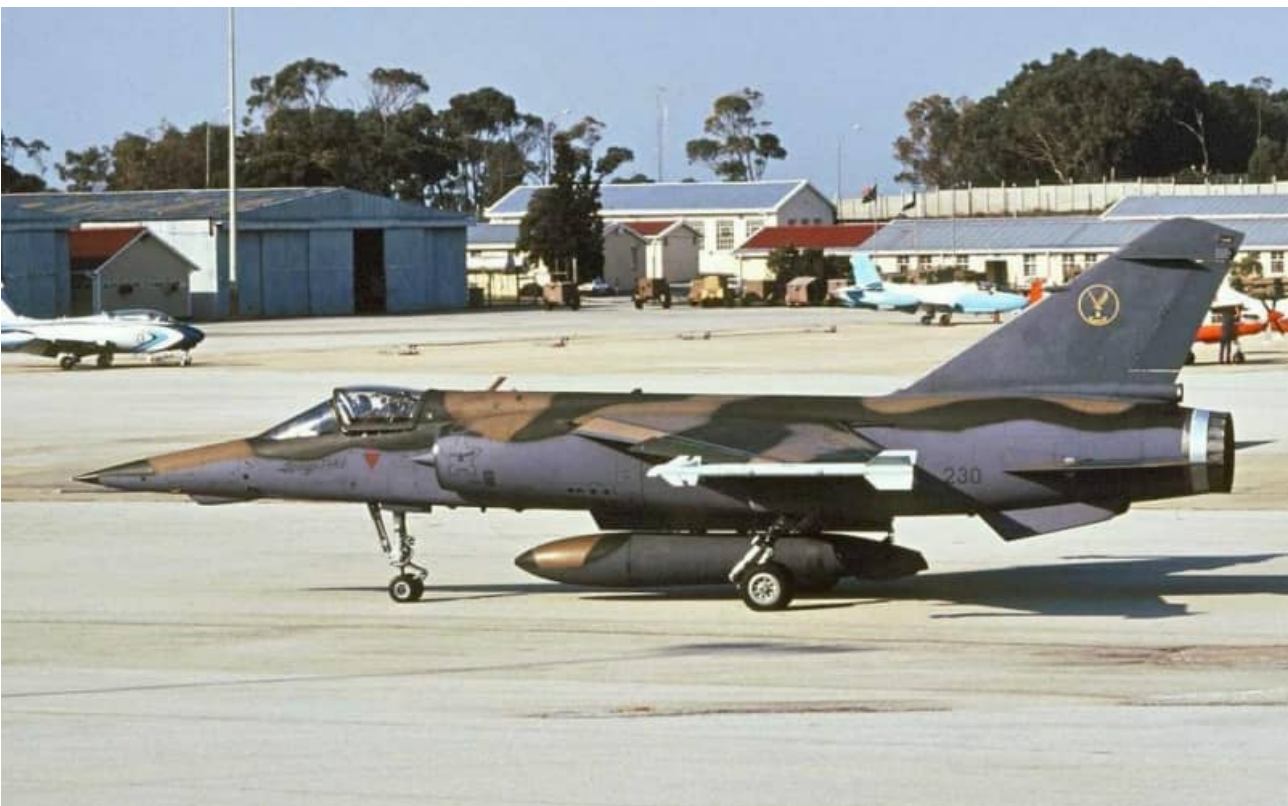
Images of AZ #222 above and AZ #230 below carrying a single RP35 fuel tank and two V3B missiles on the wingtips. This would be a typical air defence load, more the domain of the CZ. #222 is in the original buff/dark green/pale blue camouflage whereas #230 is in the final dark earth/green/medium blue-grey camouflage
