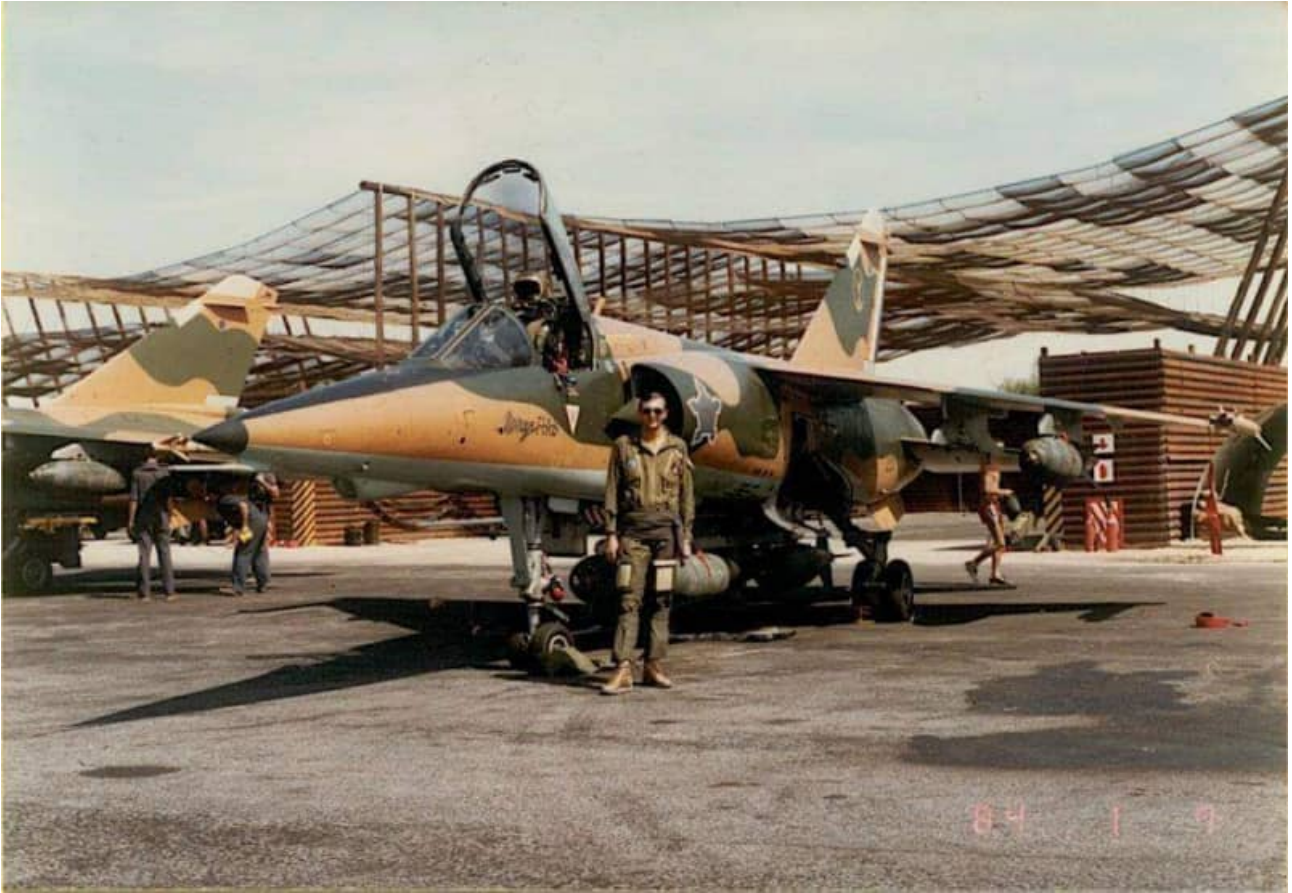
Two great images of AZs being prepared for a bombing sortie at Ondangwa Air Base in northern Namibia. The load out includes four 450kg bombs on the centerline bomb carrier and two 450kg bombs on each outboard wing station. V3B IR missiles are carried on the wingtips. The RP35 1,200 liter external fuel tank was not carried in this configuration and this would've been a short range sortie.
