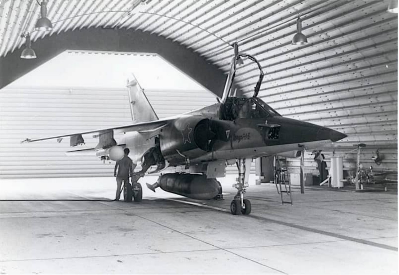
Two images of AZs (#226 above) with RP35 external fuel tank and practice bomb dispensers on the inboard wing stations. Note the fins and endplates at the rear of the RP35. The practice bomb dispenser could carry 4 inert small bombs designed to have the same ballistic properties as a standard Mk.81/82 bomb. The configuration of the inboard and outboard pylons was the same for all external stores carried.
