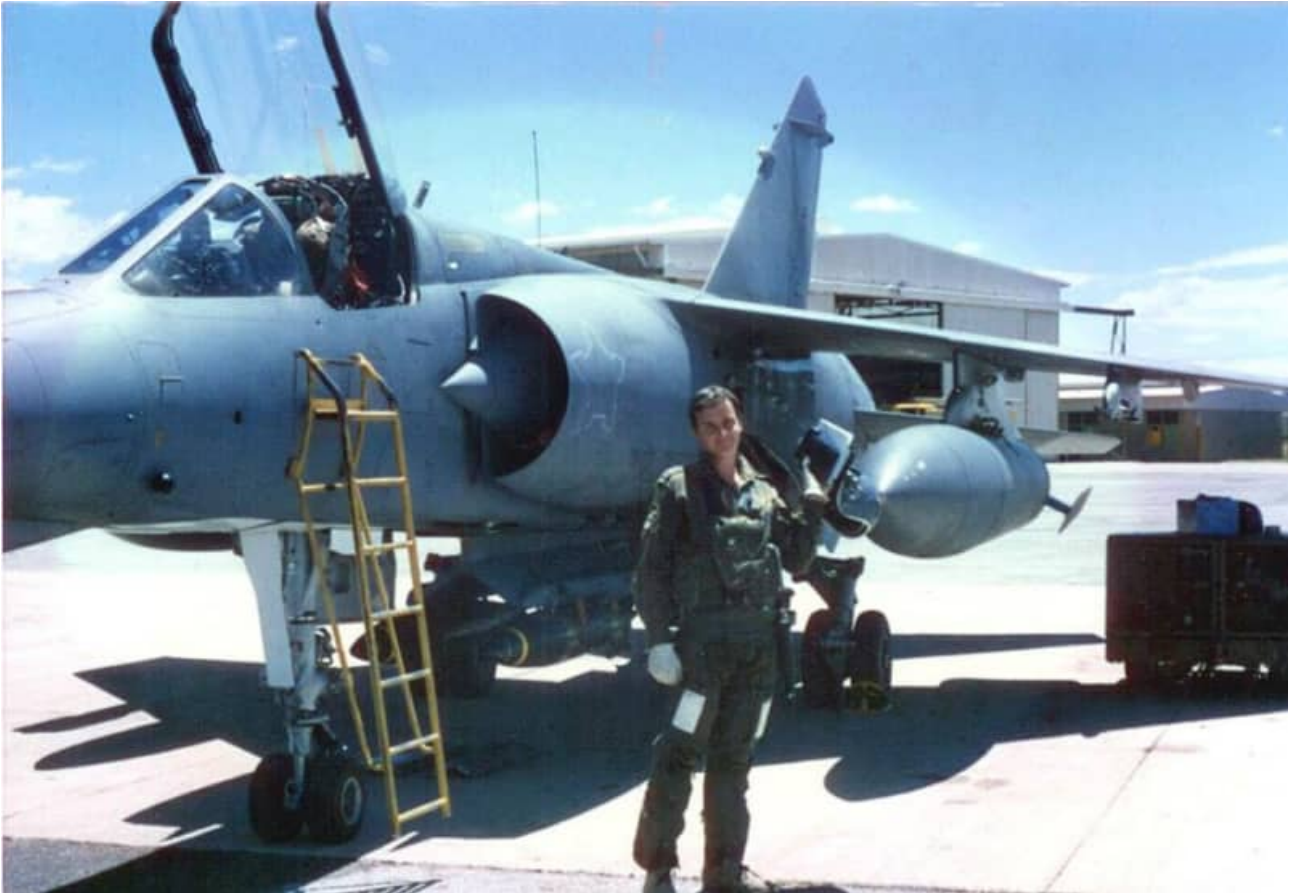
AZ with two RP35 external fuel tanks and CLB4 pylon carrying Mk.81 bombs. The tanks have been painted blue-grey.
