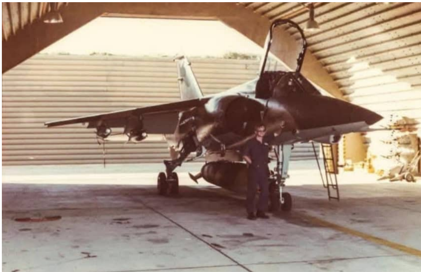
Two images of an AZ in a revetment / hardened aircraft shelter carrying a centerline RP35 fuel tank and what appear to be 4 Mk.81 GP bombs, one each on the wing station.
