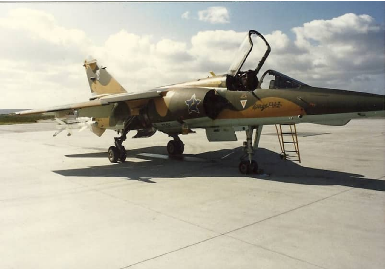
TFDC's AZ #233 carrying a V3S Snake IR missile on the starboard outboard wing station.
