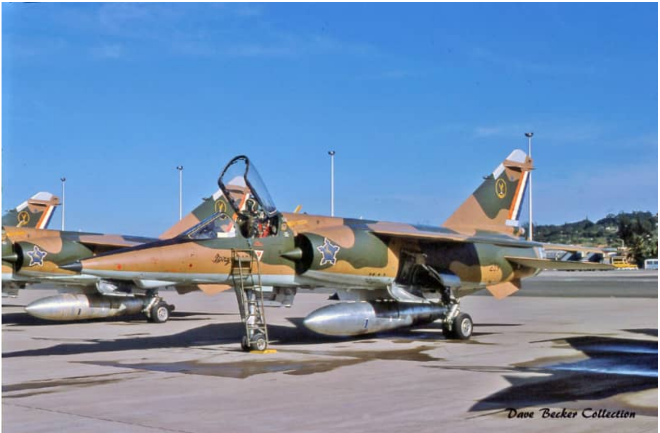
CZ #239 with a single RP35 1,200 liter external fuel tank on the fuselage centerline station. The RP35 is unpainted. The stabilizer fin can be seen at the rear of the RP35 on the AZ in the background. The RP35 was the standard external fuel tank used throughout the AZ's service with the SAAF.
