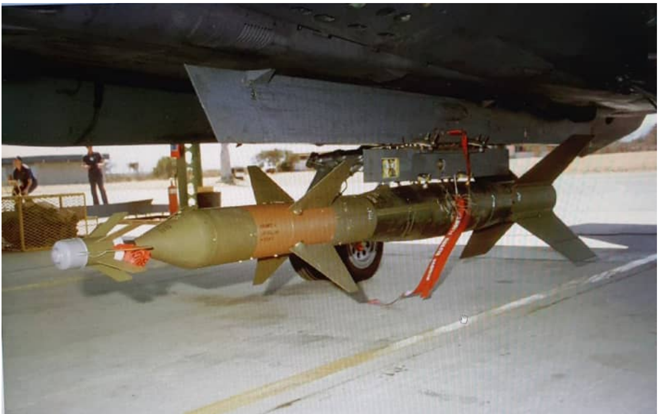
Another view of an AZ with a Griffin Laser Guided Bomb (LGB) on the centerline station. Note the adaptor between the pylon and the bomb.
