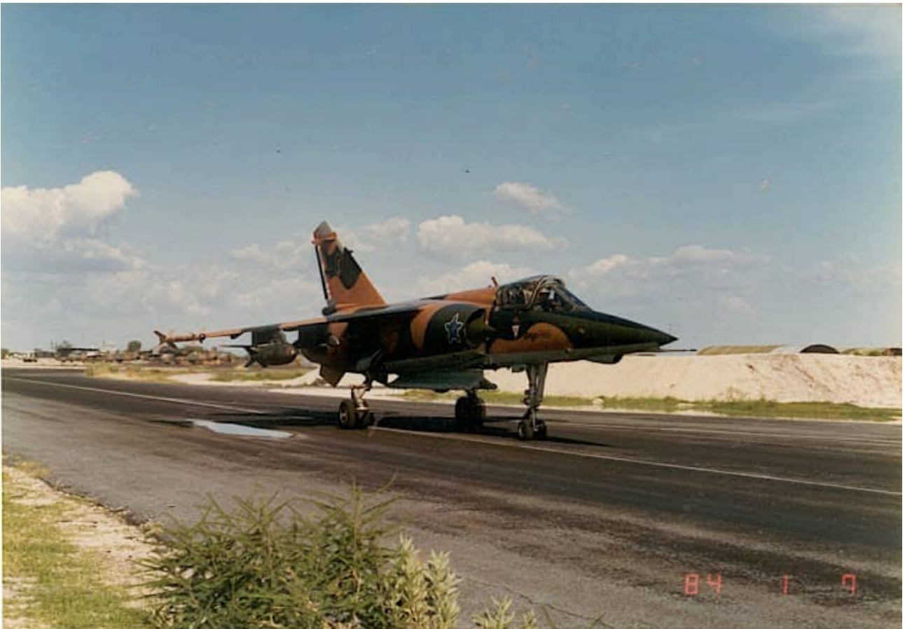
AZ in the Operational Area of Northern Namibia (Ondangwa) carrying an empty CLB4 bomb carrier on the centerline and a 450kg GP bomb on the starboard outboard wing pylon. It also carries V3B missiles on the starboard wingtip.
