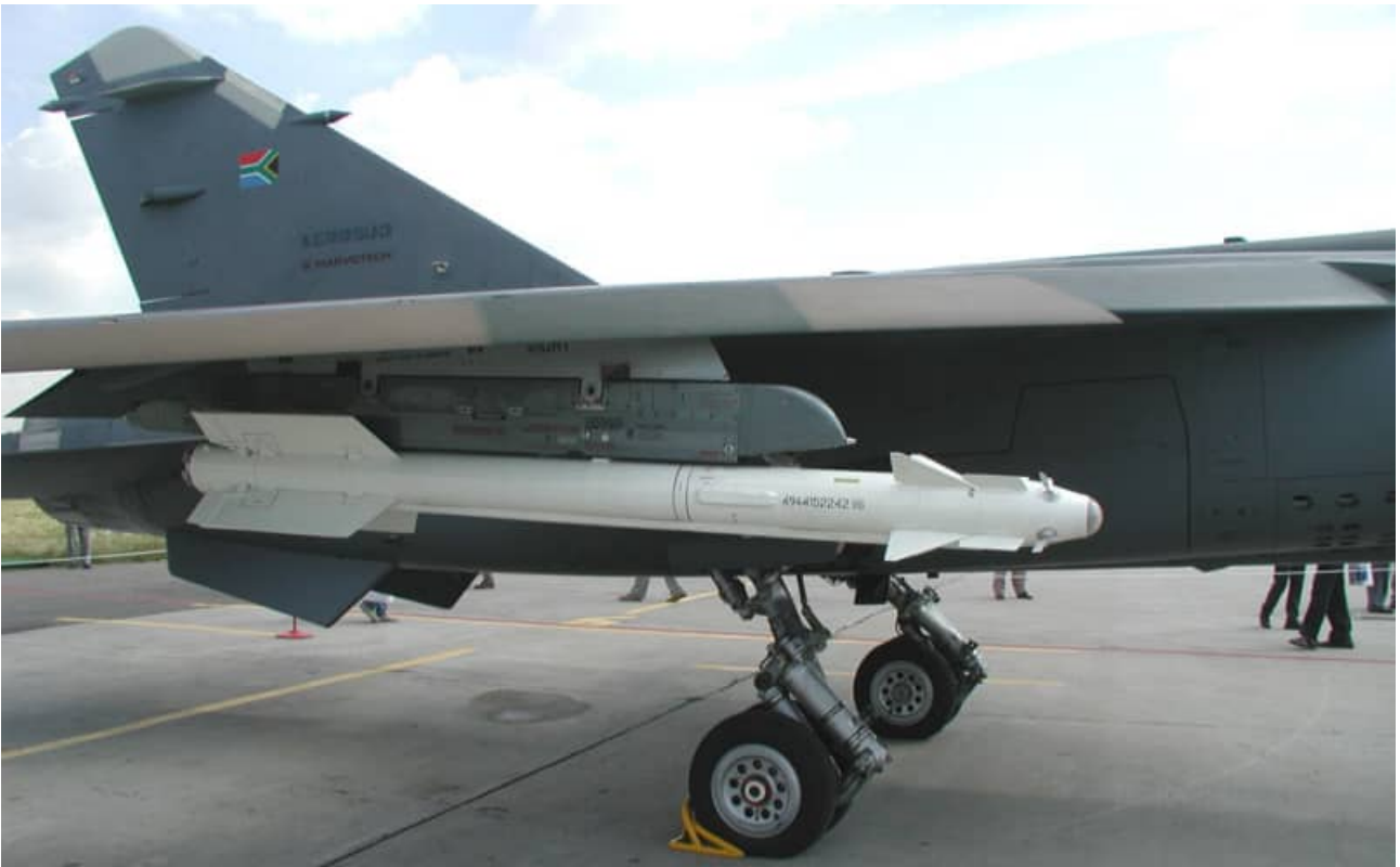
AZ #216 is pictured here with the Russian R-73 (AA-11 Archer) air to air missile installed on the outboard wing pylon. #216 was also fitted with a Russian SMR-95 engine in place of the Atar 09K50 and was dubbed "Super Mirage F1". Neither were taken into operation by the SAAF.
