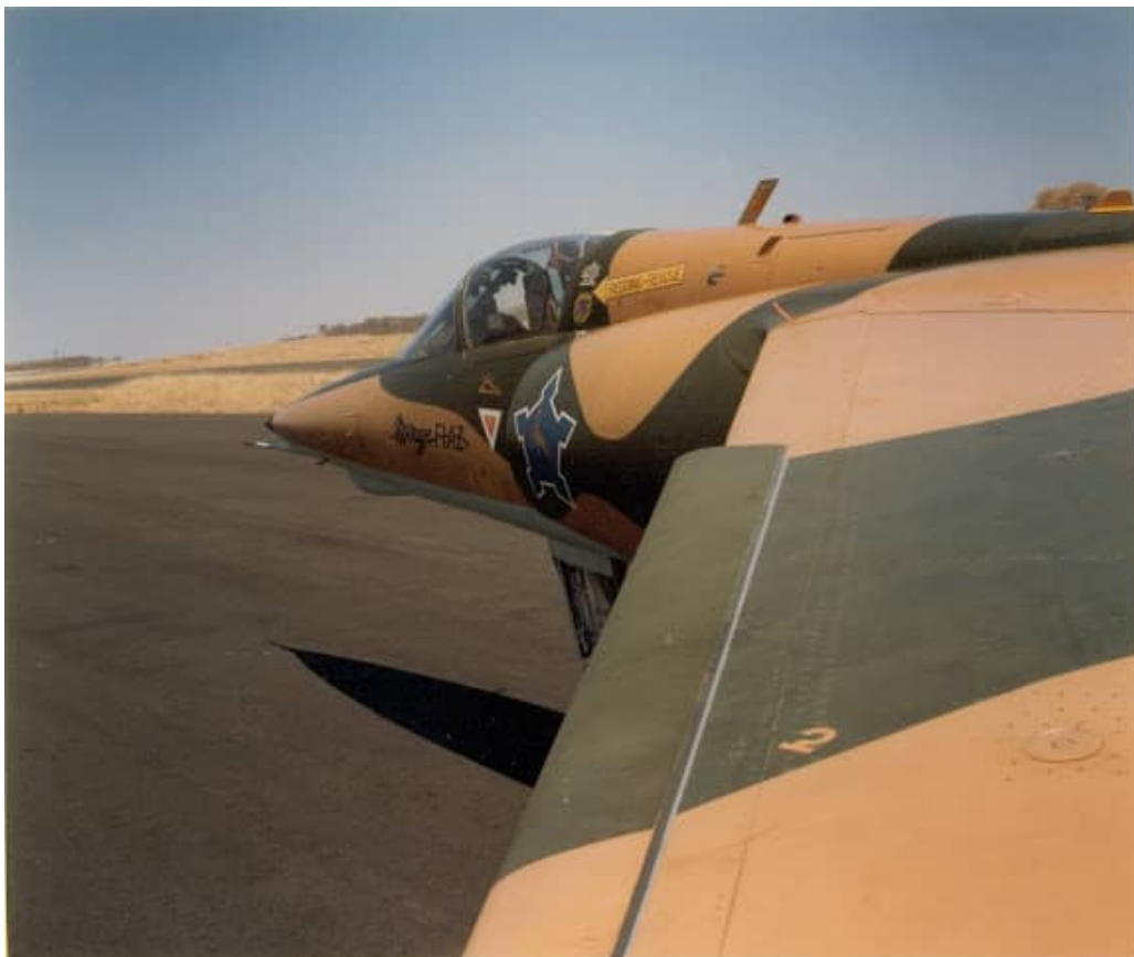
Two images of AZ #223. Note the faded appearance of the buff/dark green camouflage. The yellow marking on the wing in the image below is the standard NATO symbol for lifting point. This appears to be pattern 1 – green inboard section of leading-edge slat.
