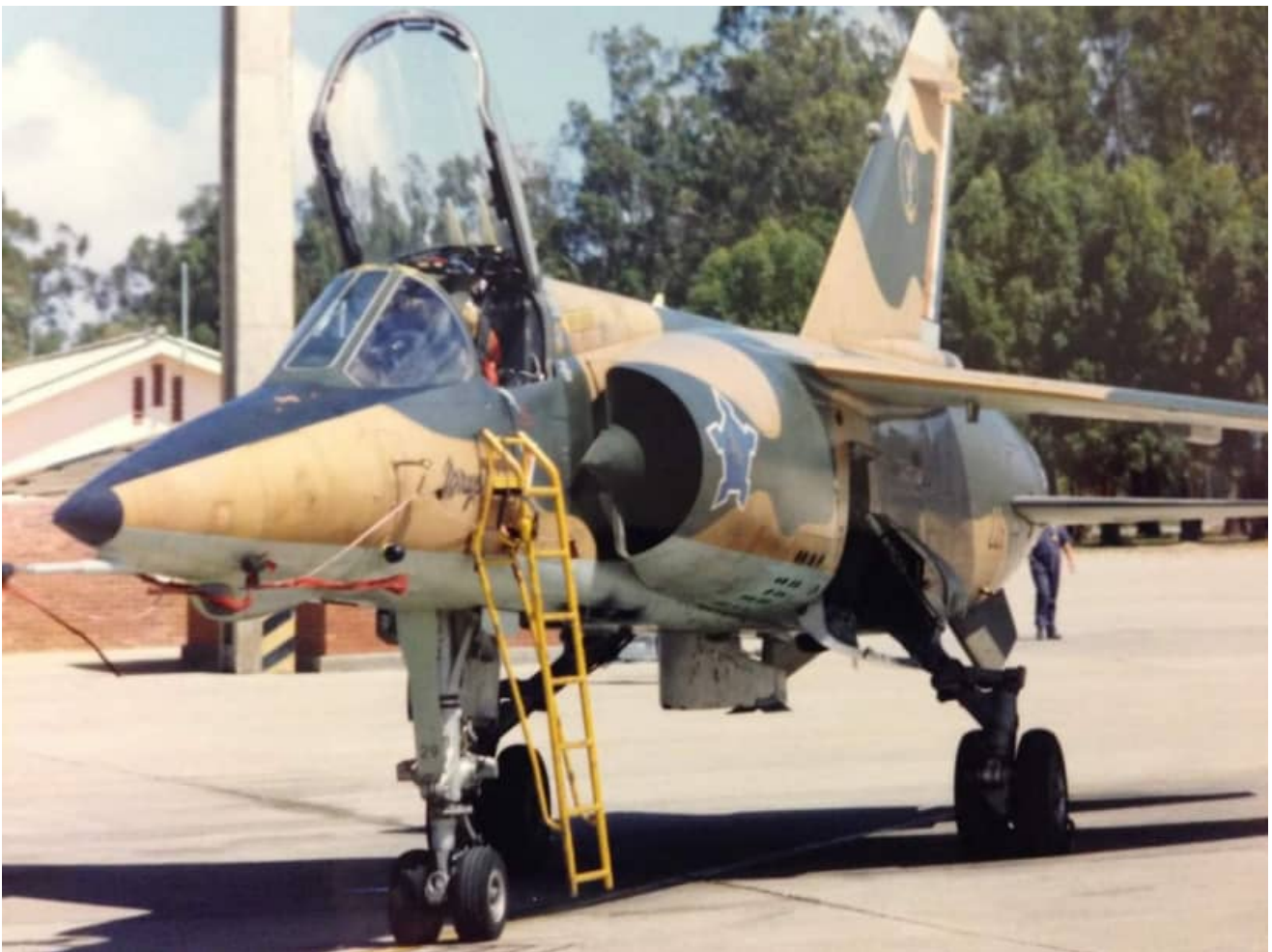
Two images of AZs #233 above and #229 below. #233 has the TFDC badge on the vertical stabilizer and the Castle with SAAF Eagle on the intake. #229 has the 1 Squadron badge on the vertical stabilizer and the original Castle and Springbok on the intake. Both aircraft have had the RWS installed, but #233 above has two non-standard black antennas located on the leading edge of the vertical stabilizer (as is indicated in other images provided elsewhere in this document). Note how the original camouflage on #229 has faded and weathered.
