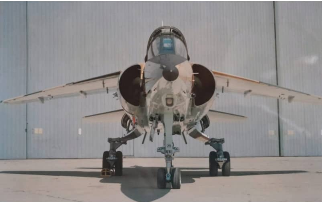
Two more images of #229. In the image below, the round laser designator can be seen in the housing beneath the nose. Note how the camouflage wraps around the underside of the wing and horizontal stabilizer leading edges.
