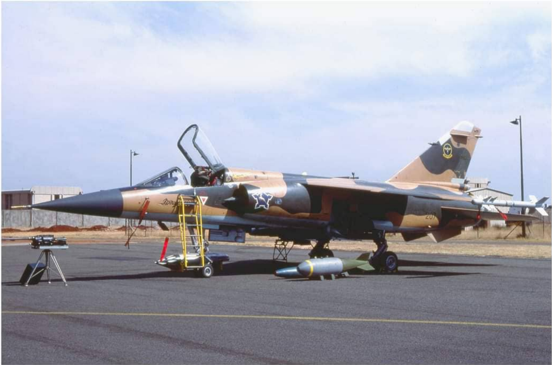
CZ #207 demonstrating some of the weapons which the CZ could carry. Matra 155 rocket pod, Mk.82 bomb, 450kg bomb and Matra R550 missile on the wingtip. One of the DEFA 30mm canon is displayed on the stand to the left. The F1 was fitted with two of these, one beneath each of the intakes.
