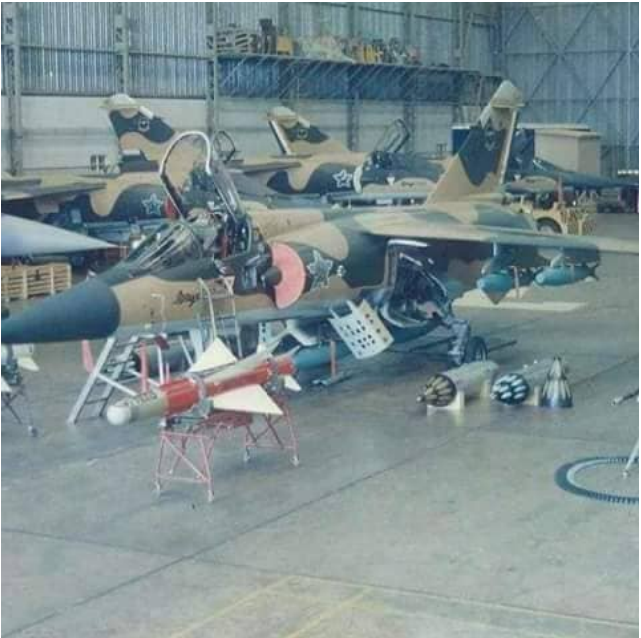
CZ on display. To note are the 8 x Mk 81 or 82 bomb configuration (4 on centerline bomb carrier, 1 on each wing station), Matra rocket pods on the floor and R530 missile on the stand in the foreground. Note that the Matra rocket pod to the right has the individual rockets protruding out of the nose cone (for display purposes) and the operational configuration with rockets inside and protected with frangible covers. The frangible covers would shatter as the rockets were fired.
