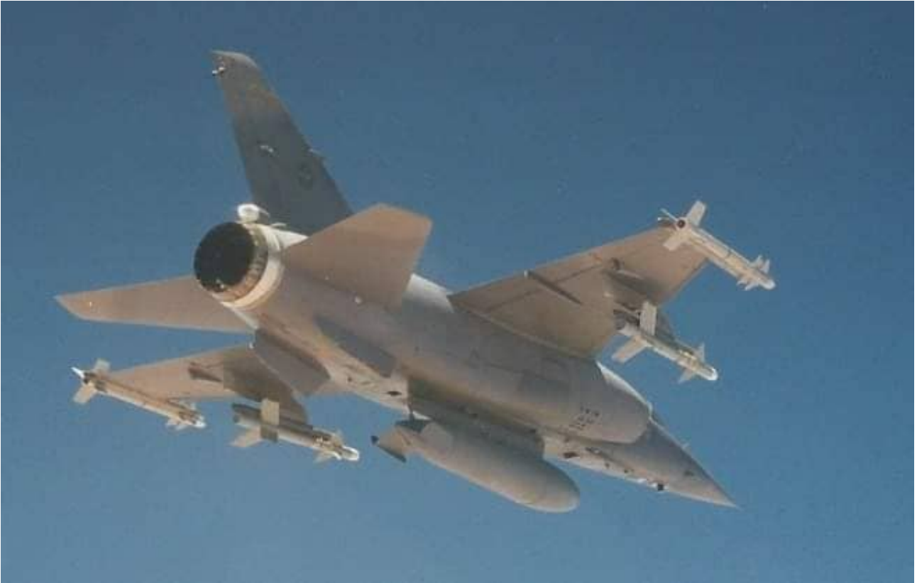
Images on this page and the next show the late configuration (post-RWS and RIMS mod state) of the CZ in the interceptor role – two V3S Snake IR missiles on the outboard wing hard points (station 2) and two R550 IR missiles on the wingtip launchers with a single RP35 external fuel tank on the centerline. The external fuel tanks were by this stage also camouflaged in a low visibility medium blue-grey colour.
