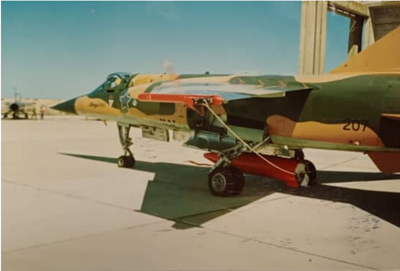
#207 above is fitted with a Taxan towed target drogue which is towed behind the aircraft and used for air-to-air gunnery practice. The Taxan agile target is highly manoeuvrable and contains a real time scoring device which counts rounds passing through a volume which is comparable in size to an enemy aircraft.
