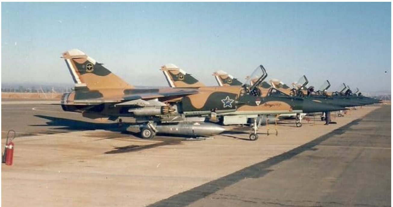
Two images of CZs carrying Matra 155 rocket pods on the inboard wing station and an RP35 external fuel tank on the fuselage centerline.
