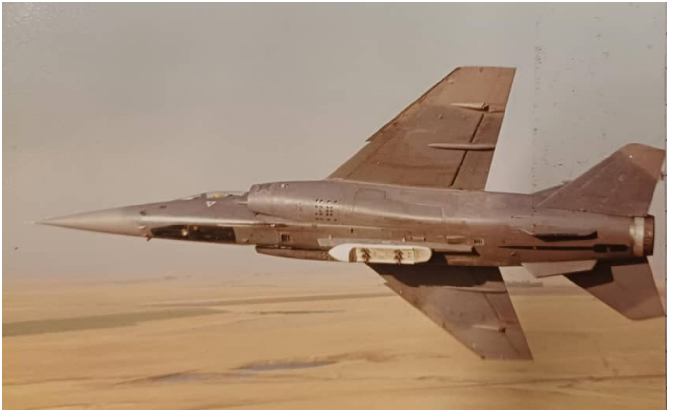
CZ carrying a single practice bomb carrier on the centerline. Note the false canopy and vertical stabilizer painted in black on the underside.
