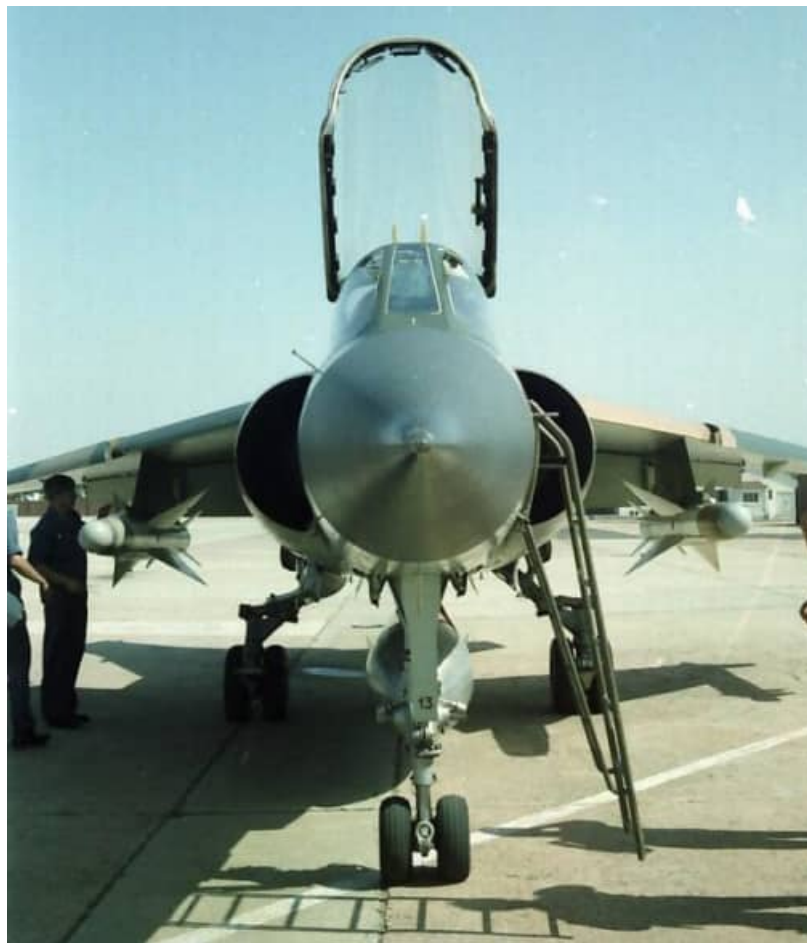
CZ #213 carrying SARH R530 missiles on the inboard wing pylons (station 1) and an RP35 external fuel tank on the fuselage centreline.
