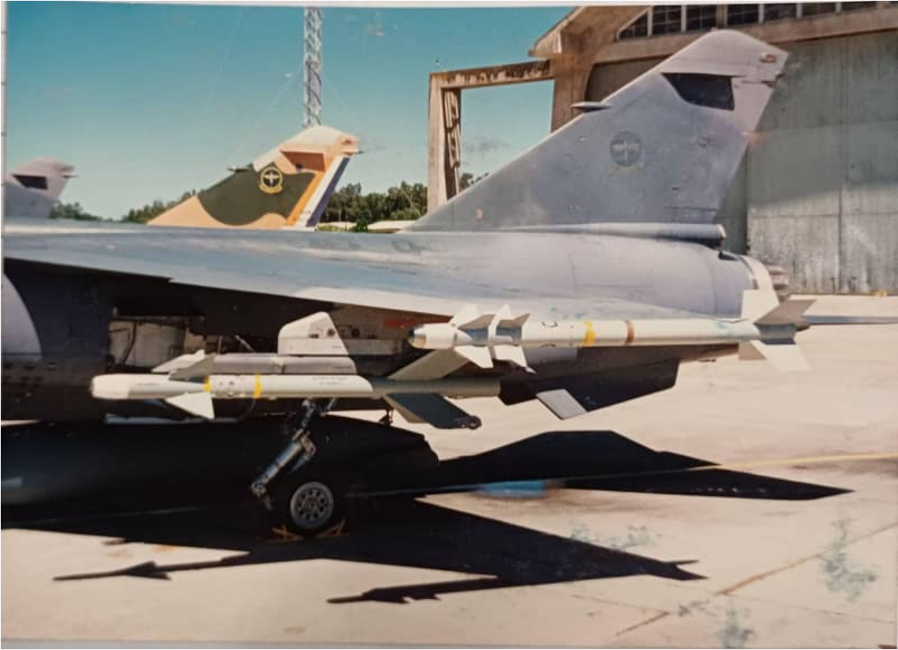
Two images of a CZ carrying V35 missiles on the outboard wing pylons. Notice how the V35 launch rail interfaces to the standard Station 2 pylon through and adaptor. The aircraft above is carrying an R550 missile on the wingtip station, whereas the aircraft below carries a V3B in this location.
