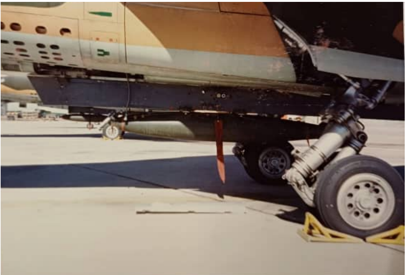
A pair of CZs carrying a single Mk.82 on the centerline pylon. This is not a combat typical load indicating they are preparing for a practice bombing sortie.
