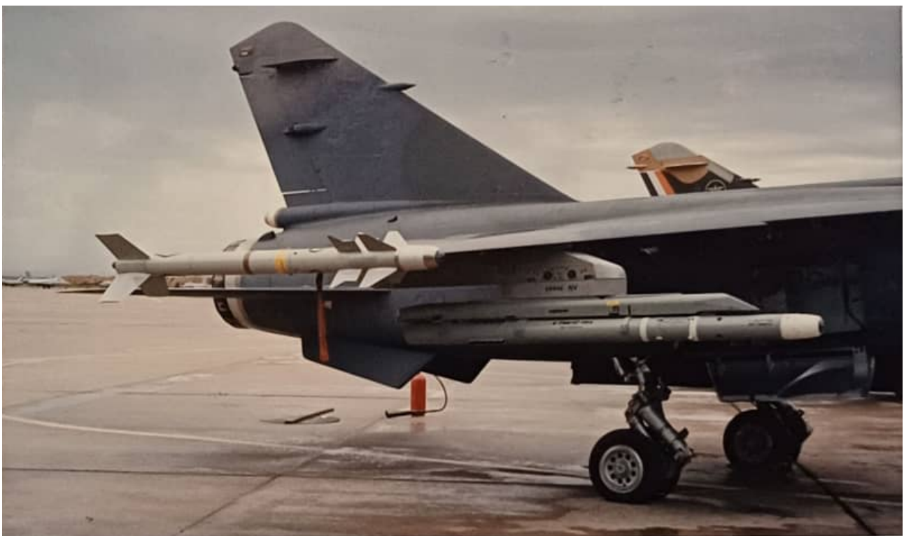
CZ #213 is fitted with a V3S CATM and a live R550 for missile firing practice. Due to the cost of live missile launches, this was not a common training activity. By the early 1990s, however, the R550 was considered old and outdated, making practice firing a good way to both dispose of them and provide live missile launch experience to pilots while doing so. The Squadron also fired V3Bs for the same reasons.
