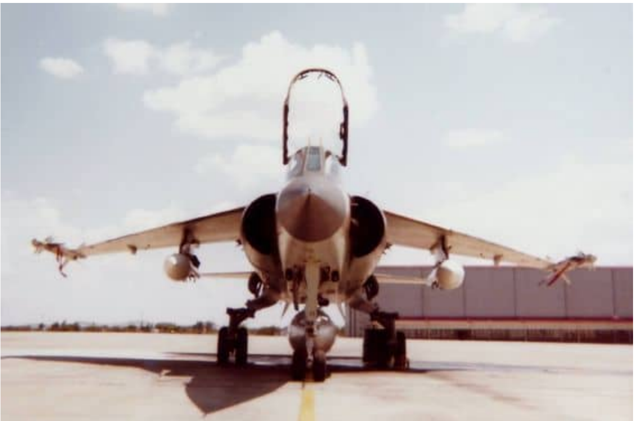
CZ with single RP35 external fuel tank, practice bomb carriers on the inboard wing stations and R550 missiles on the wingtips.
