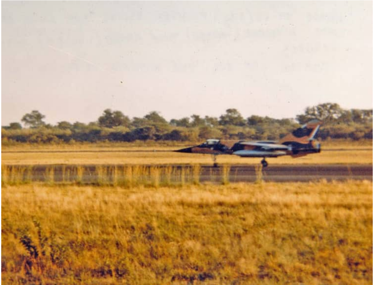
This CZ is seen operating from Mpacha Air Base in the Caprivi Strip in 1986 and is carrying an unpainted RP35 external fuel tank on the port inboard wing station – these would have been carried symmetrically on the wings. An R550 missile is carried on the wingtip station.
