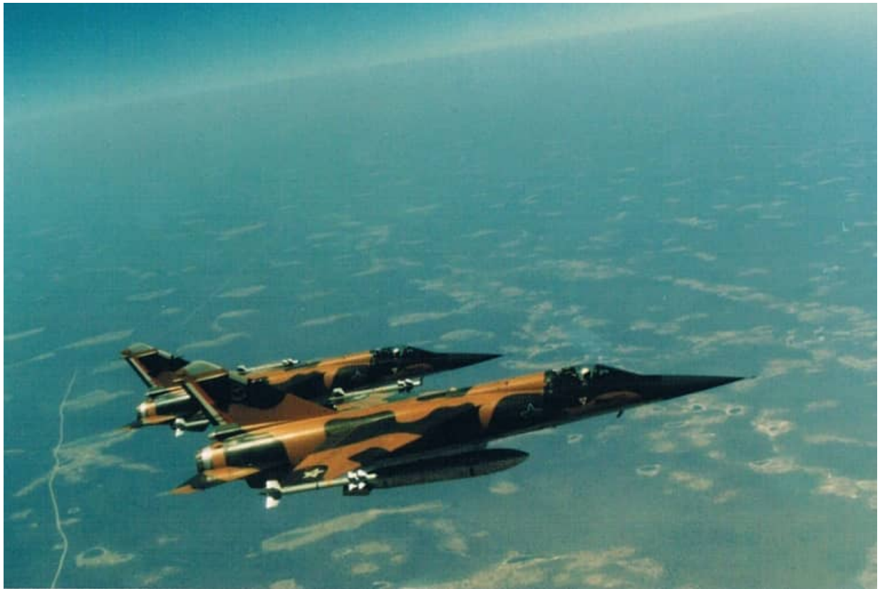
Two CZs in standard air intercept configuration with two R550 missiles and a single RP35 external fuel tank.
