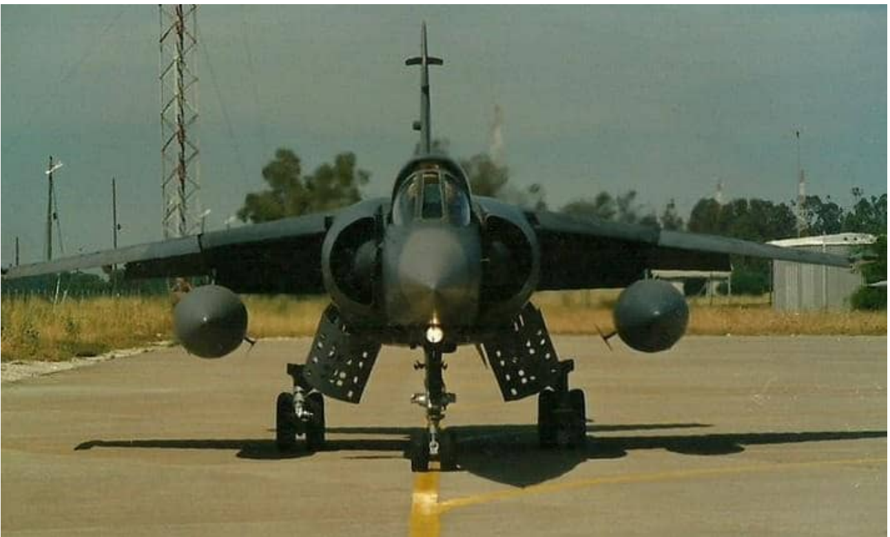
CZ in low visibility three tone blue/grey camouflage carrying two RP35 external fuel tanks on the inboard (station 1) pylons. These tanks are painted in the medium blue-grey PE Blue colour.
