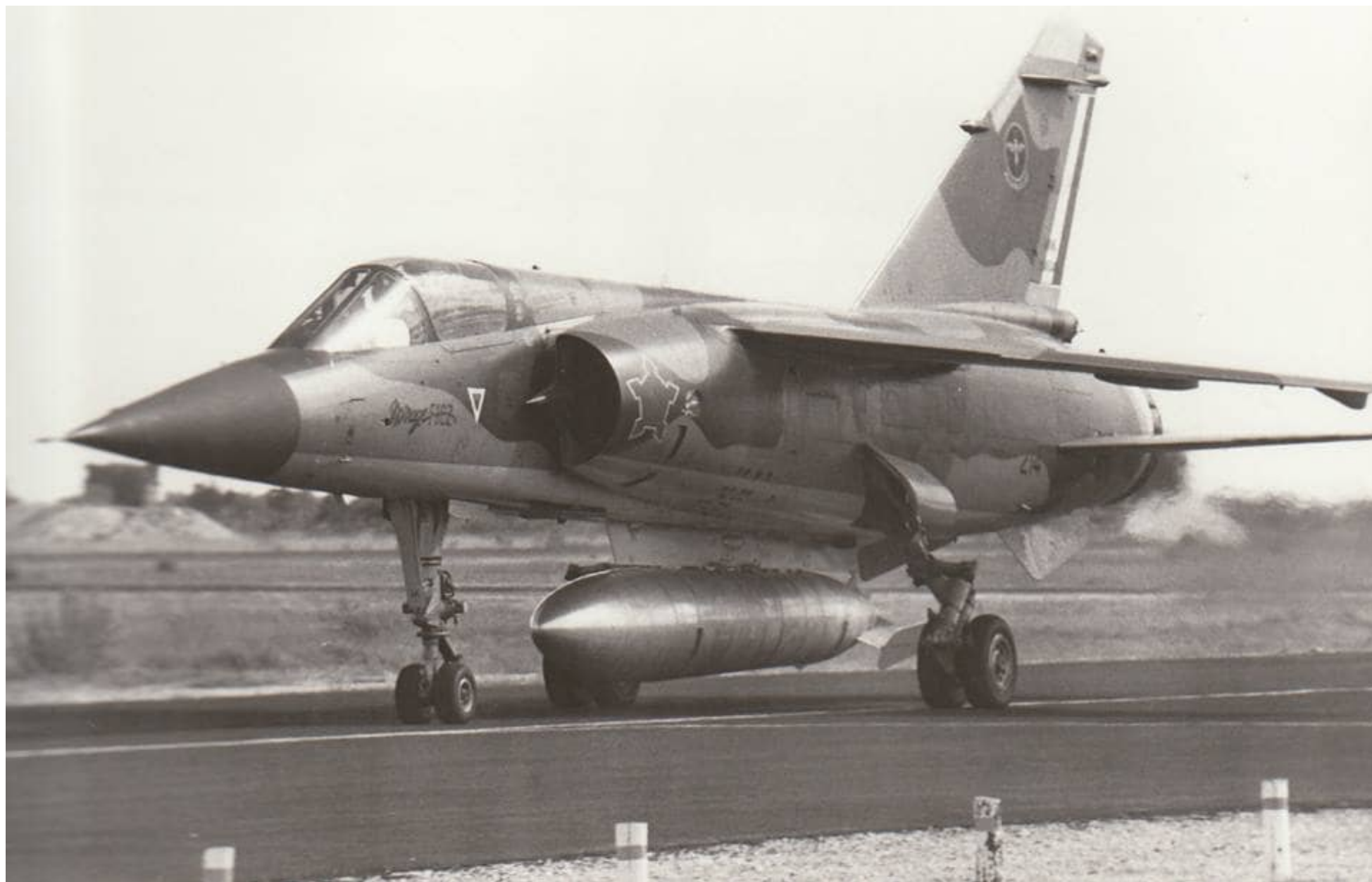
CZ #214 with single RP35 1,200 liter external fuel tank. #214 is in the original delivery scheme with a complete set of high visibility markings.
