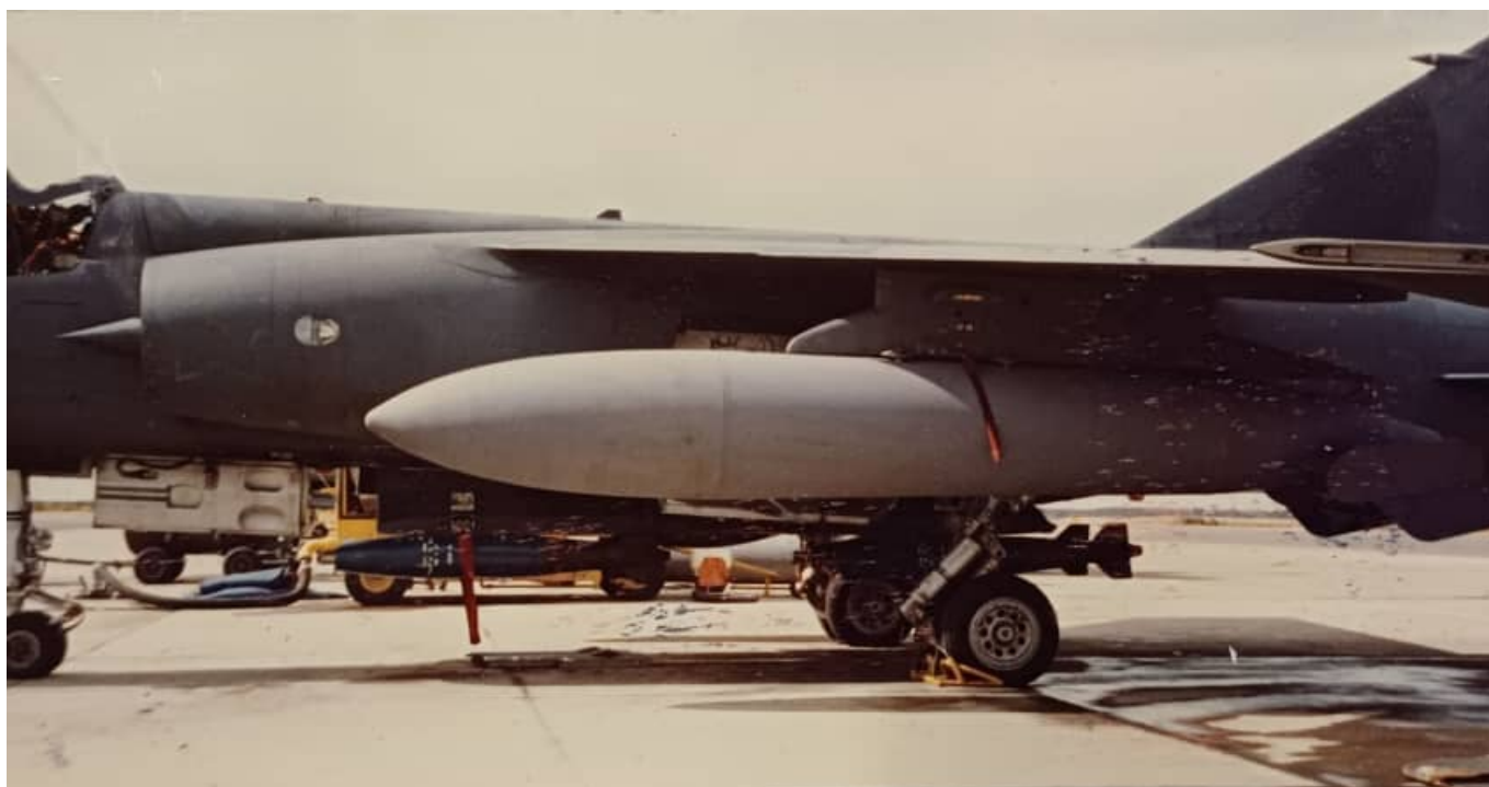
CZ carrying the CLB4 with four Mk. 82 bombs on the centerline and external fuel tanks on the wings – these are painted in a light grey.
