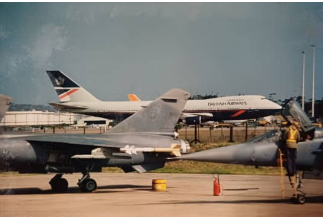
CZ shown carrying a dummy V3S launcher on the port outboard wing station and a V3C test article on the wingtip.
