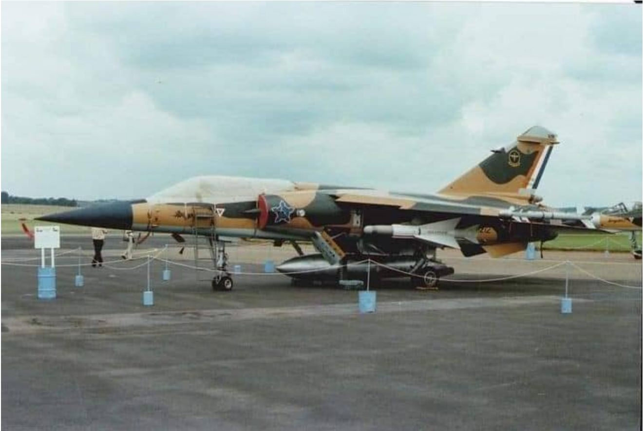
Two images of CZ #212 on airshow display duty with a standard air intercept load of two R530s, two R550s and a 1,200 liter fuel tank. The R530 was not used by the SAAF in combat operations. The external fuel tank is unpainted.
