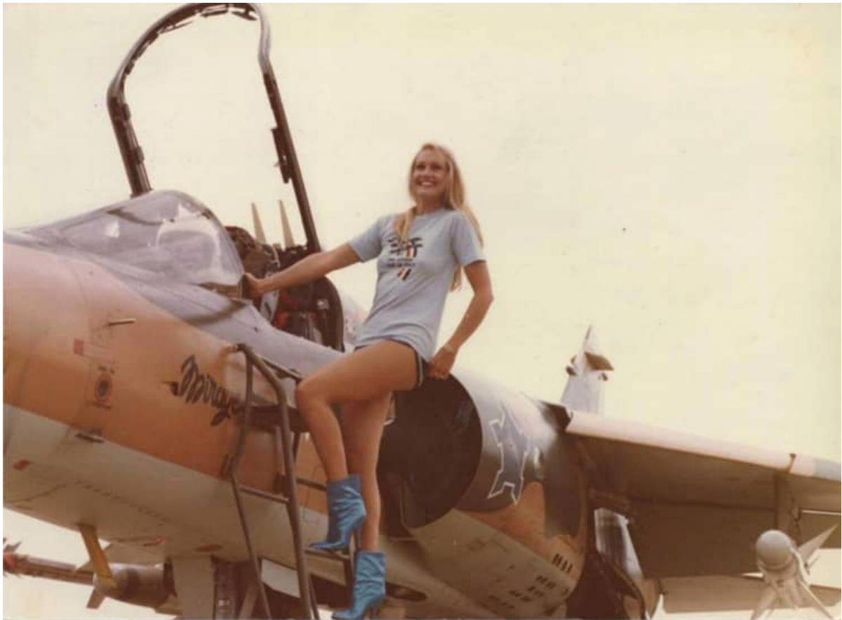
Interesting photograph apart from the obvious... a CZ in delivery camouflage with Matra SARH R530 missiles on the inboard wing pylons (station 1) and R550 IR missiles on wingtip pylons.
