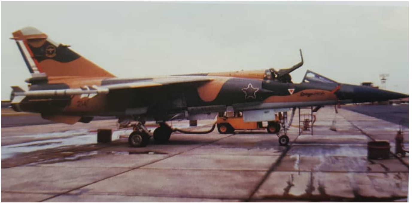
CZ #214 with wingtip mounted R550 IR guided air-to-air missiles.
