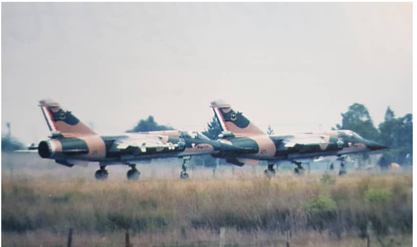
One of the CZs above is carrying wingtip mounted R550 missiles.
