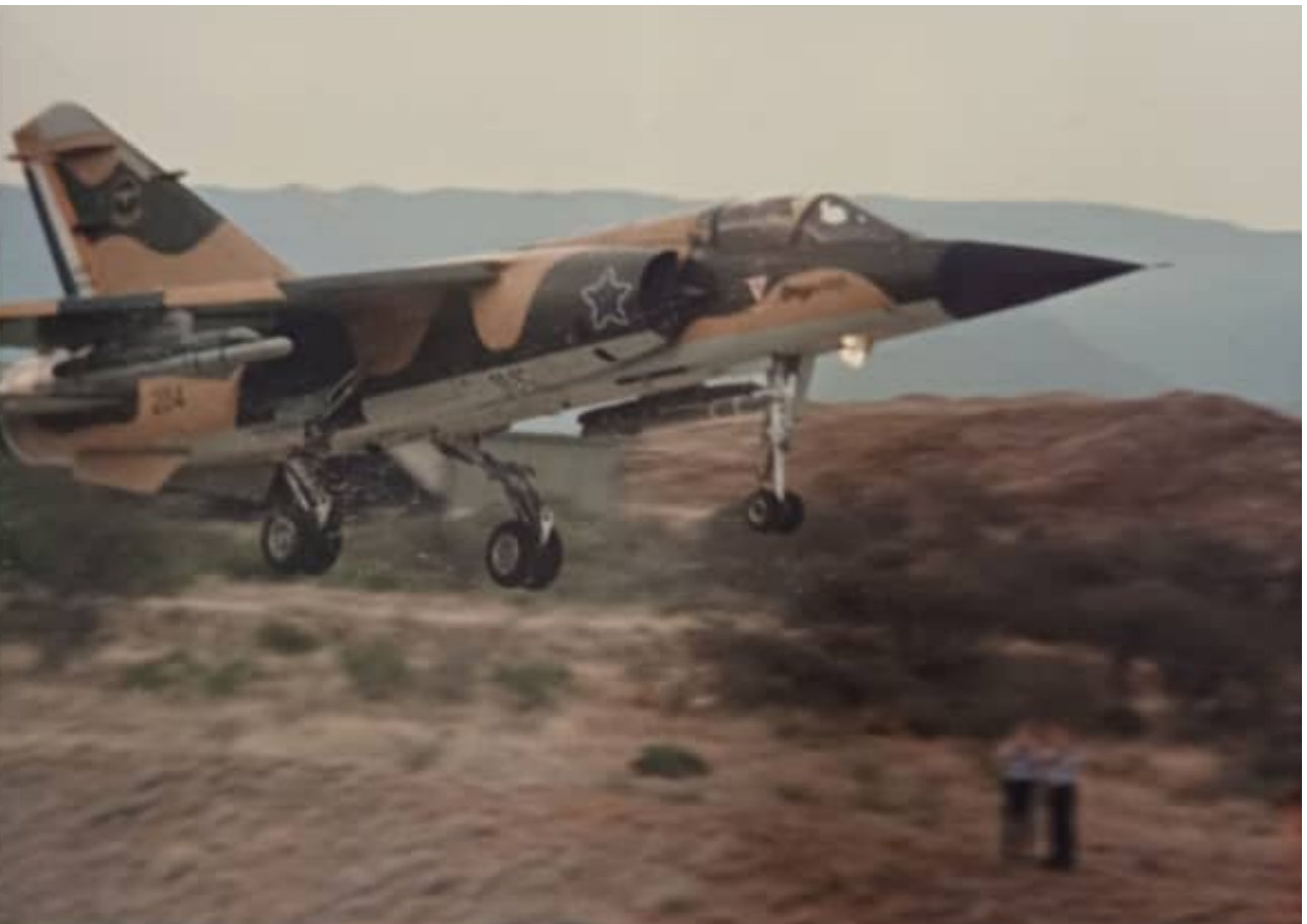
These images show the typical ACM training configuration in the last years of service, with a single V3S Captive Air Training Missile (CATM) under each wing. These are missiles with inert motors and warheads, but with live IR seeker heads for use during training. They typically have their steering fins and wings removed to reduce store drag and mass. CZ #204 below has a CATM on the port wing and a dummy missile (mass representative only) on the starboard wing.
