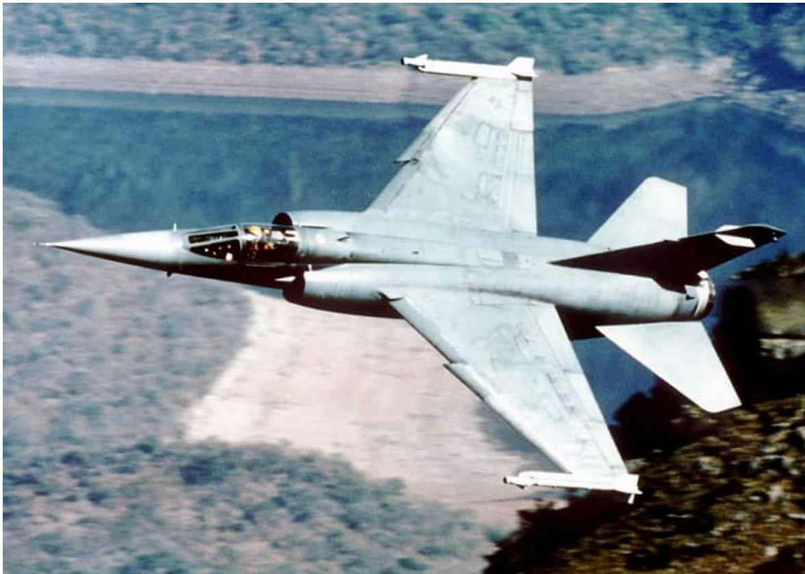
CZ with what appears to be V3B infrared missiles on the wingtips. Barely visible is the V3B canard fin configuration which is distinctly different to the Matra R550. The CZ was unlikely to have used the V3B in combat operations, favoring the R550. This aircraft has the RWS installed.
