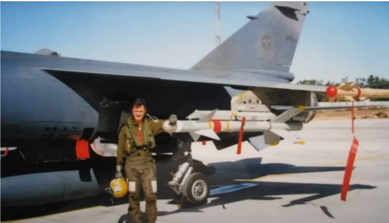
Two images of a CZ carrying V35 missiles on the outboard wing pylons. Notice how the V35 launch rail interfaces to the standard Station 2 pylon through and adaptor. The aircraft above is carrying an R550 missile on the wingtip station, whereas the aircraft below carries a V3B in this location.
