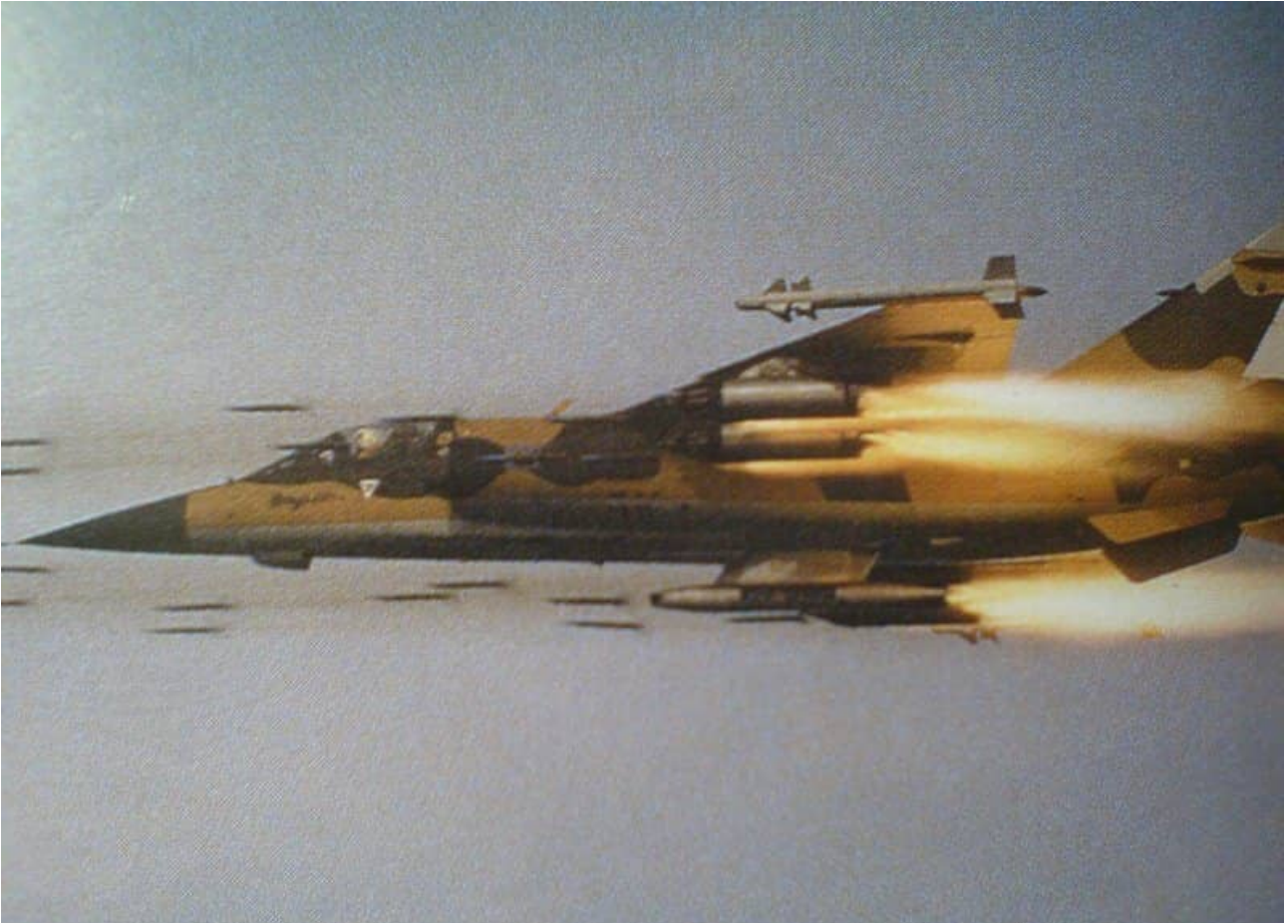
Not a common CZ load: Four Matra 155 rocket pods housing 18 SNEB 68mm rockets each. This appears to be a test firing of all four pods simultaneously. Note the rearward facing camera housing beneath the nose as well as what could be a flight test data link pod on the centerline. The missiles on the wingtips are Matra R550 IR missiles.
