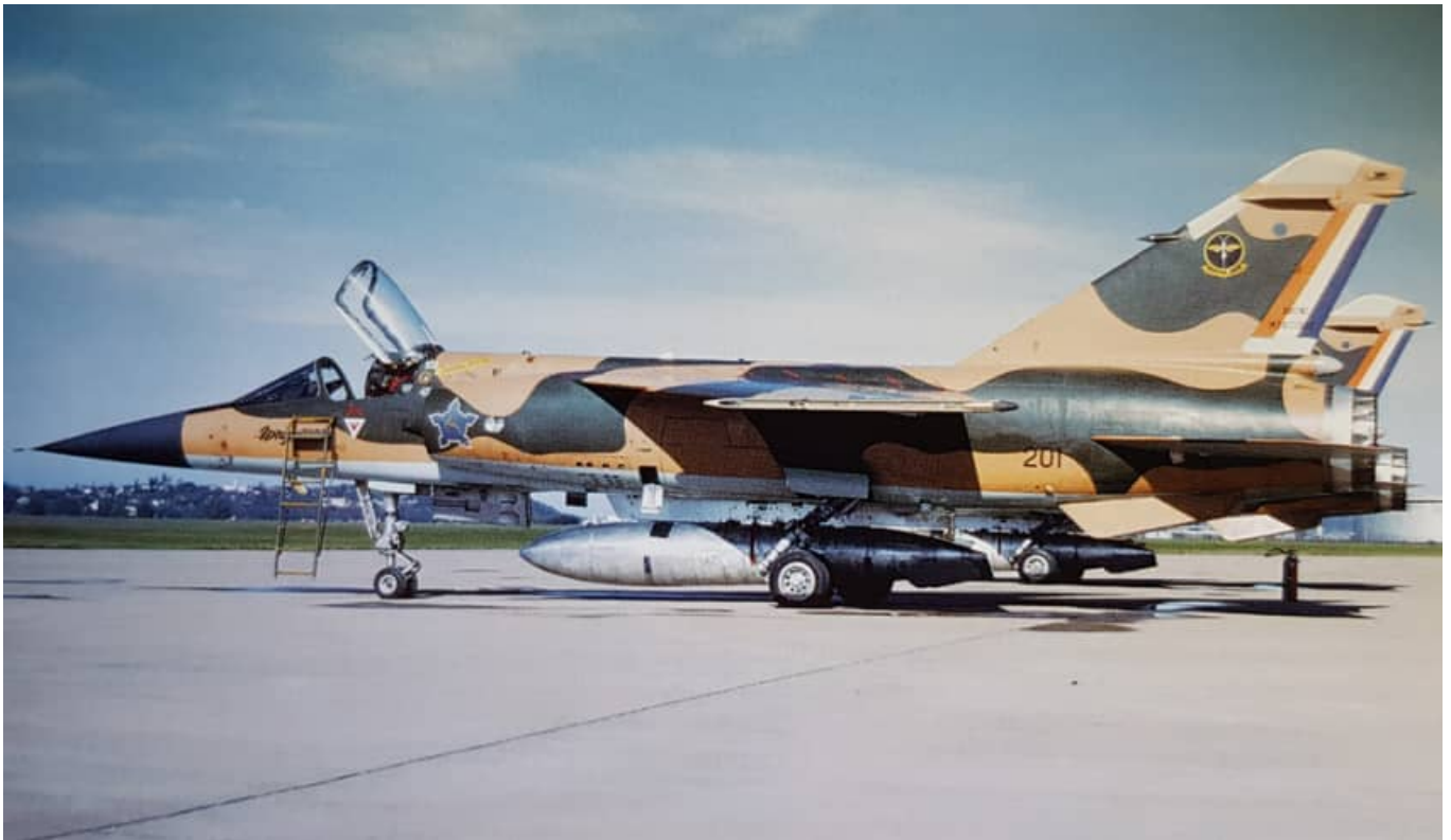
CZ #201 (above) and #211 (below) each carrying a single RP35 1,200 liter external fuel tank. These fuel tanks were initially unpainted as in these images. However, they were later painted medium blue-grey colour when the CZ received the three tone low visibility blue-grey camouflage. Wingtip missile launchers are fitted to both aircraft.
