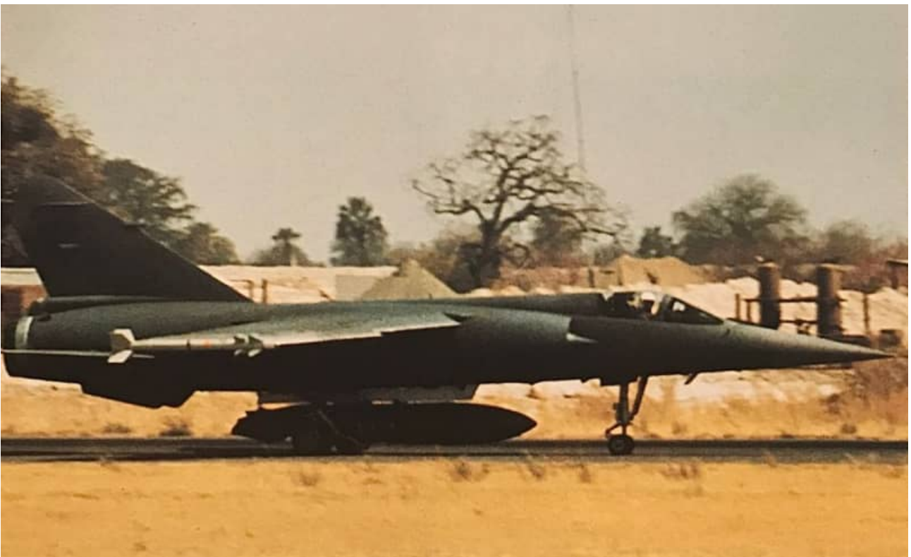
Two CZs carrying RP35 external fuel tanks and R550 missiles. This photo was taken in the Operational Area during the Border War, most likely Ondangwa. It would appear that the fuel tank in the image below has been painted in the low visibility medium blue-grey colour. The grey CZ is possibly #203 during the operational assessment of the low visibility camouflage scheme.
