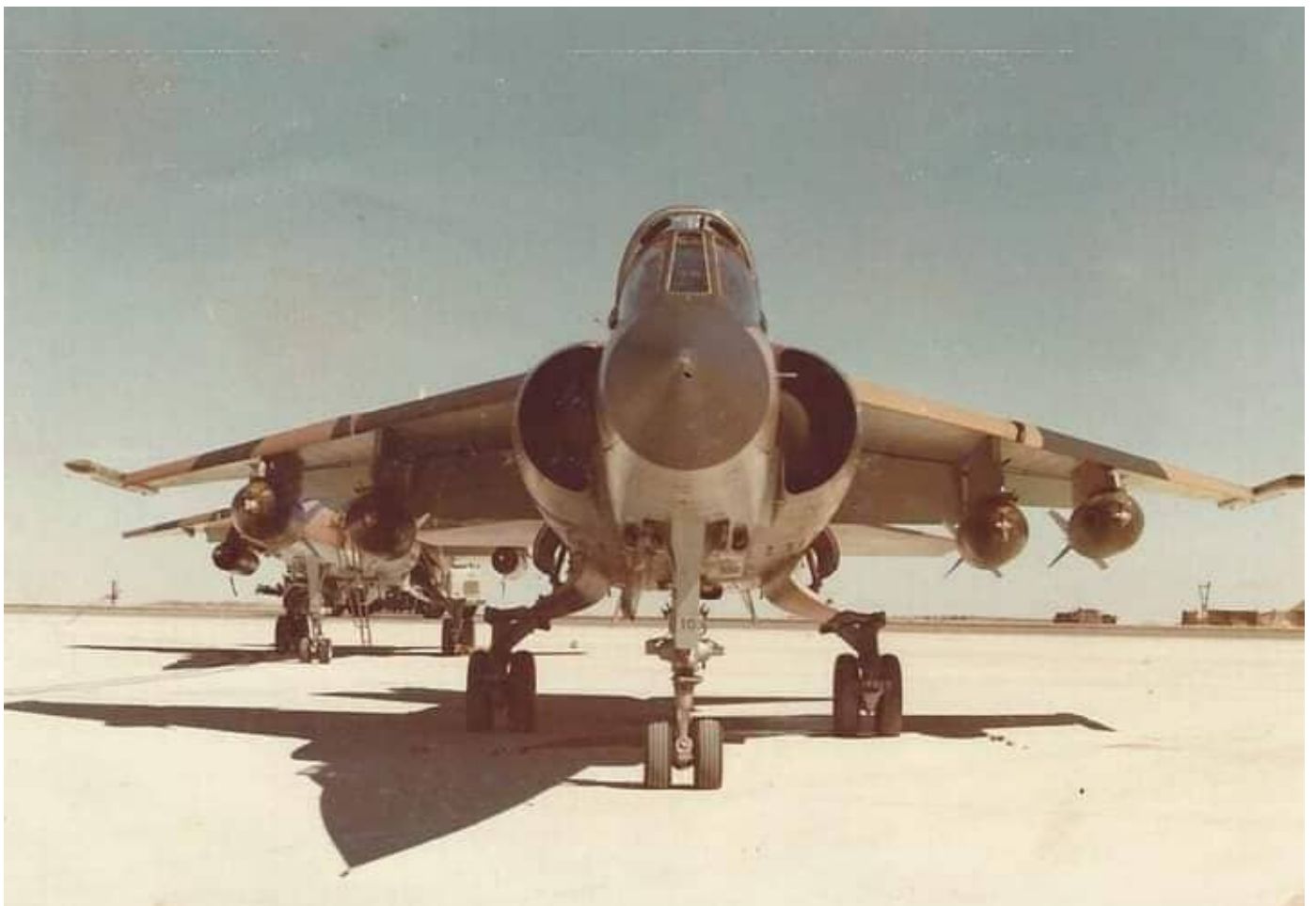
CZ #210 carrying what look to be four 450kg bombs, one on each of the underwing hardpoints. This was an unlikely operational load for the CZ.
