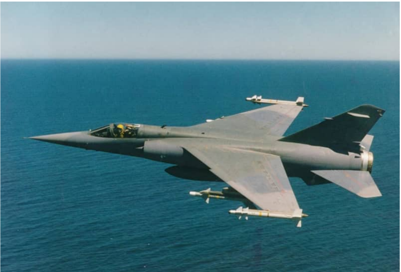
Images on this page and the next show the late configuration (post-RWS and RIMS mod state) of the CZ in the interceptor role – two V3S Snake IR missiles on the outboard wing hard points (station 2) and two R550 IR missiles on the wingtip launchers with a single RP35 external fuel tank on the centerline. The external fuel tanks were by this stage also camouflaged in a low visibility medium blue-grey colour.
