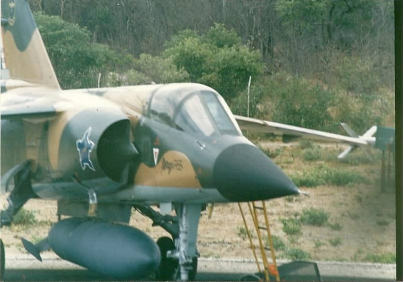
CZ with a single RP35 1,200 liter centerline tank and R550 missile on the wingtip launcher. The tank appears to have been painted in an overall medium blue-grey PE Blue colour.
