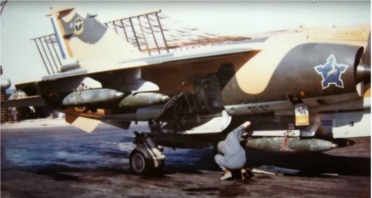
Another view of a CZ (note the 3 Sqn badge on the tail) armed with eight Mk.82 bombs. Just visible to the left of the photo is the protective cover for the R550 IR seeker.
