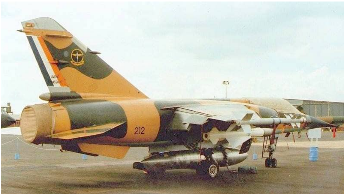
Two images of CZ #212 on airshow display duty with a standard air intercept load of two R530s, two R550s and a 1,200 liter fuel tank. The R530 was not used by the SAAF in combat operations. The external fuel tank is unpainted.
