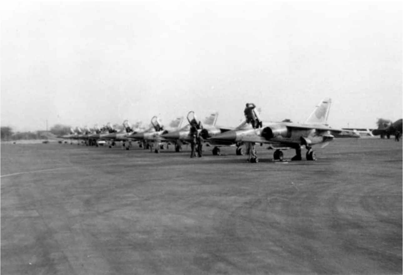
A flock of CZs on the flightline during Operation Protea in 1981. They are equipped with the CLB4 4-bomb carrier on the centerline station. The aircraft on the right carries R550 missiles on the wingtips.
