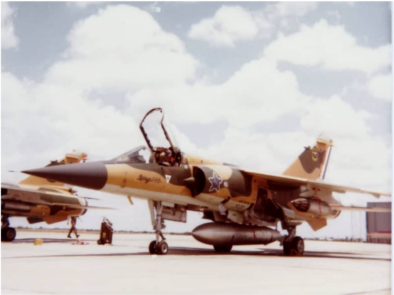
Two images of CZs carrying Matra 155 rocket pods on the inboard wing station and an RP35 external fuel tank on the fuselage centerline.
