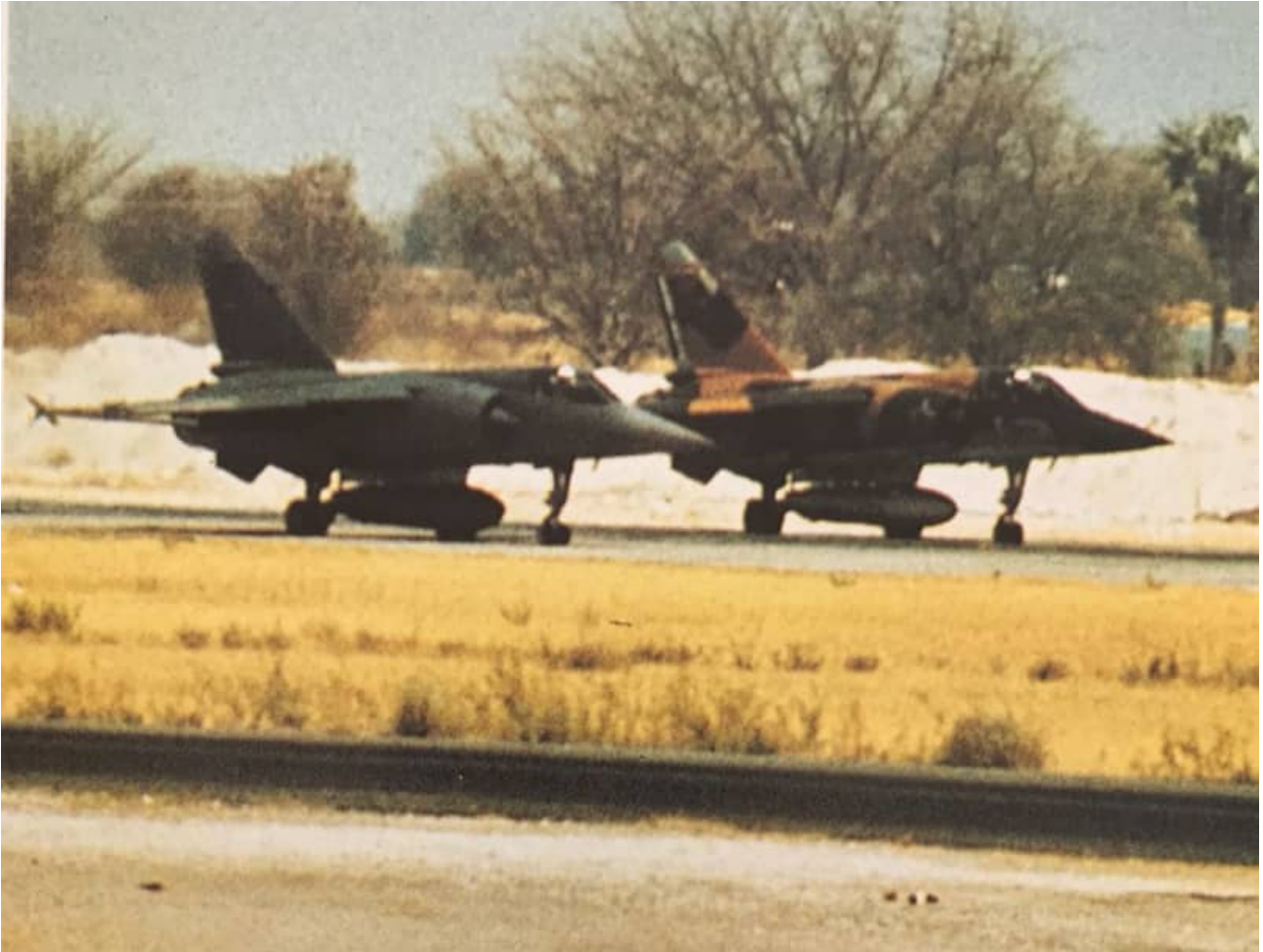
Two CZs carrying RP35 external fuel tanks and R550 missiles. This photo was taken in the Operational Area during the Border War, most likely Ondangwa. It would appear that the fuel tank in the image below has been painted in the low visibility medium blue-grey colour. The grey CZ is possibly #203 during the operational assessment of the low visibility camouflage scheme.
