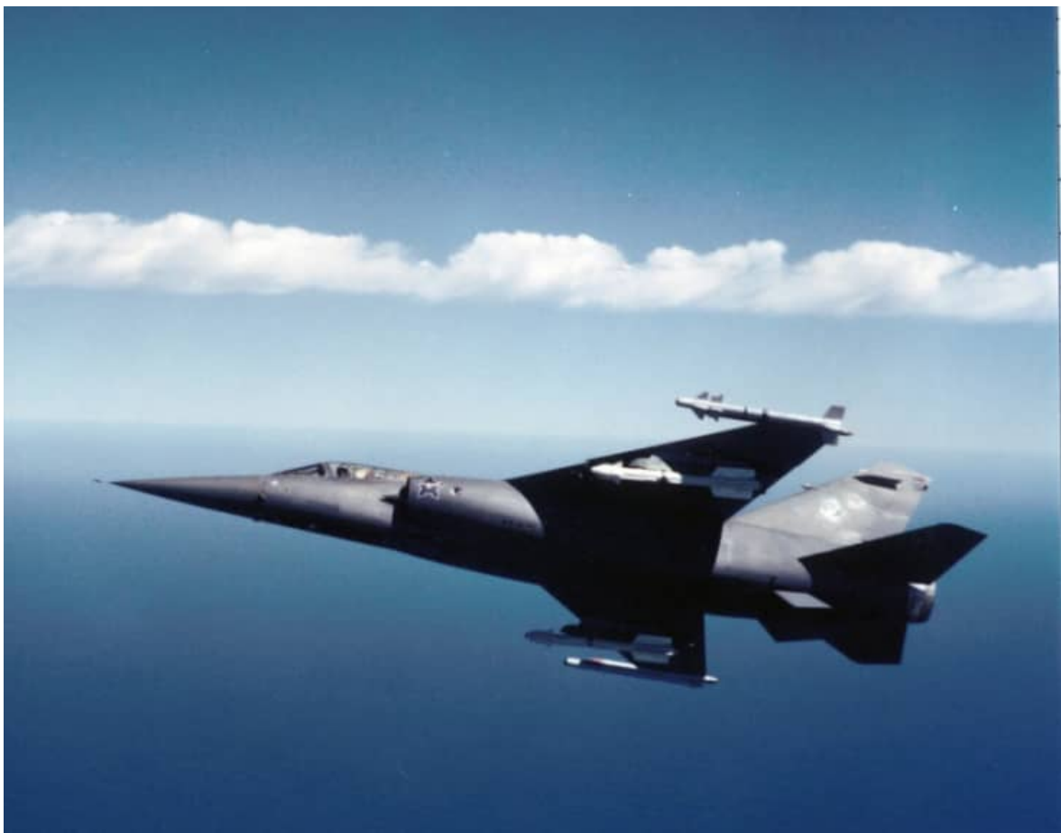
This image shows the installation of Russian Vypel R73 (NATO name AA-11 Archer) infrared air to air missiles on outboard wing stations of the F1CZ. R550 missiles are carried on the wingtips. The R73 was integrated and successfully test fired from the CZ, but was not taken into service by the SAAF despite a number being acquired.
