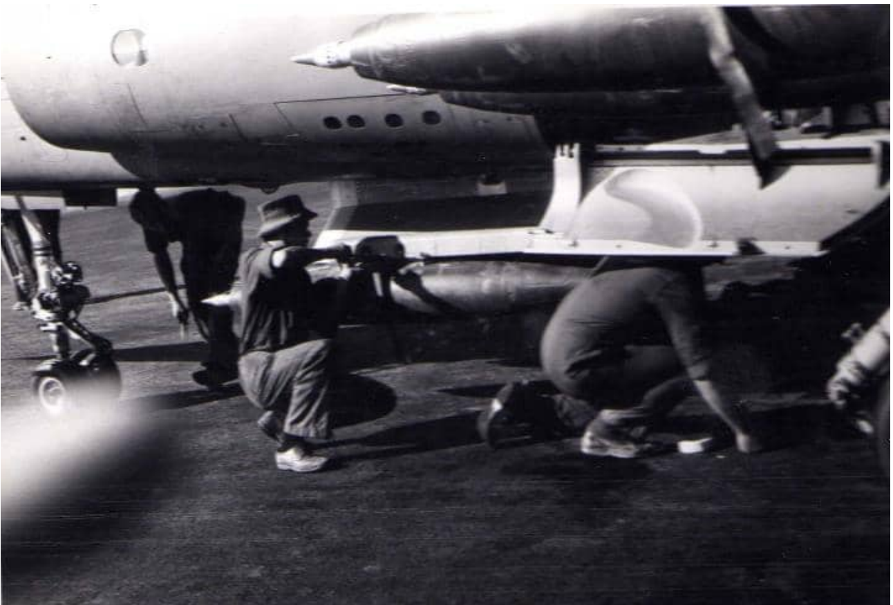
Interesting image of a CZ (note the spotlight on the intake) carrying the CLB4 4-bomb carrier which is being loaded with what look like Mk.82 bombs. There is also one Mk.82 on each of the wing pylons, for a total load of eight bombs.
