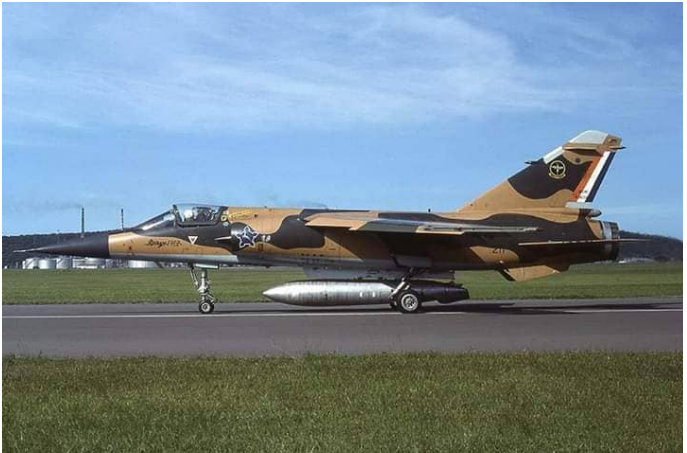
CZ #201 (above) and #211 (below) each carrying a single RP35 1,200 liter external fuel tank. These fuel tanks were initially unpainted as in these images. However, they were later painted medium blue-grey colour when the CZ received the three tone low visibility blue-grey camouflage. Wingtip missile launchers are fitted to both aircraft.
