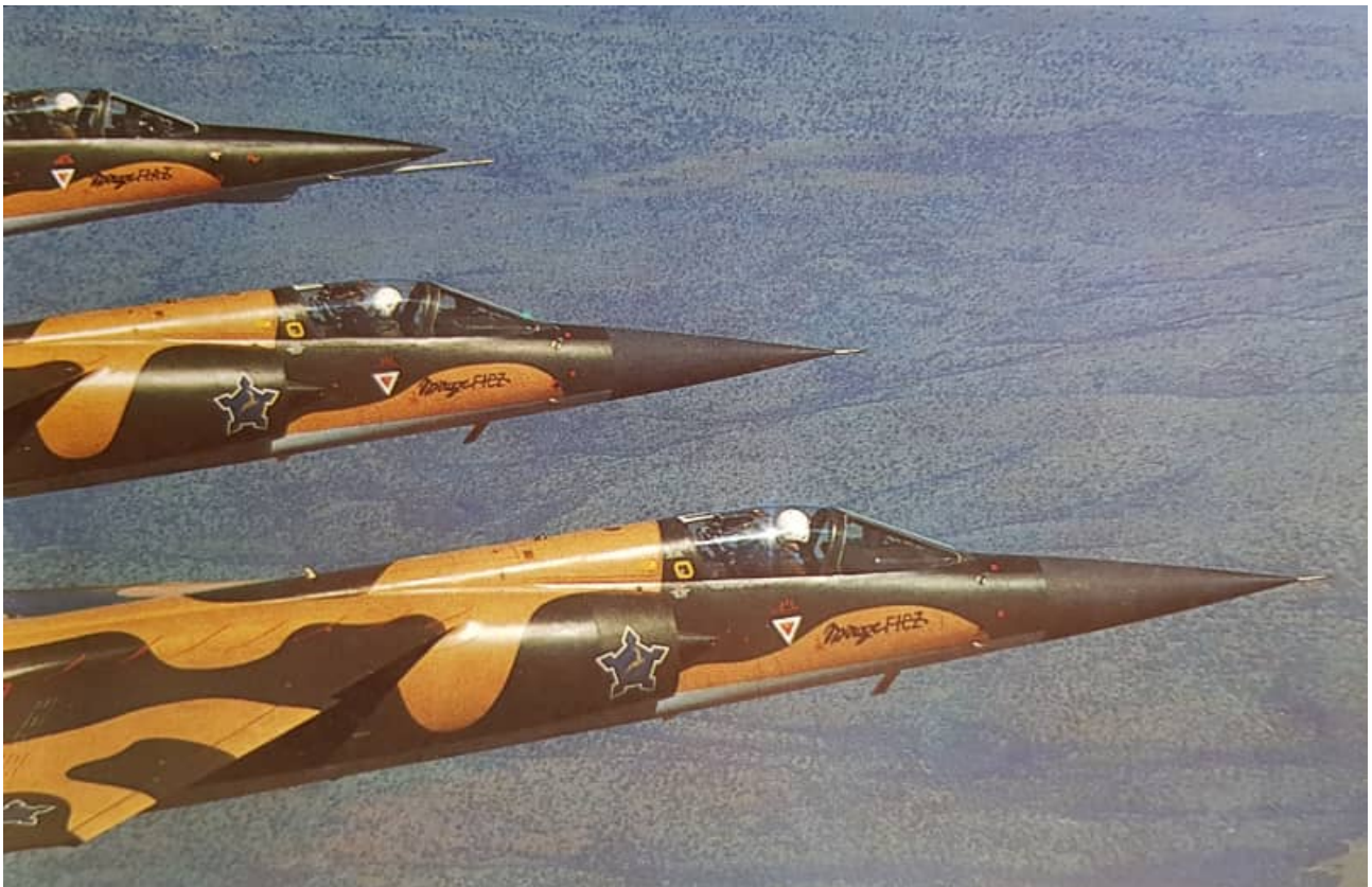
The SAAF Castles (24") are blue surrounded by white. The Springbok is gold (and not yellow) and faces forward on the fuselage and inwards on the wings with legs towards the trailing edge. Note the location of the Castles on the upper wing surface. The yellow surround to the emergency canopy jettison handle is visible behind the canopy. Prominent ejection seat triangles are displayed beneath the canopy. The red diagonal stripes along the wing / fuselage junction are visible- these are not all applied at the same angle. The third aircraft is an AZ. The underside colour appears to be a very pale blue.
