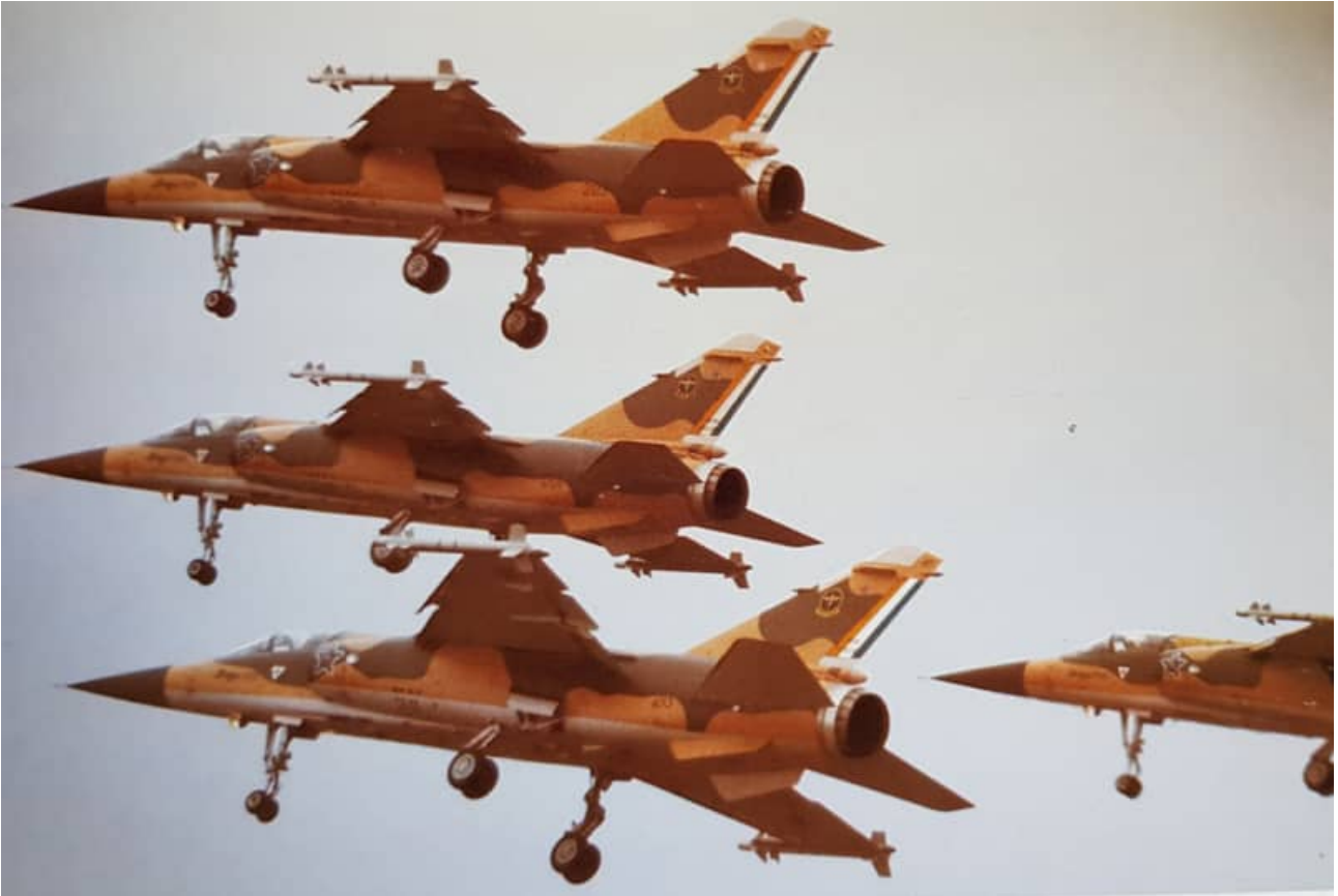
Four CZs in the delivery camouflage scheme. 3 Squadron "Wasp" badges are on the vertical stabilizers. All four carry the Matra R550 IR air-to-air missile on the wingtip launchers. Note the spotlight on the intake used for night intercepts. The AZ did not have the spotlight. It would appear that none of these aircraft have the Castles applied to the lower wings.
