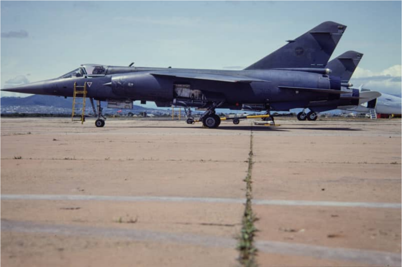
Ysterplaat AFB. CZ #209 with what appears to be freshly applied Castles, 3 Squadron badge and other markings. This image reflects the characteristic nose up stance of the F1. #209 has the upgraded RWS suite – note the cylindrical RWS antenna beneath the lower forward fuselage. Several access panels are open on the aircraft underside.
