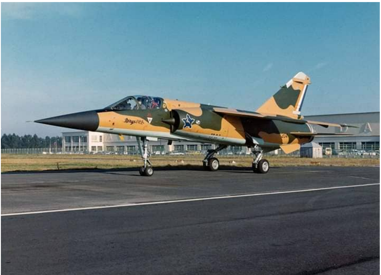
CZ #204 fresh off the production line in France. All markings have been added except for the 3 Squadron badge on the vertical stabilizer. Note the night intercept light on the intake just aft of the Castle. With hydraulic power on the main gear and nose gear doors were closed for takeoff and landing, only opening during cycling of the landing gear. #204 demonstrates the typical nose up attitude of the F1.
