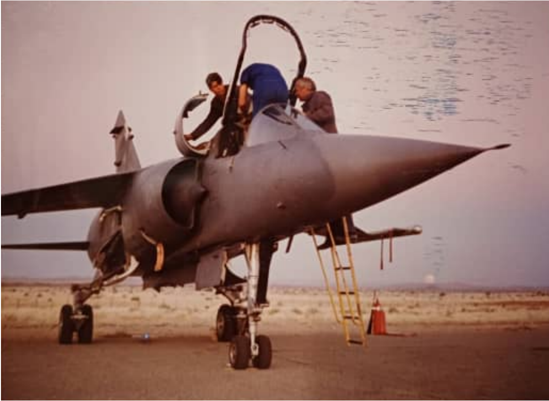
Unknown CZ at Upington in June 1989. The aircraft is not yet equipped with RWS or RIMS. Note the black nose gear doors indicating a false canopy has been applied.
