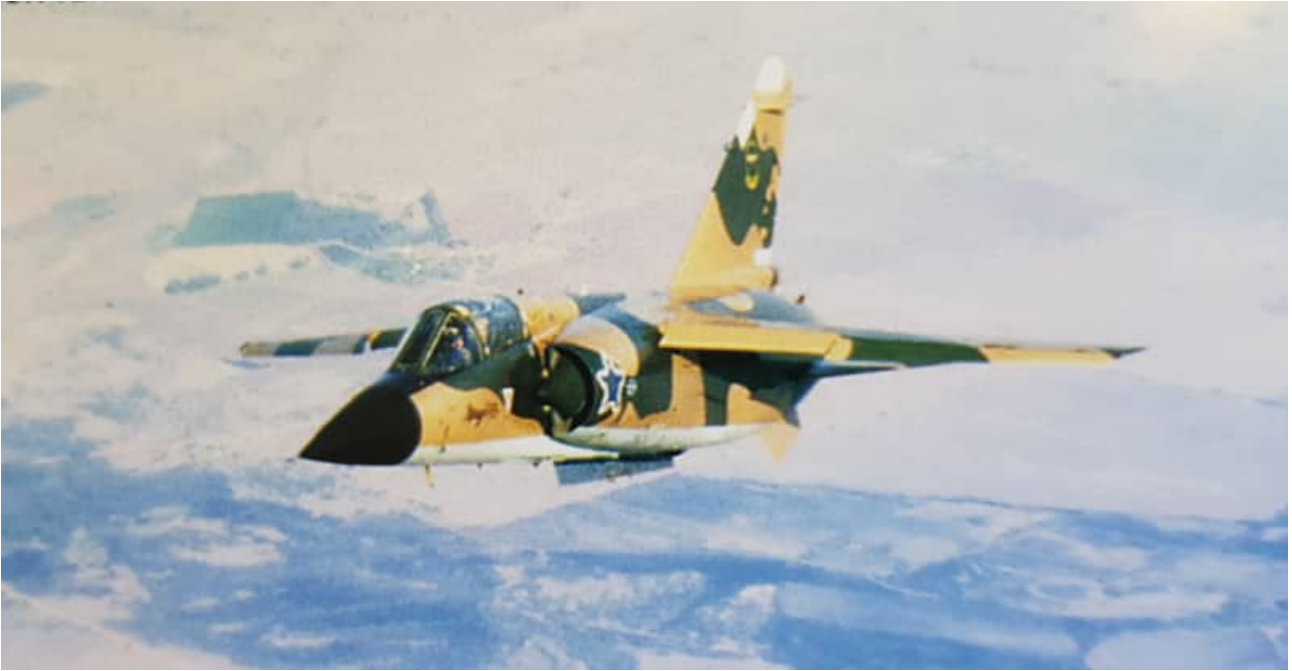
CZ with a centerline external fuel tank pylon installed. Note how the outer surface of the ventral stabilizer is painted in buff. The inner surfaces were painted in the underside colour. The camouflage is carried partially into the intakes and on the shock cone as can be seen in this image. The F1 has its leading edge slats and flaps in extended/drooped position in this image. Note the black anti-glare panel between windshield and radome.
