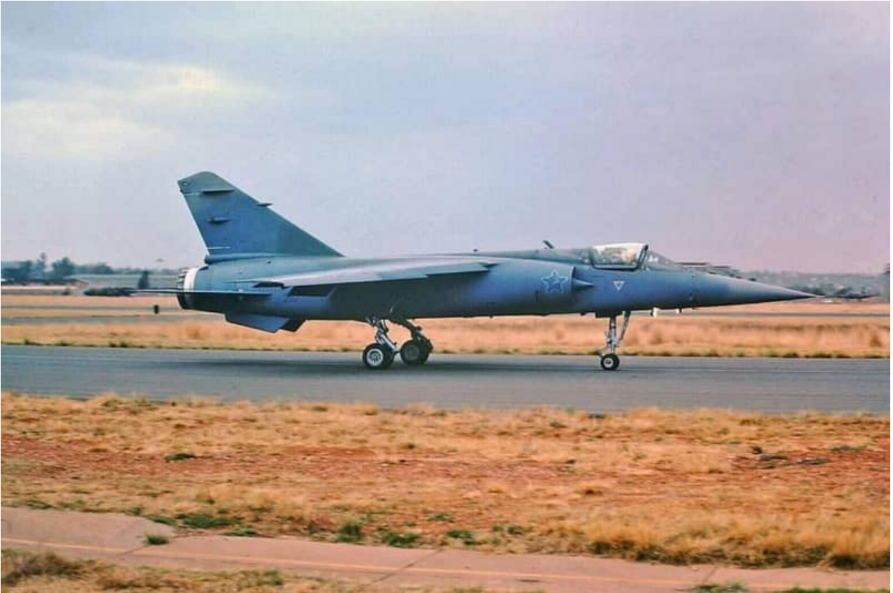
CZ #210 with prominent Castles on the intakes. The camouflage appears to be freshly applied. Both aircraft on the page have the RWS and RIMS ventral fins installed. The UHF blade antenna has been relocated to the spine aft of the cockpit. #205 below has had the 3 Squadron badge on the vertical stabilizer painted over. Note how variable the greys/blues appear in the two images – a product of light and photo processing. #205 below has a single medium grey painted nose cone.
