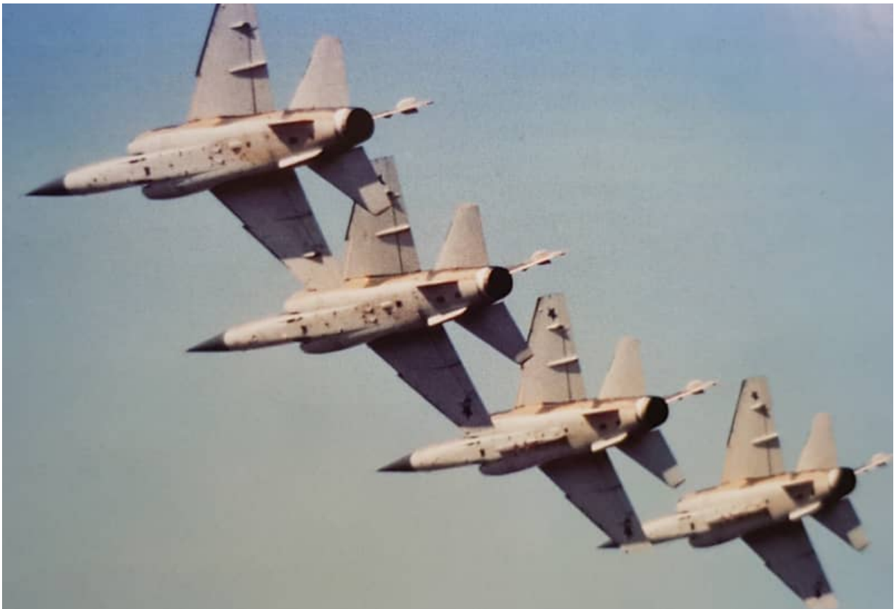
SAAF CZs were delivered with a light grey (Light Admiralty Grey) lower colour as seen in the image above. This was changed later to a very light blue, as is visible in some images in this volume. Note the location of the under-wing Castles (24" size) on three of the CZs and how the upper surface colours wraparound onto the lower leading edges of the wings and stabilizers. The F1 on the left does not have the Castles on the lower wings. These aircraft have the original ventral fins without the later chaff/flare dispensers. The right two CZs carry a centerline RP35 external fuel tank pylon. All four CZs are devoid of the wingtip missile launcher rails.
