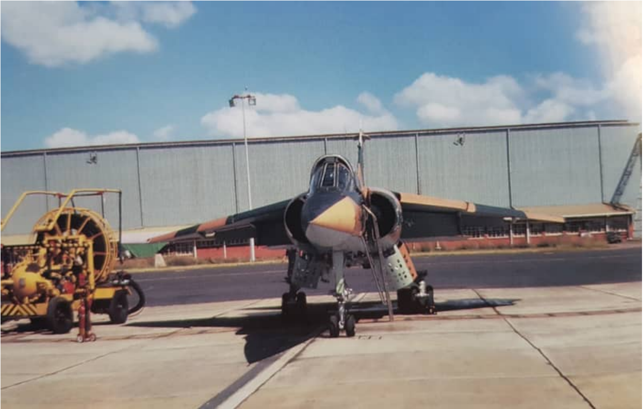
As always, there are exceptions to the norm. This CZ does not have a black radome. This is most likely a ballast nose, which would have been installed when the radar had been removed. This was not very common judging by available images of CZs. The buff and grey colours on the nose are also clearly brighter than the colours on the rest of the aircraft.
