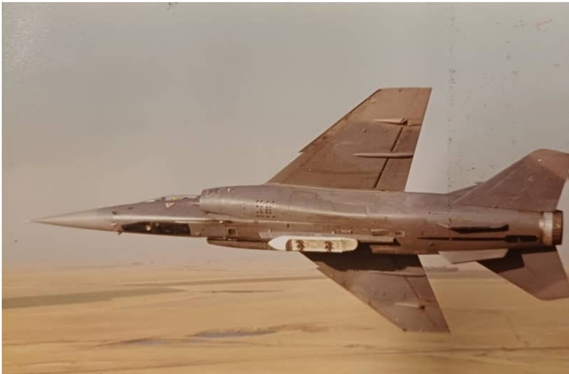
Another view of the false canopy and tail seen on #209. The aircraft is in a post RWS and RIMS mod state. Note again the lack of castles under the wings. The aircraft is carrying a practise bomb rack on the centreline station.
