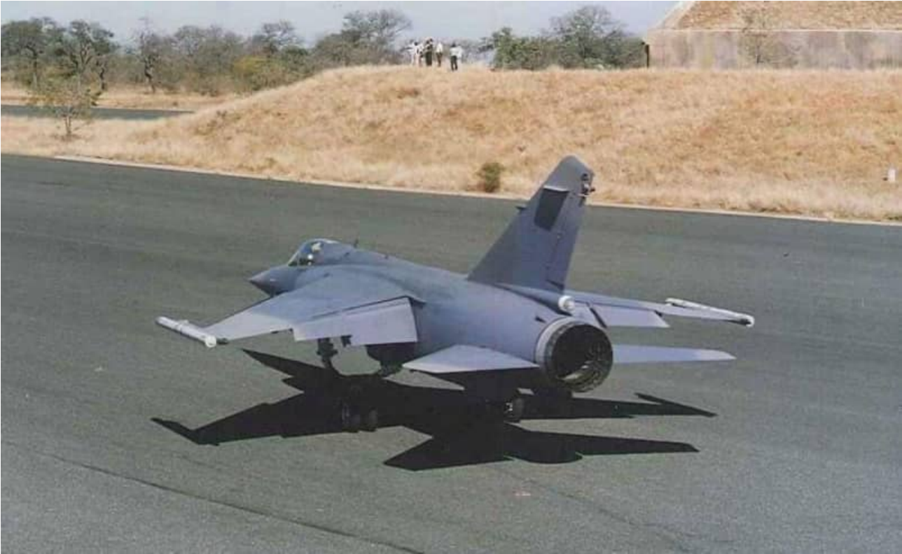
Two images of CZs in post-RWS and RIMS mod state. UHF antenna is now on the fuselage spine aft of the canopy.
