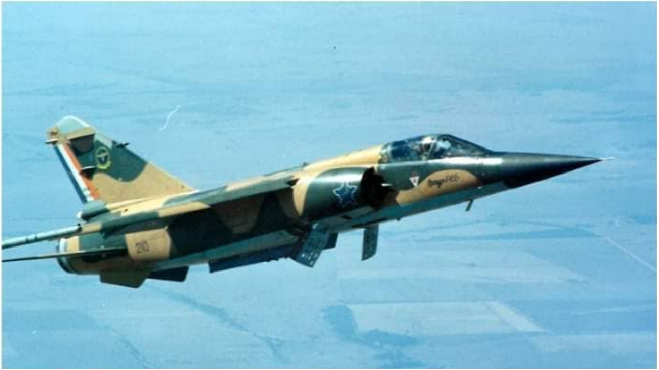
CZ #210 with what looks to be a practice captive R550 missile body on the starboard wing tip launcher – it has the black IR seeker head but no fins. Note that the antennas on the top of the vertical stabilizer are grey with white leading edges.
