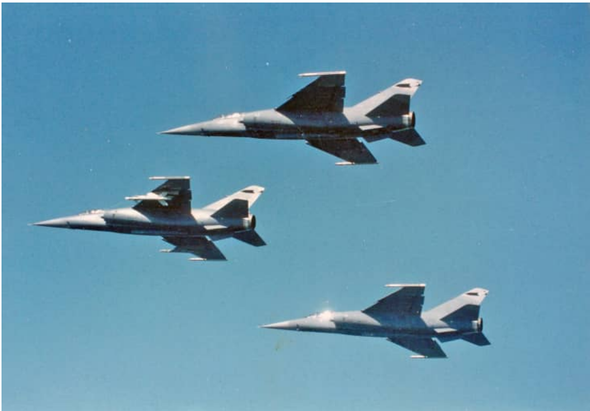
Three CZs in the final low visibility blue-grey camouflage scheme. The lead aircraft carries a single V35 missile beneath the port wing and an inert missile shape on the starboard wing.
