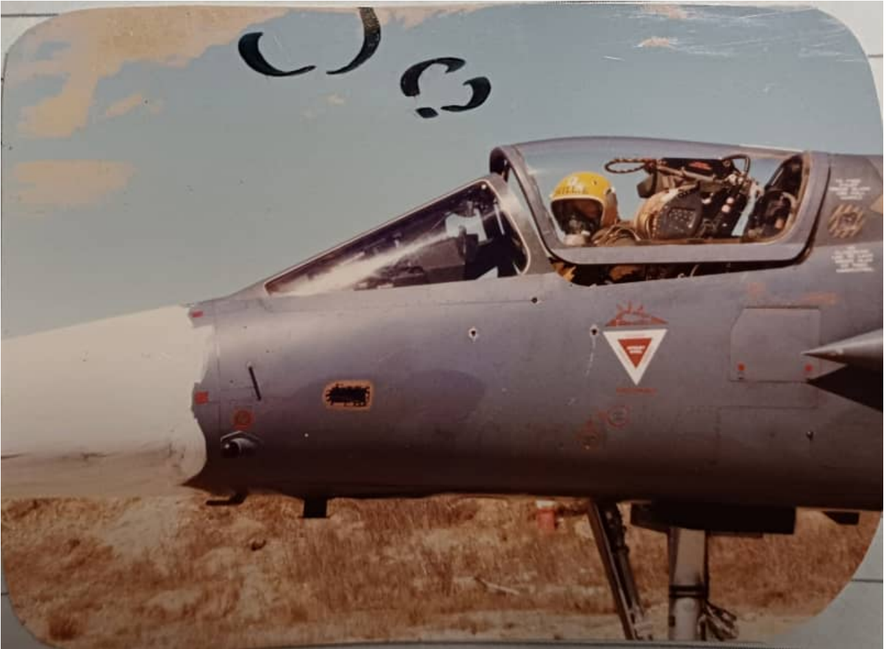
Early applications of the white noses as seen here on CZ # 209 were rather primitive. Later some CZs has their radomes more formally repainted in a matte white.
