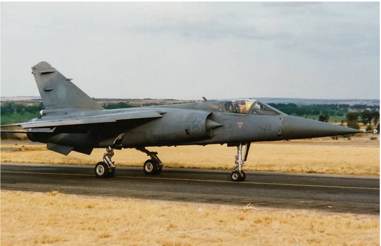
CZ #210 with prominent Castles on the intakes. The camouflage appears to be freshly applied. Both aircraft on the page have the RWS and RIMS ventral fins installed. The UHF blade antenna has been relocated to the spine aft of the cockpit. #205 below has had the 3 Squadron badge on the vertical stabilizer painted over. Note how variable the greys/blues appear in the two images – a product of light and photo processing. #205 below has a single medium grey painted nose cone.
