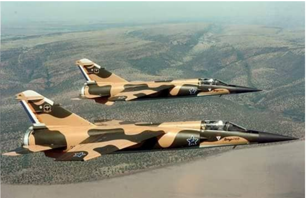
Two CZs look very clean and exceptionally elegant and are resplendent in full high visibility markings. The white circle on the vertical stabilizer is part of the original Dassault installed BF radar detection antenna suite. The pointed shapes on the vertical stabilizer leading and trailing edges are also part of this system. The dark object at the top rear of the vertical stabilizer is the red/clear navigation light. The blade antenna beneath the forward fuselage is the main UHF antenna. This was later relocated to the upper fuselage aft of the canopy when the upgraded RWS had been installed.
