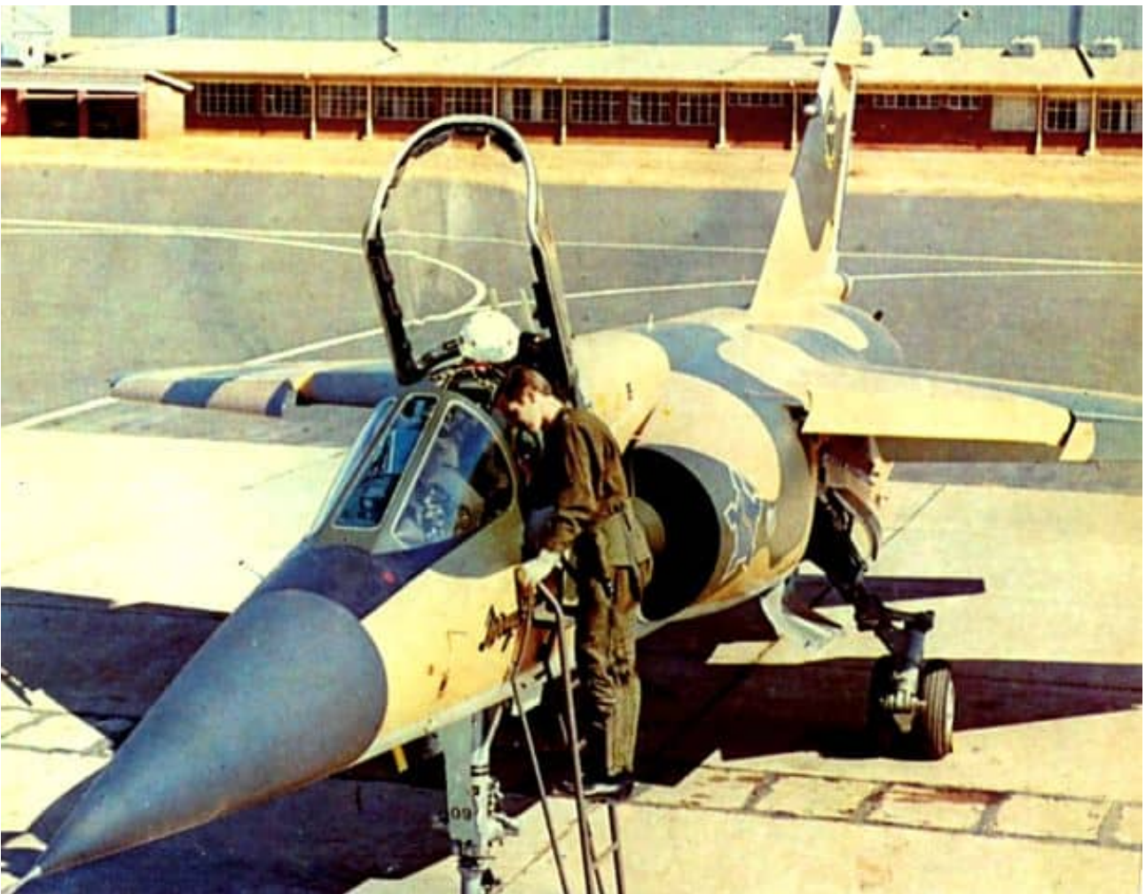
Of interest in this image is the dull grey colour of the radome whereas the rest of the aircraft looks very clean and unweathered in the original camouflage scheme. The anti-glare panel is black. This is CZ #209 as can be seen by the small "09" digits on the nose gear door. Note how the outboard leading edge slats extend forwards whereas the inboard leading edge flaps droop down. Note also the yellow sealing trim around the windshield frames.
