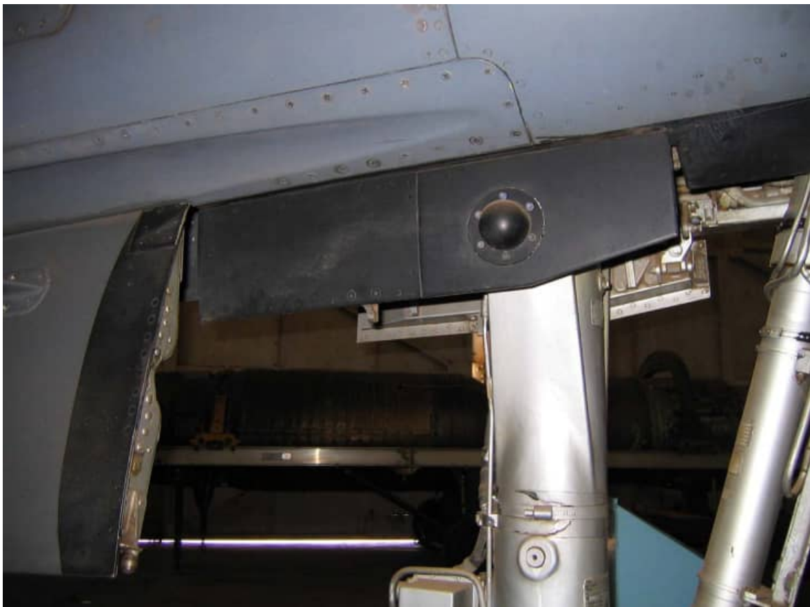
RWS button antenna on the right-hand forward nose gear door. Undercarriage legs (nose and main) are painted aluminium. The black painted area forms part of the "false" canopy marking on the underside of the forward fuselage as applied to CZs in the low visibility blue-grey camouflage.
