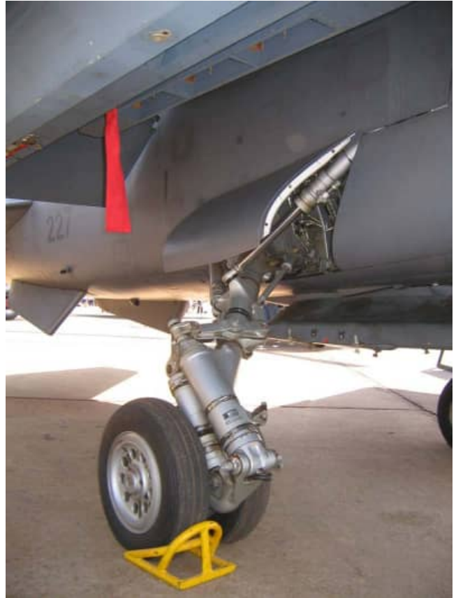
Main undercarriage compressed correctly imparting nose-up stance to the aircraft. Compare this to the images of the unloaded undercarriage of CZ #207 earlier in this document.
