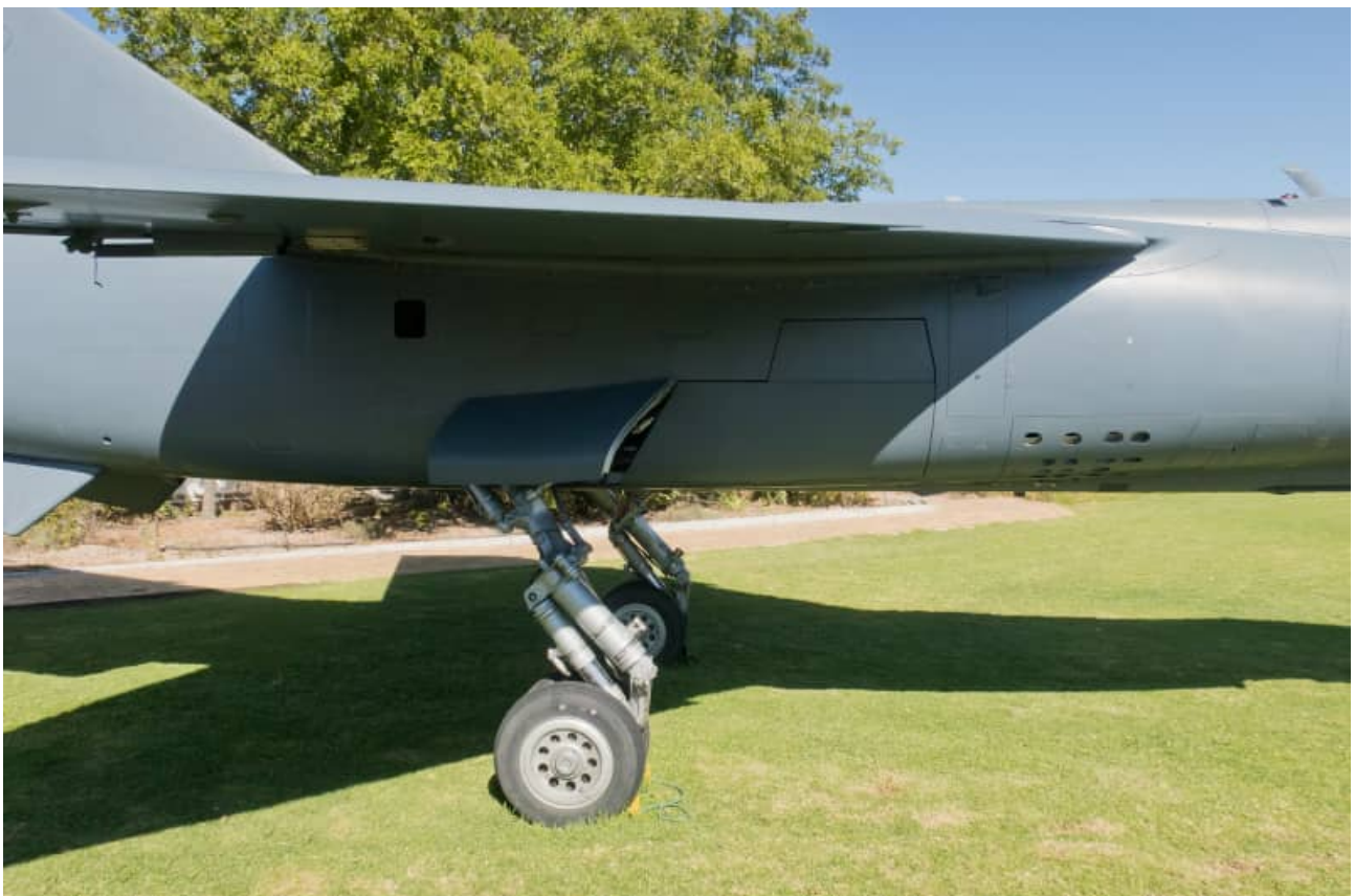
Note the unloaded tail up "stance" of the aircraft without the engine fitted.
