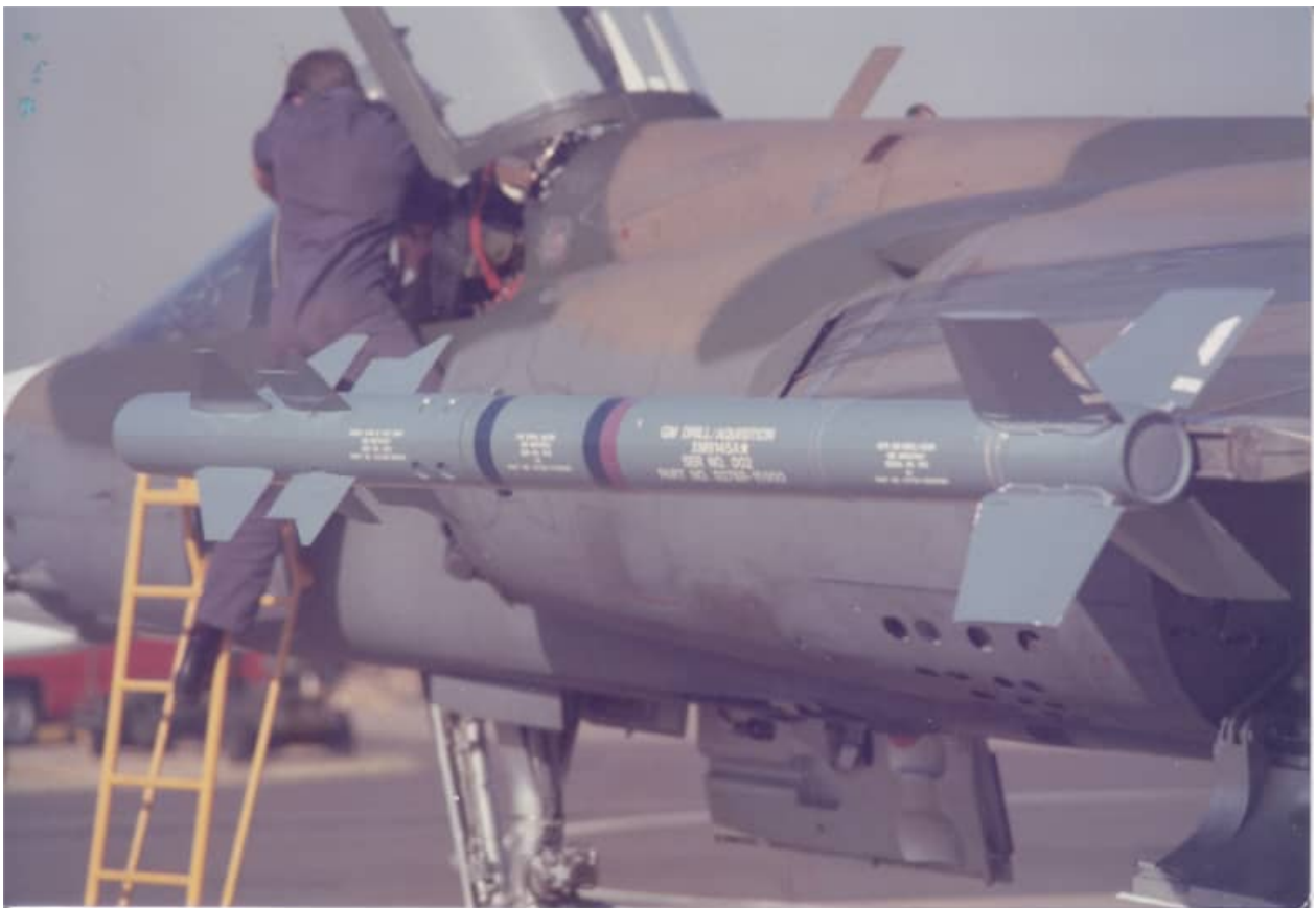
The V3C was identical to the R550 in appearance. The main visual difference between the two are the large "eyes" of the laser proximity fuse present on V3C, 2 just aft of each of the rear canards.
