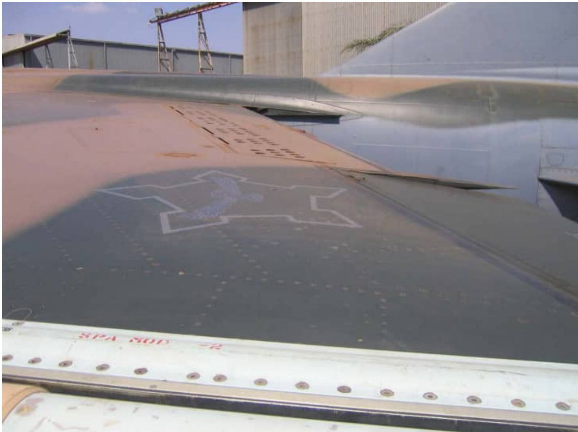
SAF Castle with Eagle on port upper wing. These did not appear on the lower wing surfaces for this colour scheme. Another detail to note is the dark grey no walk stripe ahead of the ailerons.
