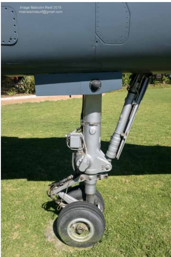
Note the asymmetric arrangement of hydraulic tubes on the sides of the nose gear retraction piston.
