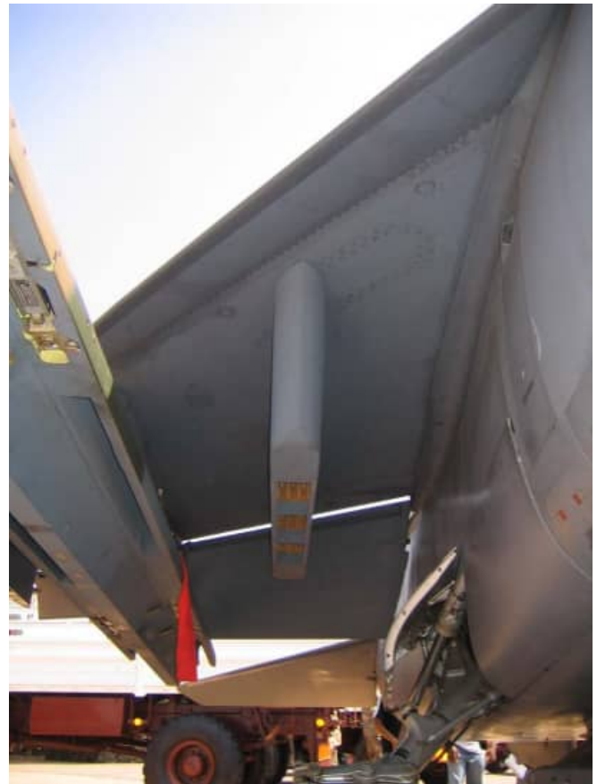
Details of the wing mounted CLB8 / A26 4-bomb carrier with the staggered arrangement of bomb shackles. The slots aft of the bomb shackles are for the bomb fins, indicating that these were carried in a cruciform arrangement (hence the staggered arrangement) unlike those on the centerline which were carried such that the fins were in a diagonal arrangement. #227 as it appears in these images, represents the 14-bomb configuration (typically 14 x 125kg Mk. 81 bombs, including one each on the outboard pylons). Range in this configuration would have been limited. The inboard RIMS chaff / flare dispenser is seen in the image on the right located on Station "0". It is unlikely that these were used by the SAAF on combat operations.
