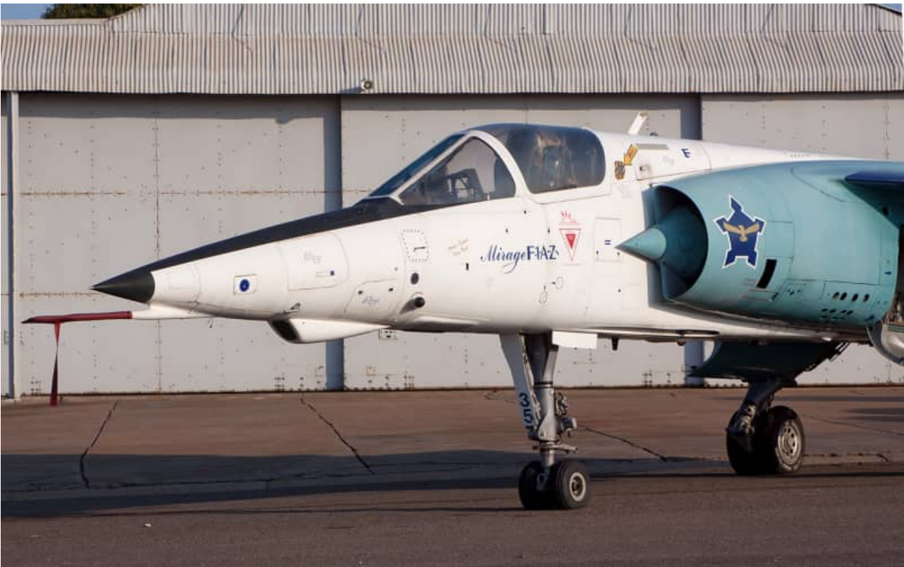
Details of AZ nose. The profile is different to that of the CZ radar nose. The fairing for the laser designator can be clearly seen on the underside of the nose. The access panel details on the AZ nose do not appear on the CZ's radar nose. #235 has the later Castle with golden SAAF Eagle applied.
