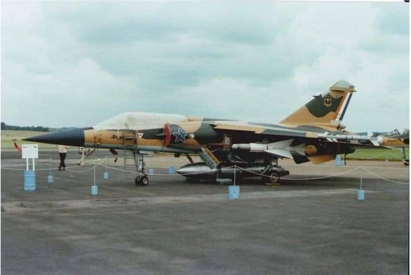
CZ #212 on airshow display duty with two R530s on the inboard wing stations and two R550s on the wingtip stations. It carries a centerline RP35 1,200 liter fuel tank. The R530 was not used by the SAAF in combat operations.
