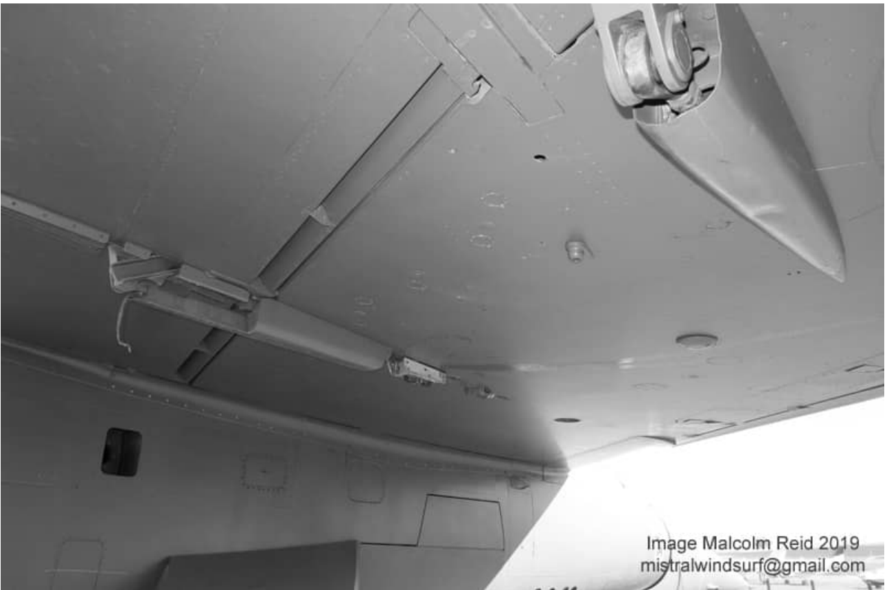
Flap actuators. The aerodynamic cover on the inboard one is missing.
