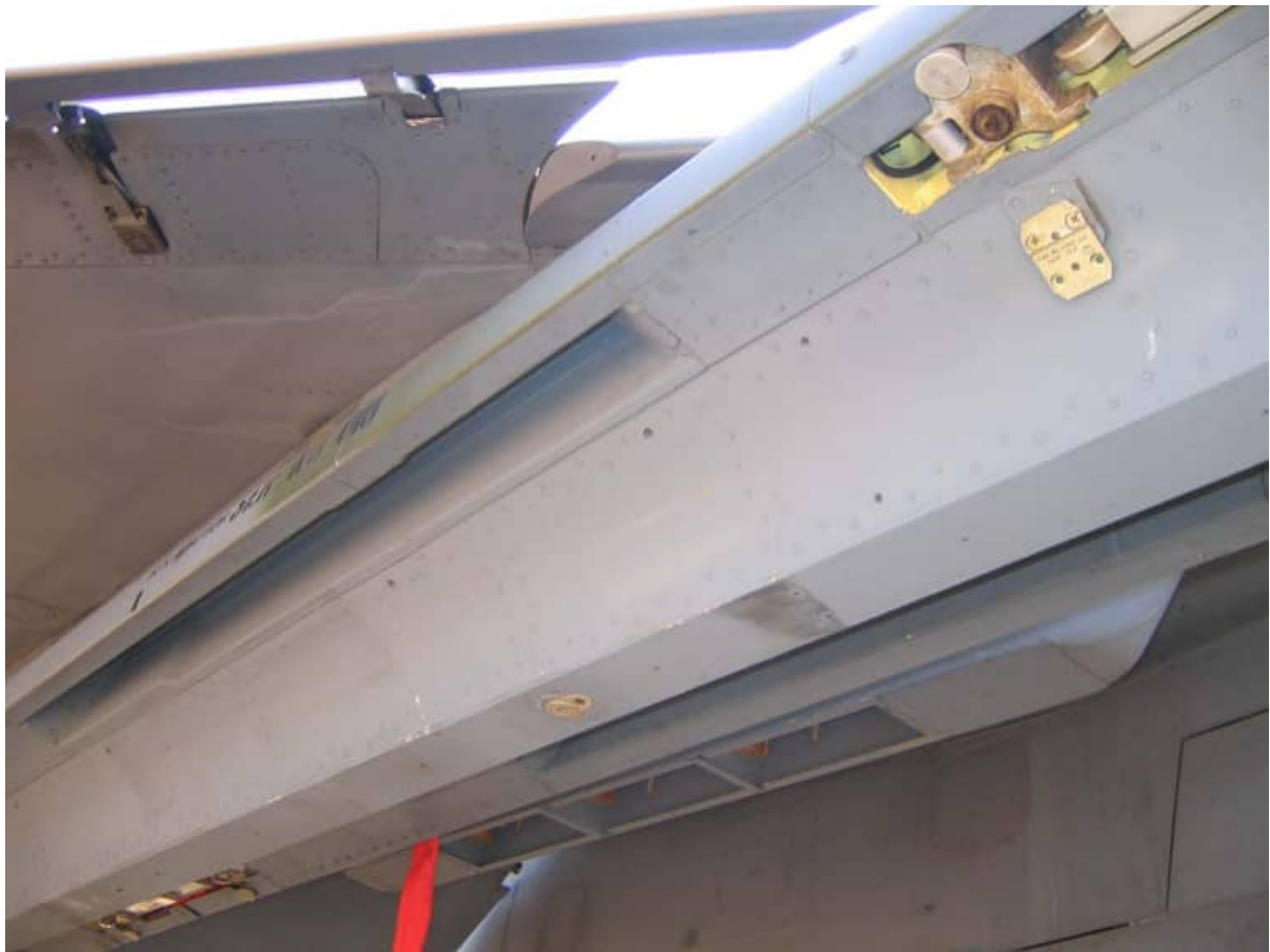
Details of wing CLB8 / A26 4-bomb carrier. Recesses are for the bomb fins. Note the RIMS dispenser pod behind this with three empty bays for the chaff / flare cartridges. These dispensers appear to be wider than those fitted into the ventral fins.
