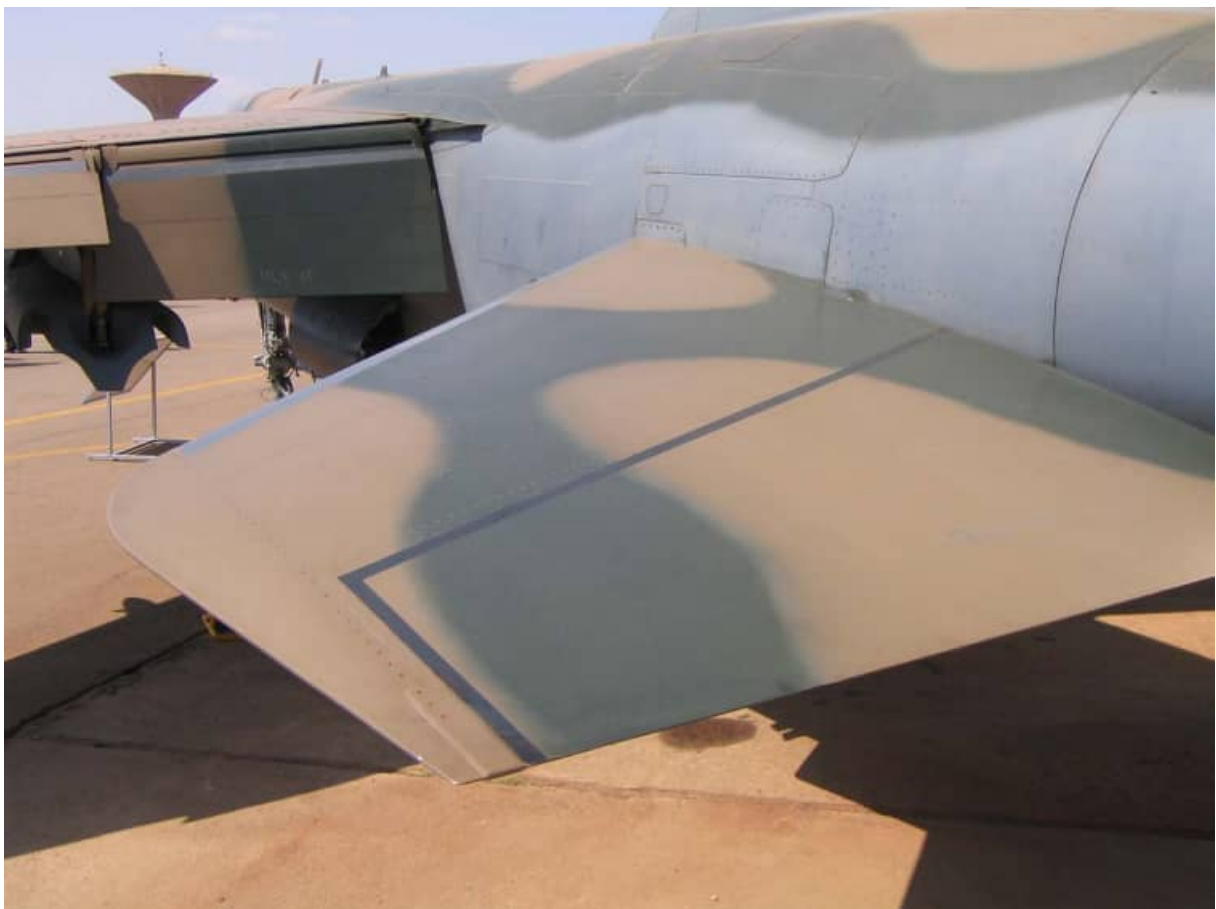
Characteristic nose up attitude of the horizontal stabilizers when the F1 is at rest. Note the grey leading edge as well as black walkway markings. The drag chute cone is missing. The port side afterburner cooling intake is visible ahead of the exhaust.
