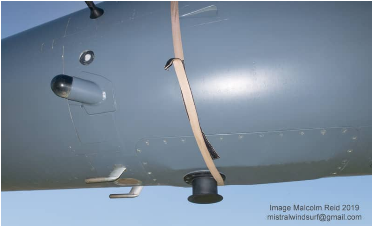
Visible are the dual pitot probes and the black cylindrical and spherical RWS antennas. Note the shape of panel onto which the cylindrical RWS antenna has been located. This panel appears to be of a different arrangement to that originally fitted to the F1s. This necessitated the relocation of the UHF blade antenna from this position to the fuselage spine aft of the canopy. The black cylindrical antenna is for directional / azimuth data for the RWS and was installed only on the CZ and not the AZ. The back object at the top left of the image is a protective cover over the incidence probe.
