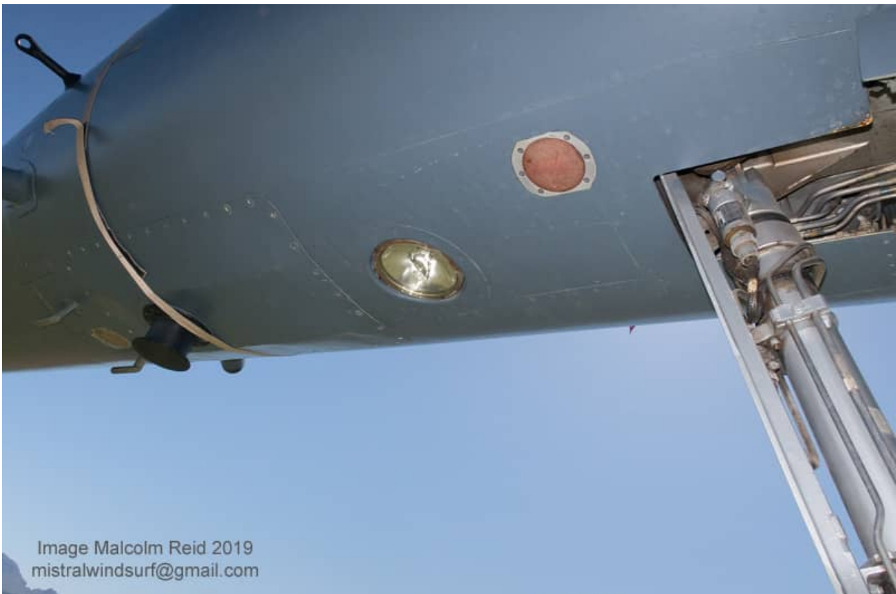
Landing light – this drops down during landing and takeoff. The red object is the radar altimeter antenna.
