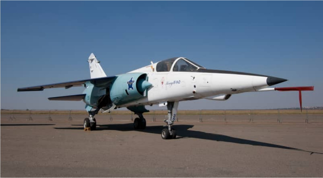
Details of AZ nose. The profile is different to that of the CZ radar nose. The fairing for the laser designator can be clearly seen on the underside of the nose. The access panel details on the AZ nose do not appear on the CZ's radar nose. #235 has the later Castle with golden SAAF Eagle applied.
