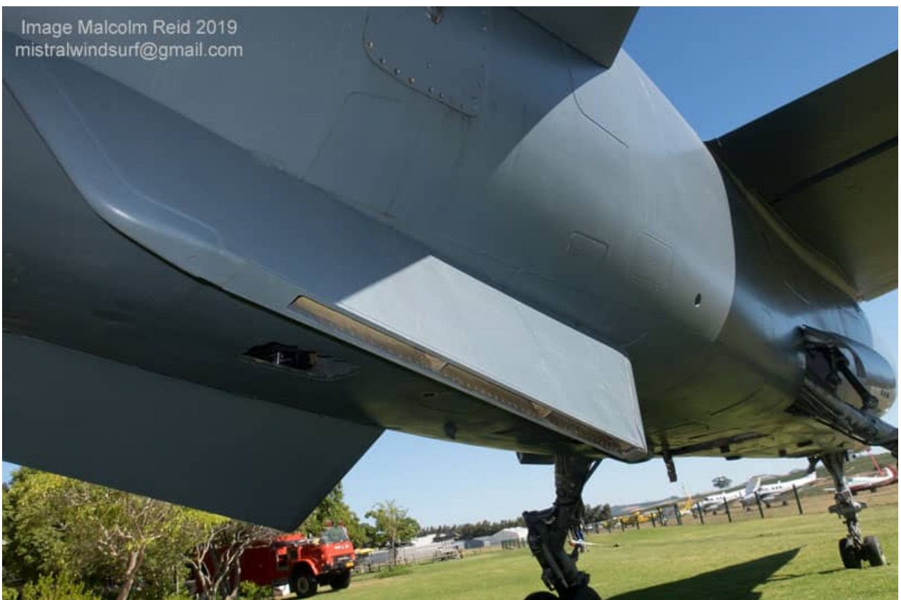
Details of the locally produced ventral fin with integral RIMS chaff/flare cartridges. These replaced the original Dassault ventral fins and were installed on both the AZ and CZ fleet. The three empty bays for the RIMS cartridges can be seen in the image below.
