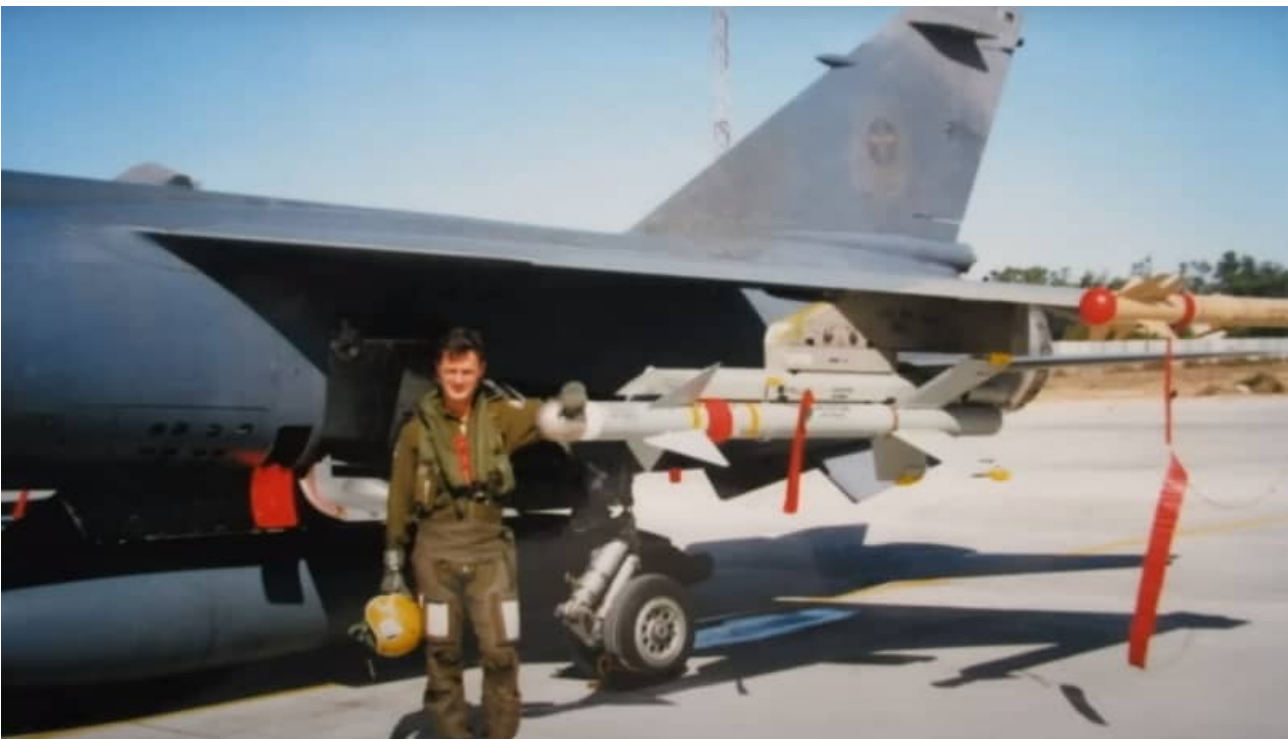
Two images of CZs carrying V35 missiles on the outboard wing pylons. Notice how the V35 launch rail interfaces to the standard Station 2 pylon through and adaptor. The aircraft above is carrying an R550 missile on the wingtip station, whereas the aircraft below carries a V3B in this location.
