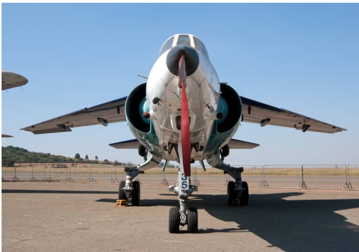
The location of the two forward facing RWS antennas can be clearly seen in this image. The clear window for the laser range finder can be seen beneath the nose.
