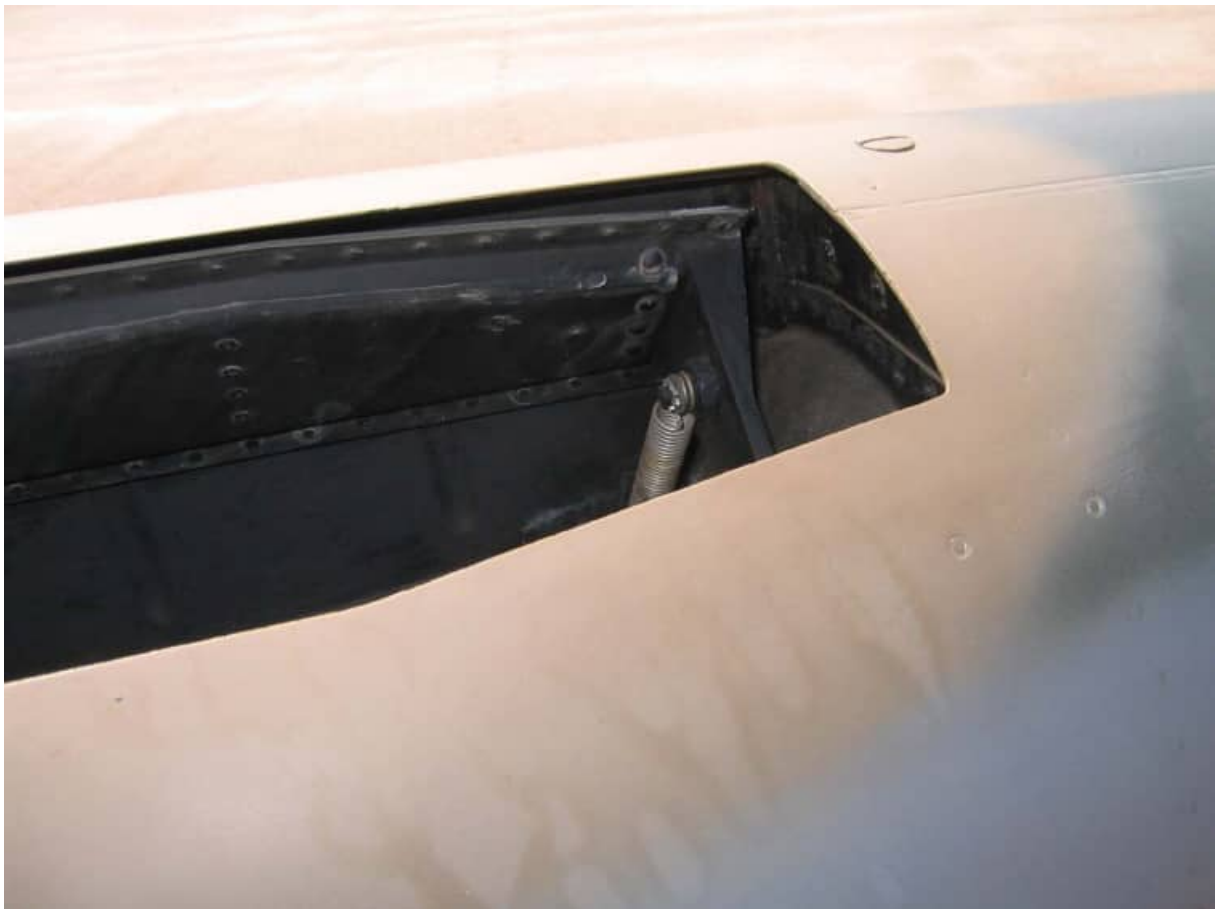
Details of the retractable refueling probe bay which is offset to starboard on the AZ nose. The bay aft cover is fixed to the probe itself. The forward bay door (to the right in the image above) rotates to the left.
