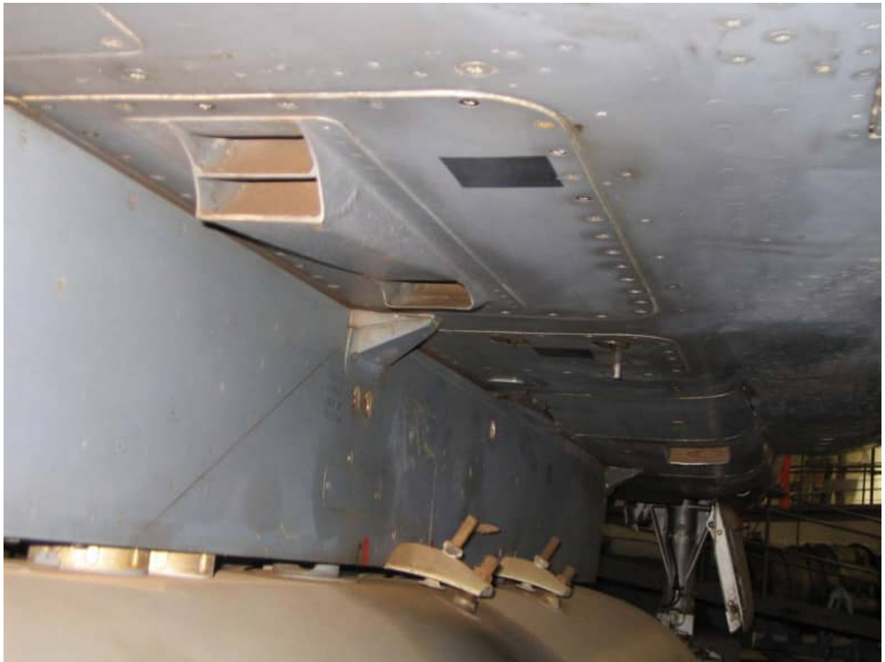
Details of underside vents, external fuel tank and pylon. Note the red edging to the various access panels – this to allow ground / flight crew to identify open panels easily prior to start-up.
