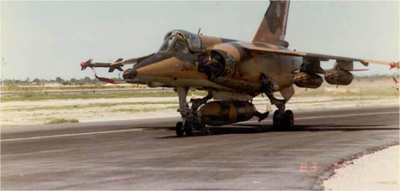
In this image dated from 1983, an AZ is taxiing out for a strike with four rocket pods. The port forward black RWS spiral antenna is visible above the nose landing gear leg. The RIMS ventral fins are not fitted – these are clearly of thinner section when compared to the later RIMS units.
