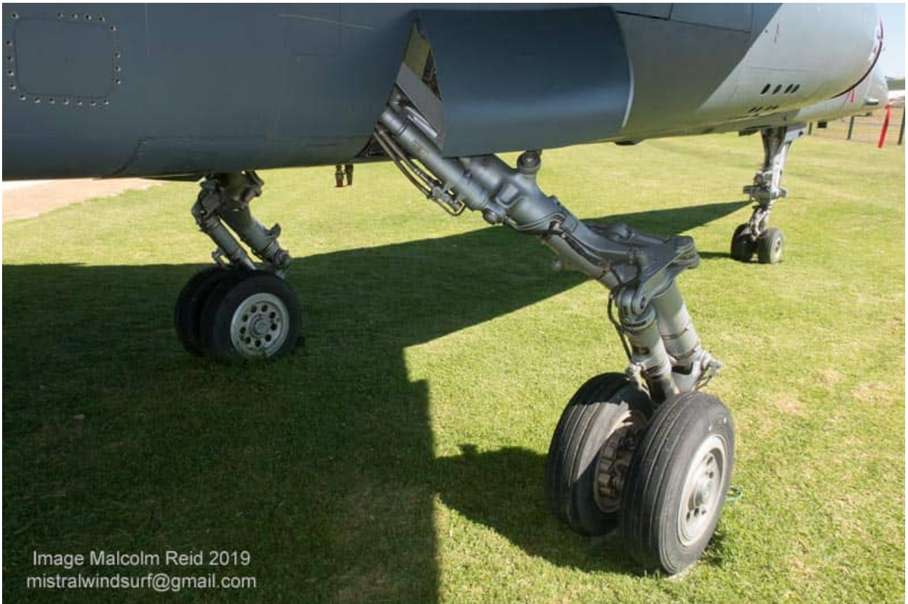
#207 does not have the engine installed. When fully loaded the F1 had a distinct nose up stance.
