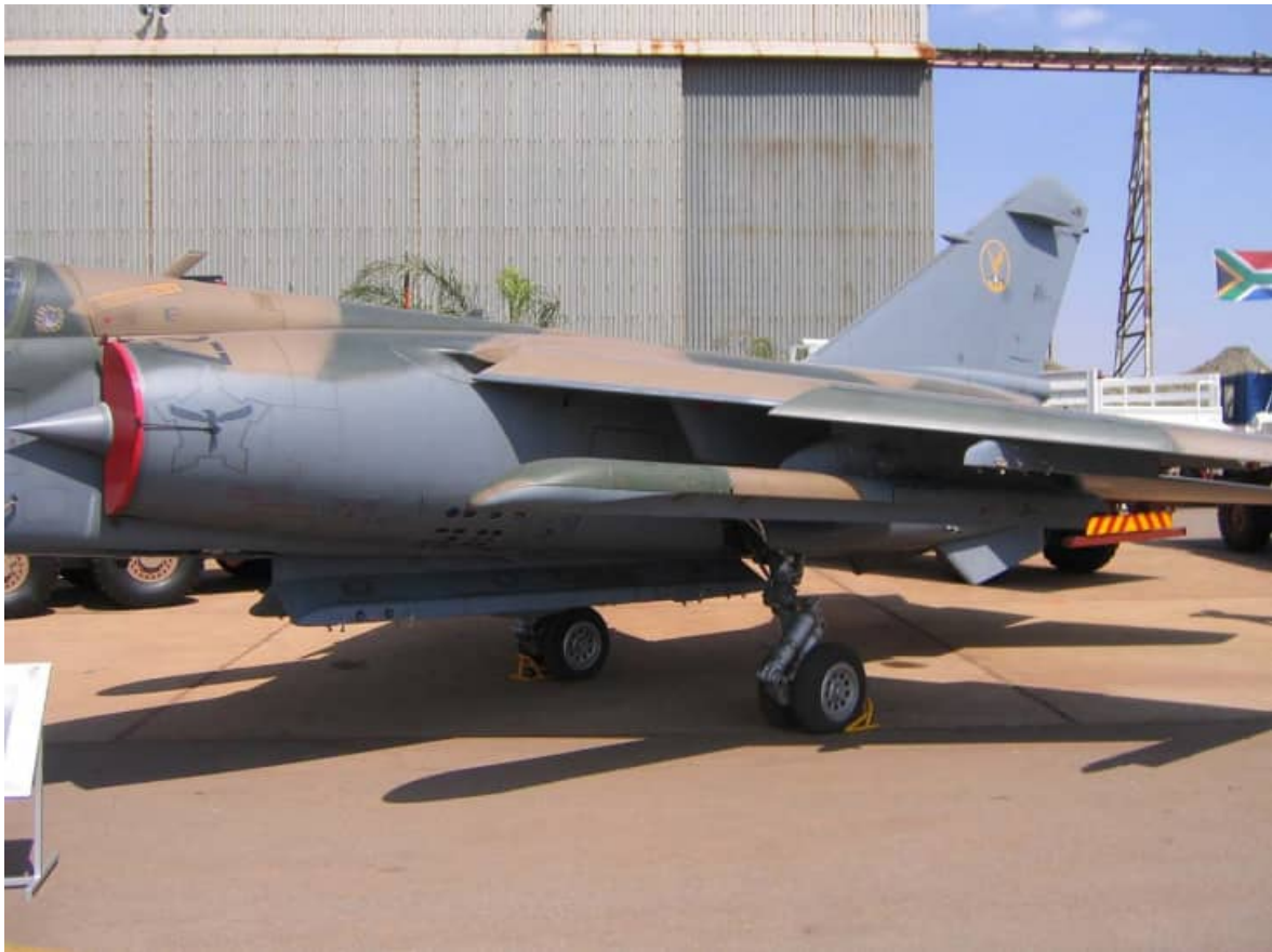
The front of the wing inboard leading-edge flap and the vertical stabilizer are painted in a darker grey. Note that outboard leading-edge slats are extended and inboard leading edge flaps are lowered. F16s would be seen variably at rest with flaps/slats extended/drooped or all retracted.
