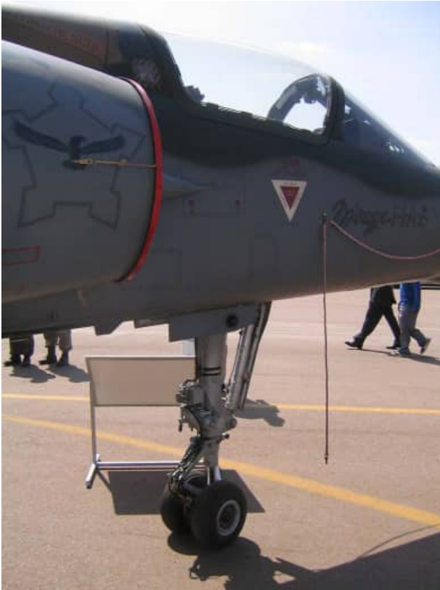
Main undercarriage compressed correctly imparting nose-up stance to the aircraft. Compare this to the images of the unloaded undercarriage of CZ #207 earlier in this document.
