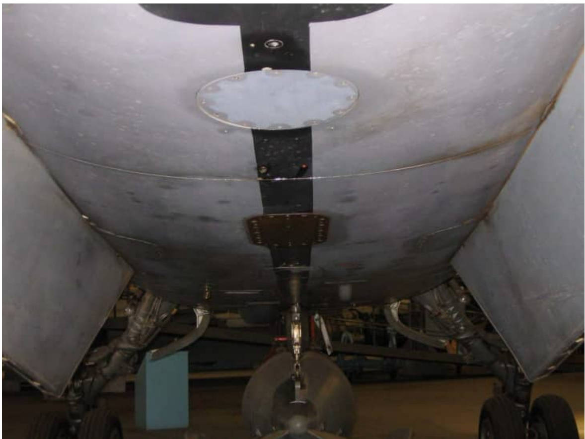
Rear underside view looking forward. The black stripe is the "false" vertical stabilizer painted to confuse the enemy in a close turning fight. This was only applied to the F1CZs painted in the three-tone blue/grey camouflage. Note the modified ventral fins which contain the RIMS chaff and flare dispensers.
