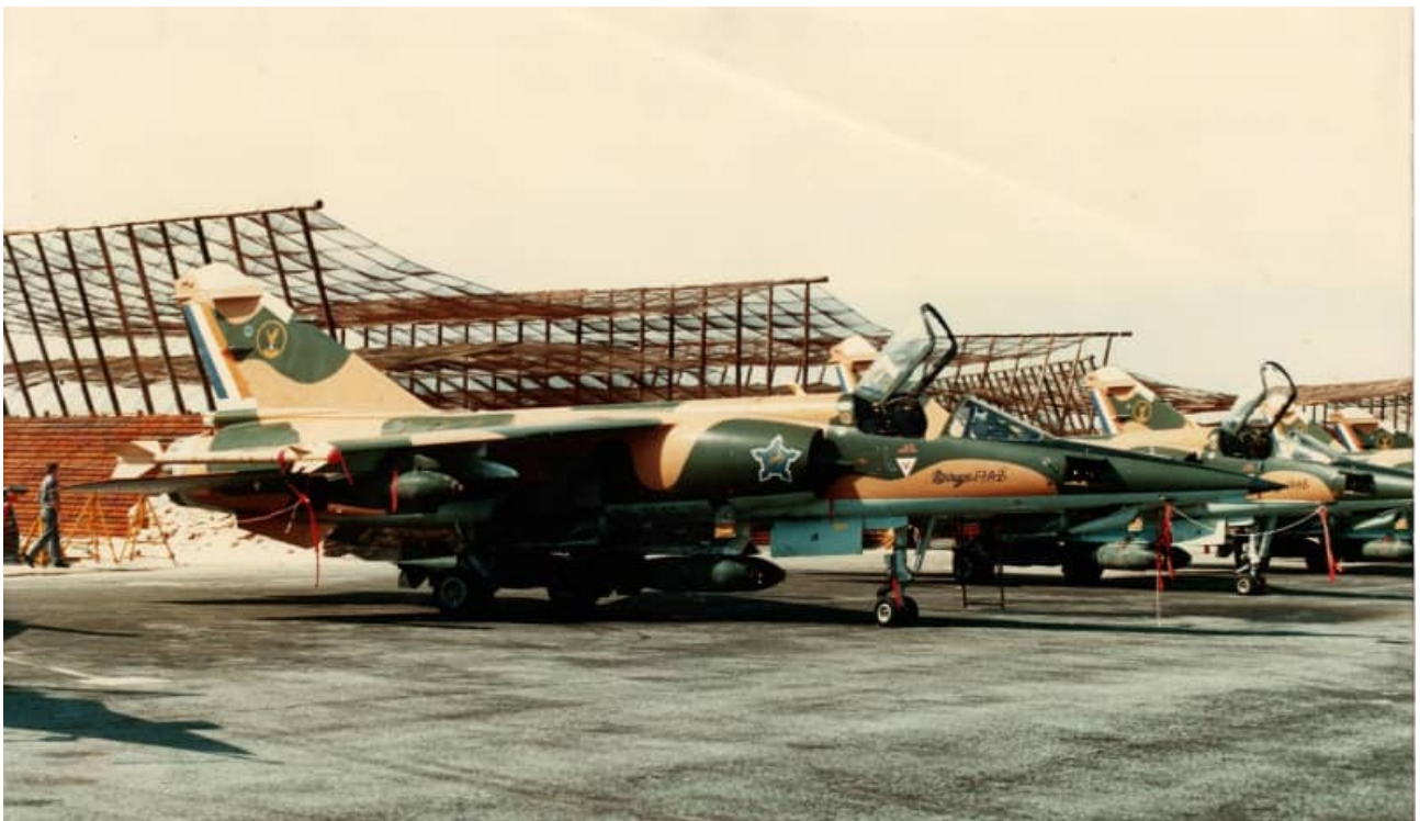
AZ with wingtip mounted V3B missiles. Note the different canard arrangements between the two as well as the more slender (high aspect ratio) tail fins of the R550.
