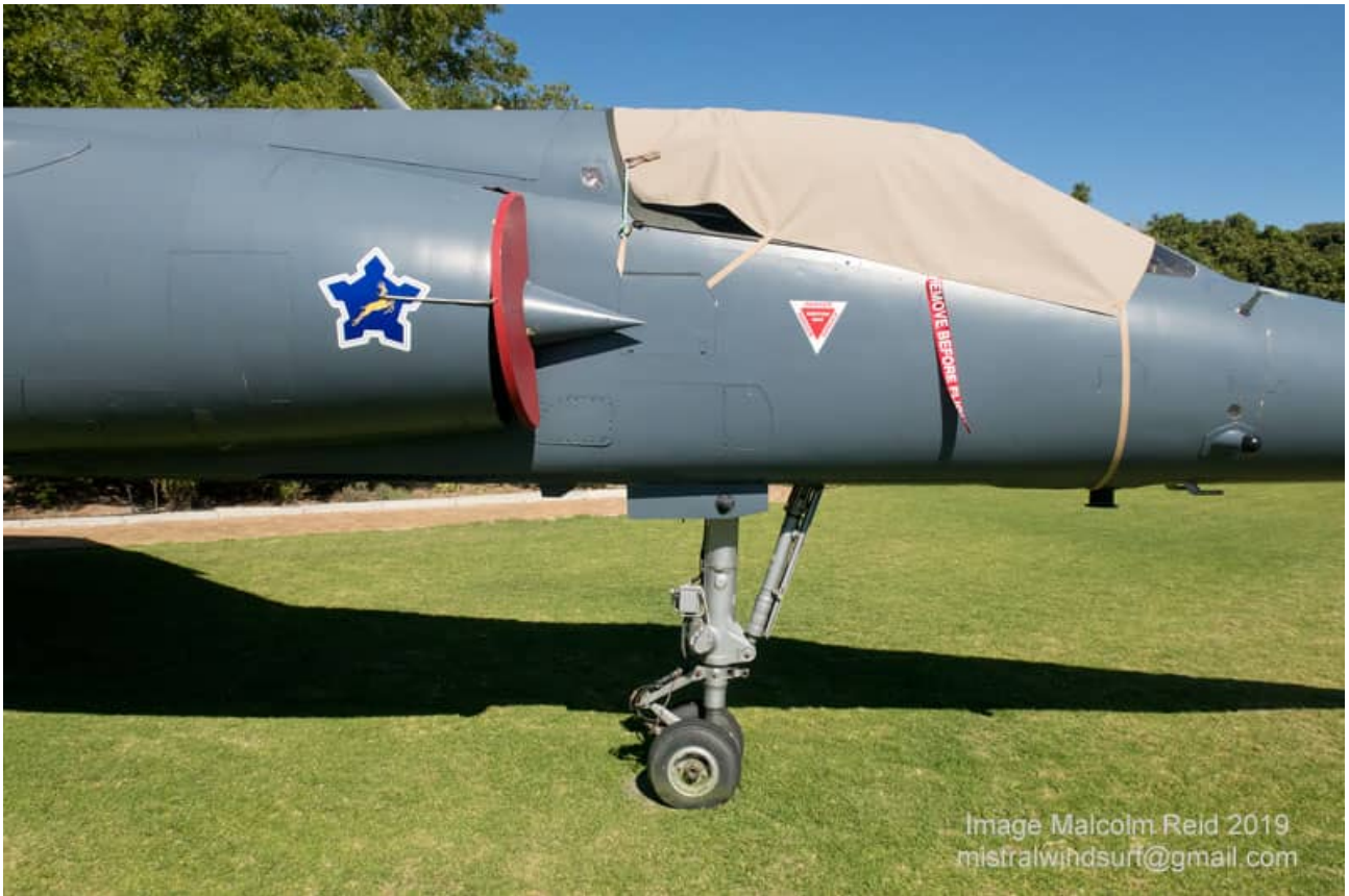
The SAAF Castle applied to #207 is totally inaccurate both in size and the width of the white border. Note the shape and length of the intake conical shock cone.
