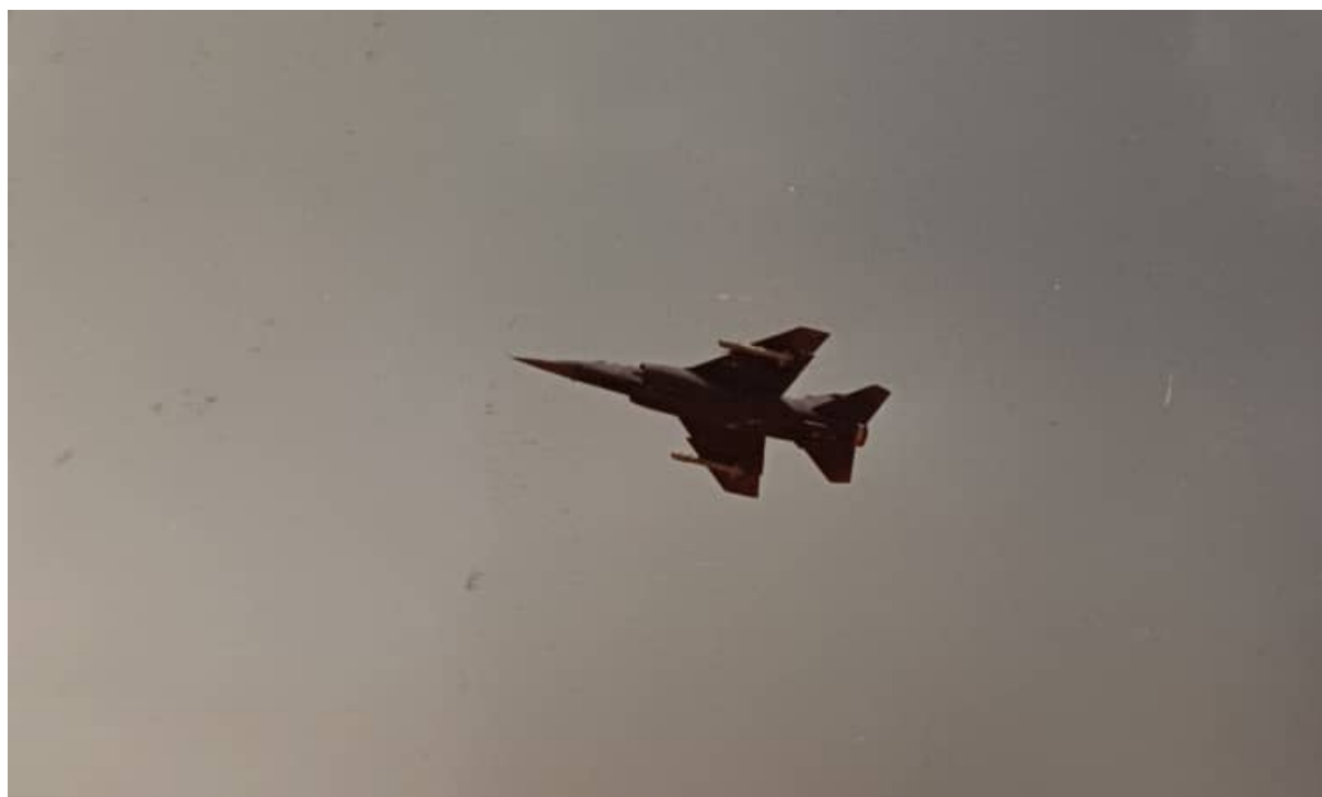
CZ tail number "205.5" (the forward fuselage of #205 mated with the rear fuselage of #206) over the Hammanskraal range in the early 1990s. It is equipped with two ACS pods – a rather atypical configuration on the CZ.
