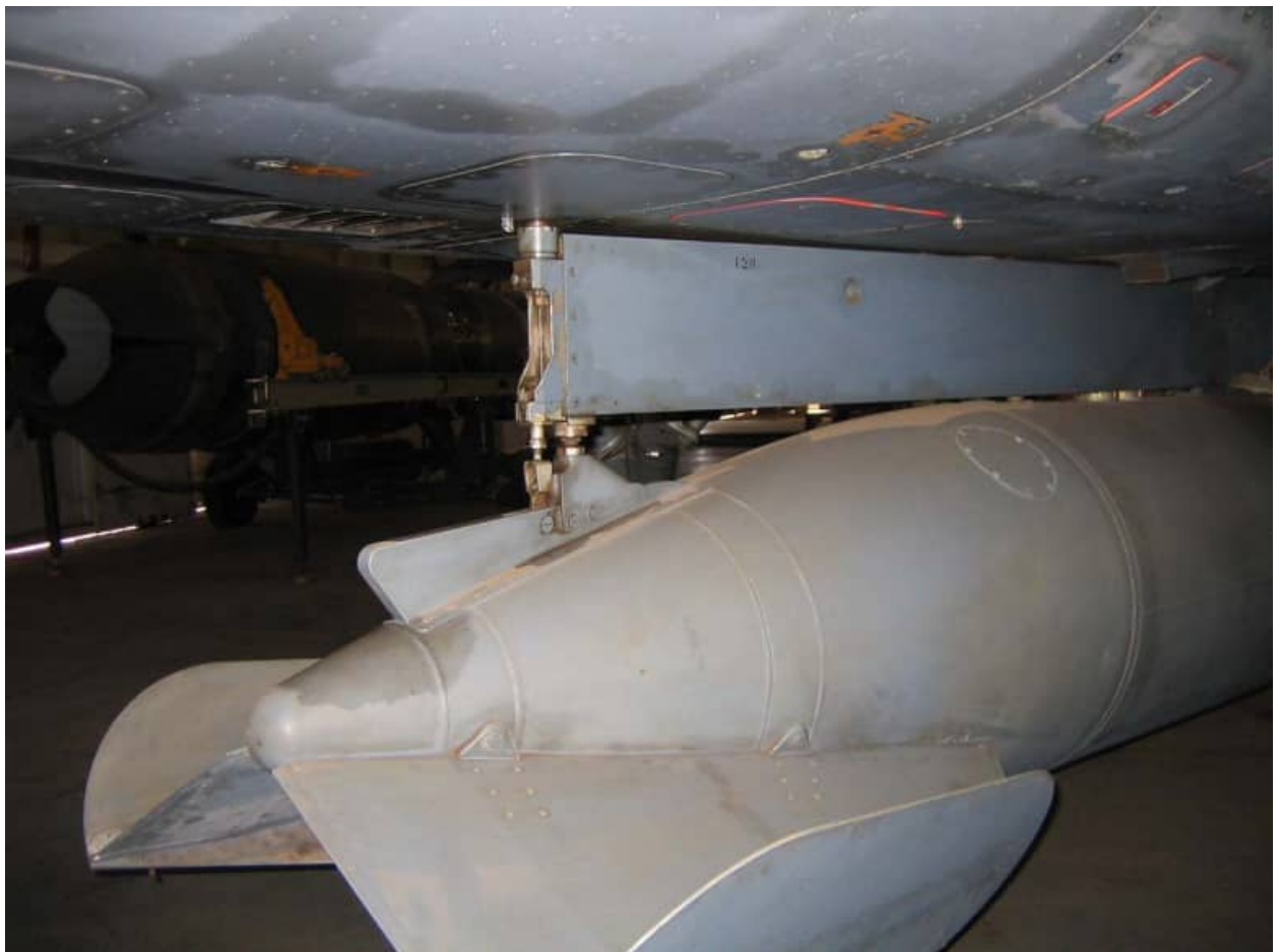
Details of underside vents, external fuel tank and pylon. Note the red edging to the various access panels – this to allow ground / flight crew to identify open panels easily prior to start-up.
