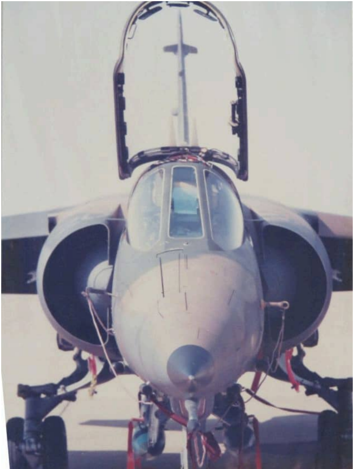
Head on photo of an AZ. Note the offset location of the refueling probe on the upper nose and the small black ranging radar.
