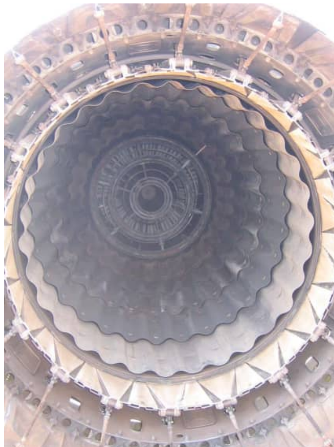
Atar 09K50 engine afterburner and exhaust nozzle details.
