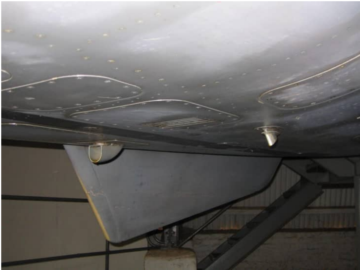
203 is equipped with the locally produced ventral fin with integral RIMS chaff/flare cartridges. The shape is more angular than the original French supplied units. The actual fin is also a lot wider to accommodate the cartridges.
