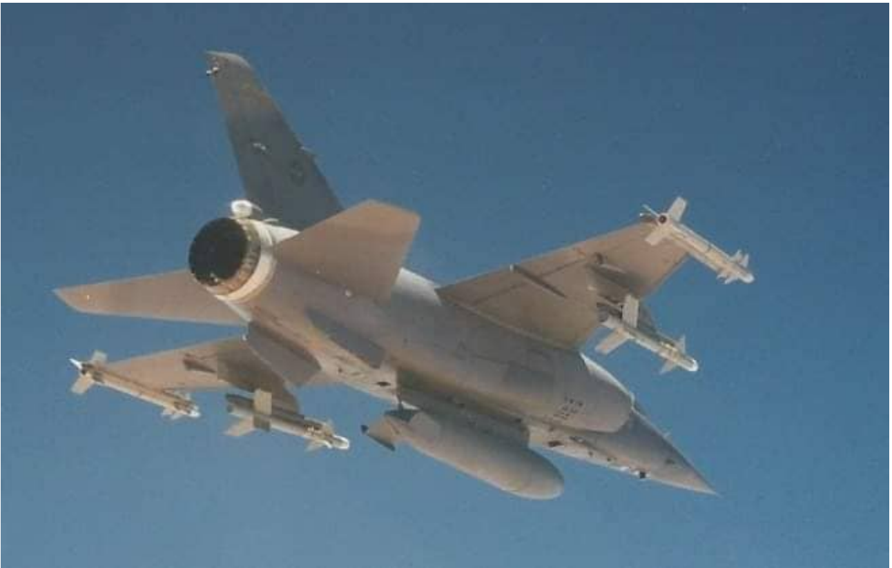
Post combat operations image of a CZ showing the RIMS and RWS installation. Note the two black antennas at top of the vertical stabilizer and cylindrical CD/DF antenna beneath the nose. The black button antenna on the nose gear door as well as the starboard forward-facing antenna are also just visible. The RIMS chaff/flare cassettes are visible in the ventral fins.
