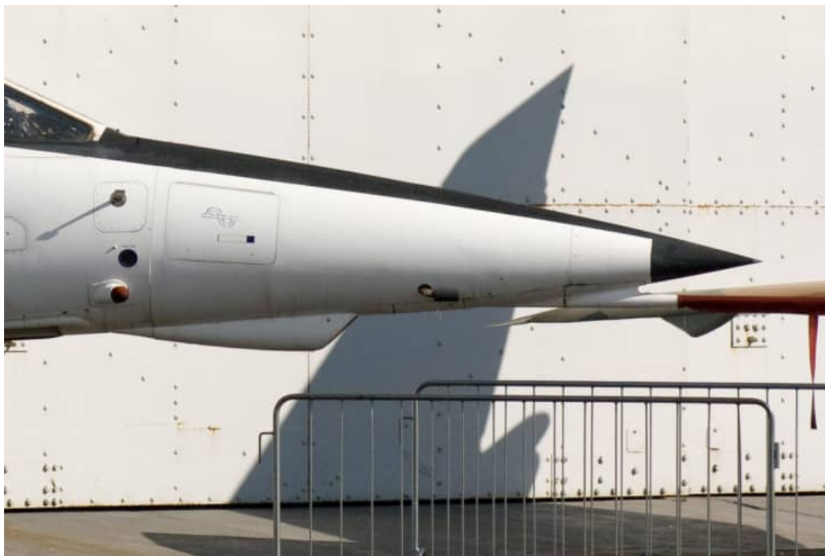
AZ nose profile. Note the small black ranging radar and the laser designator beneath the nose. There are also access panels both sides of the AZ nose. The pitot probe is located beneath the ranging radar.
