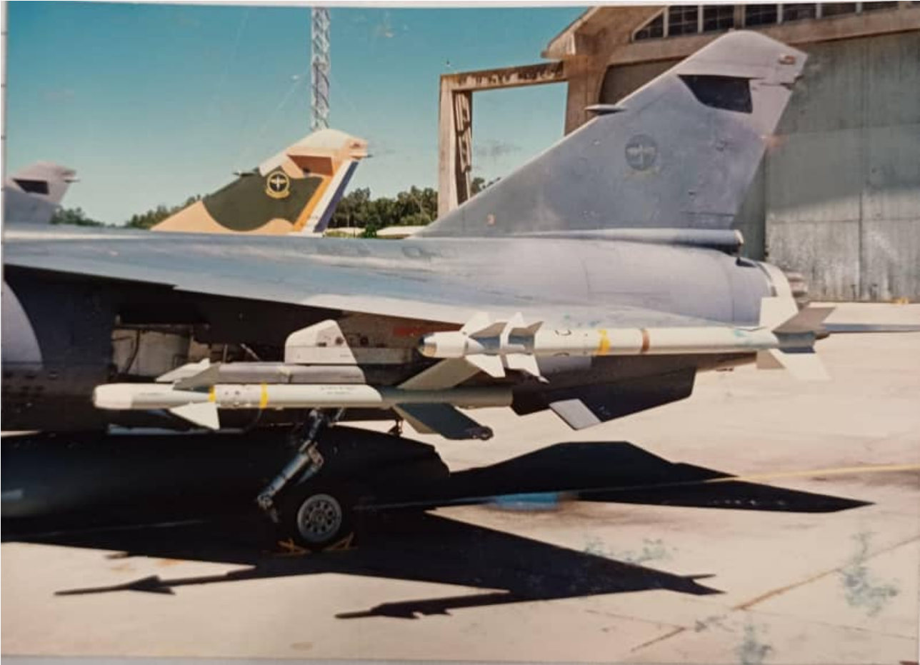
Two images of CZs carrying V35 missiles on the outboard wing pylons. Notice how the V35 launch rail interfaces to the standard Station 2 pylon through and adaptor. The aircraft above is carrying an R550 missile on the wingtip station, whereas the aircraft below carries a V3B in this location.
