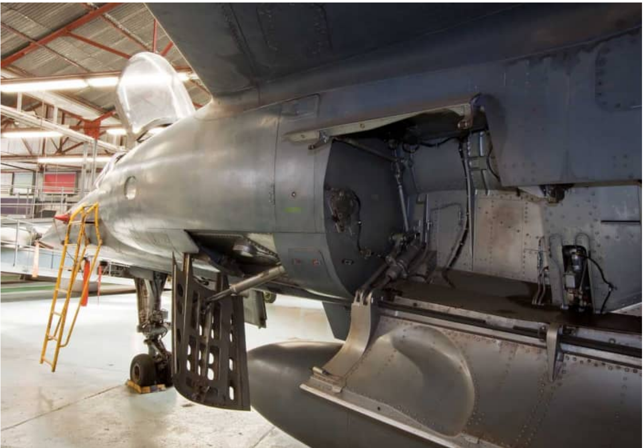
The F1CZ had a spotlight for night intercepts on the forward port intake. The AZ did not. The interior of undercarriage and airbrake bays were bare aluminum. Note the structural details of the airbrake.
