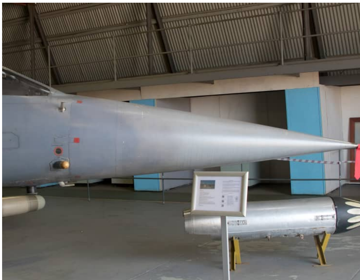
CZ nose profile. The nose shape is more symmetrically conical to house the Cyrano IV radar. There are no access panels. The pitot probe extends from the tip of the nose.
