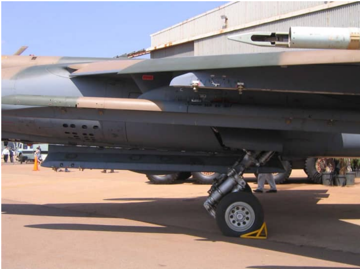
The SAAF used the centerline CLB4 4-bomb carrier in combat (on both the AZ and CZ). Note the difference in longitudinal angle between the fuselage and the CLB4 which is angled down towards the front.
