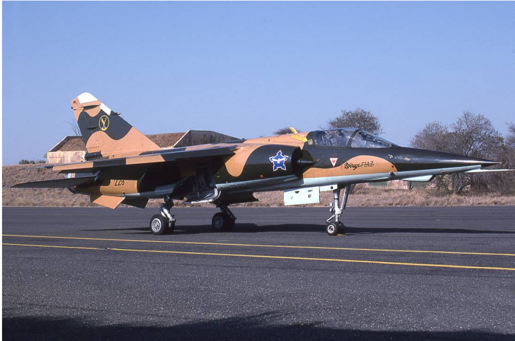
AZ #229 showing both RIMS and RWS installation. Note the two black antennas at top of the vertical stabilizer and the starboard forward-facing antenna on the nose. are also just visible. The black button antenna is visible on the small nose gear door and the black blade antenna is visible on the larger nose gear door. The ventral fins have a more defined angular plan view compared to the original fins (which had more rounded corners).
