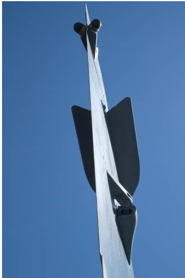
RWS antennas on the vertical stabilizer. The two horizontal blade antennas are for the VOR/ILS system. The rudder actuator is present on the starboard side.
