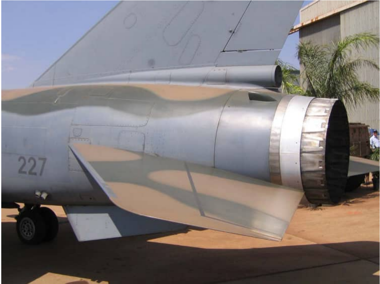
Characteristic nose up attitude of the horizontal stabilizers when the F1 is at rest. Note the grey leading edge as well as black walkway markings. The drag chute cone is missing. The port side afterburner cooling intake is visible ahead of the exhaust.
