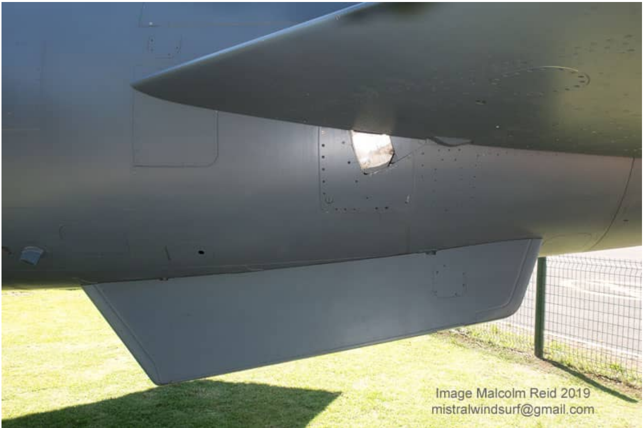
Details of the locally produced ventral fin with integral RIMS chaff/flare cartridges. These replaced the original Dassault ventral fins and were installed on both the AZ and CZ fleet. The three empty bays for the RIMS cartridges can be seen in the image below.
