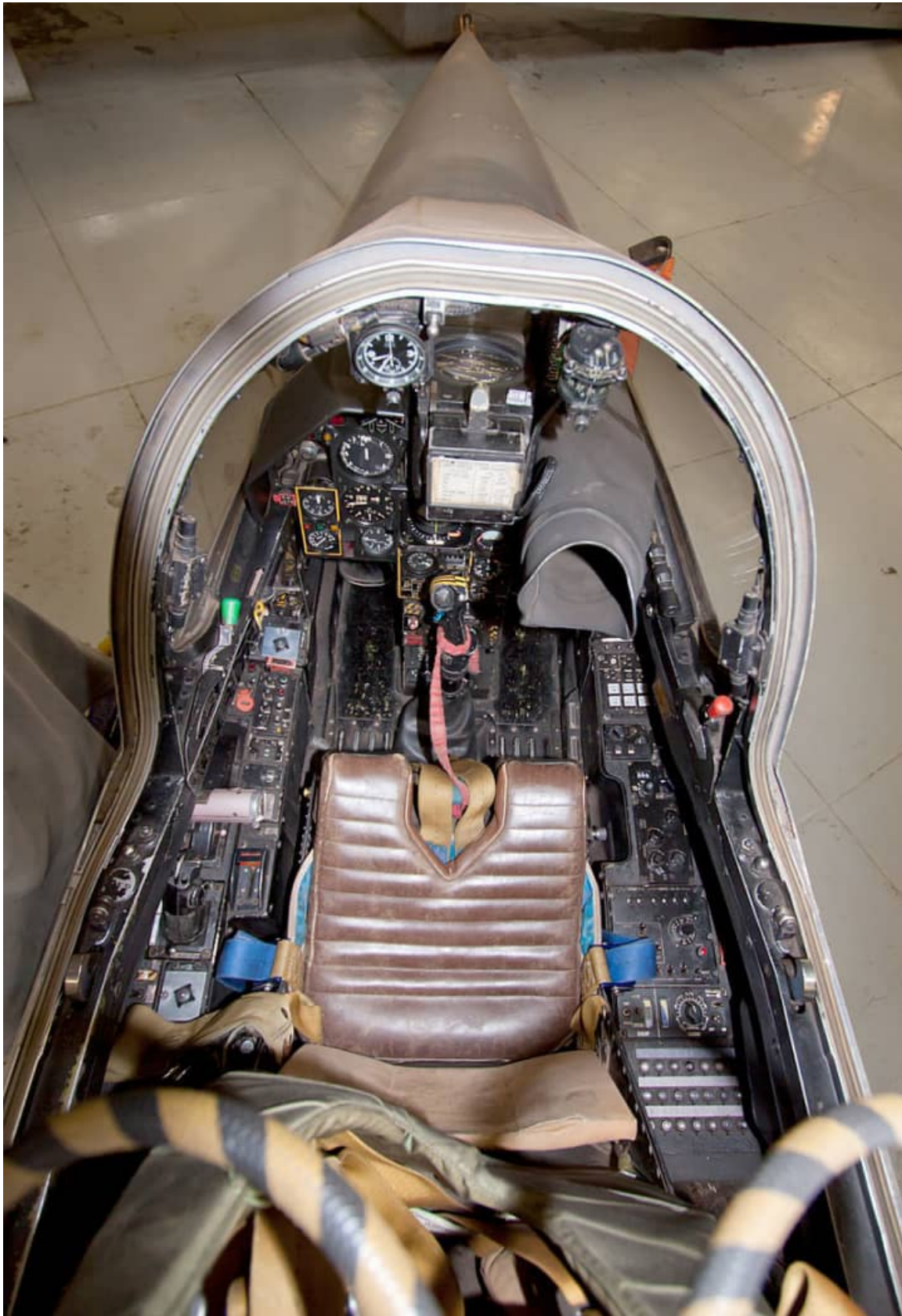
CZ #203 cockpit with MB.Mk.4 ejection seat and the distinctive shroud over the Cyrano radar display unit on the upper right of the instrument panel.
