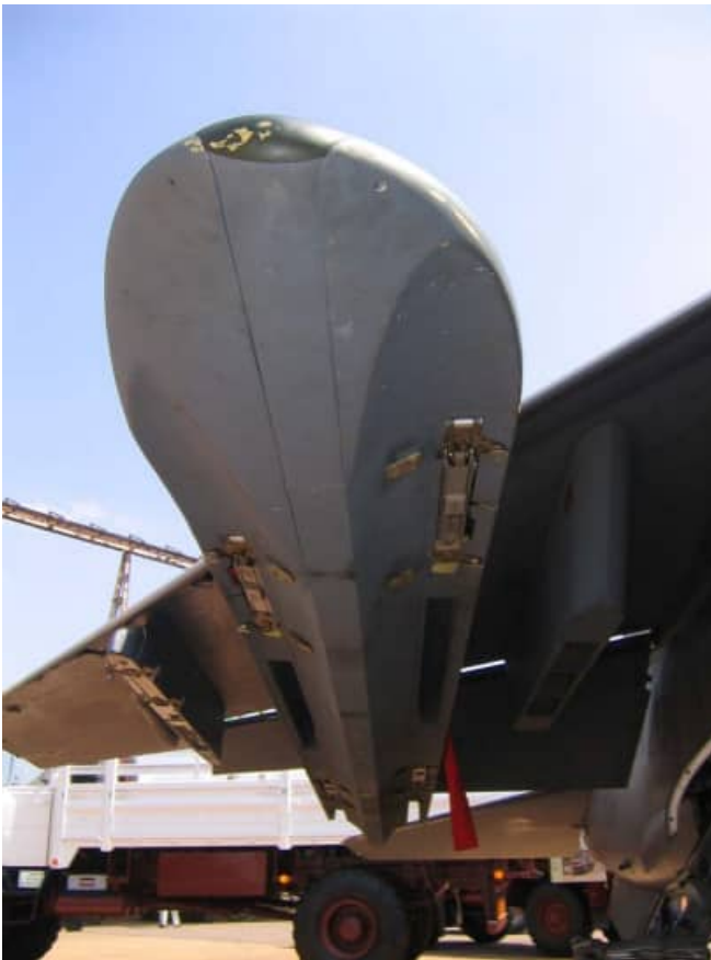
Details of the wing mounted CLB8 / A26 4-bomb carrier with the staggered arrangement of bomb shackles. The slots aft of the bomb shackles are for the bomb fins, indicating that these were carried in a cruciform arrangement (hence the staggered arrangement) unlike those on the centerline which were carried such that the fins were in a diagonal arrangement. #227 as it appears in these images, represents the 14-bomb configuration (typically 14 x 125kg Mk. 81 bombs, including one each on the outboard pylons). Range in this configuration would have been limited. The inboard RIMS chaff / flare dispenser is seen in the image on the right located on Station "0". It is unlikely that these were used by the SAAF on combat operations.
