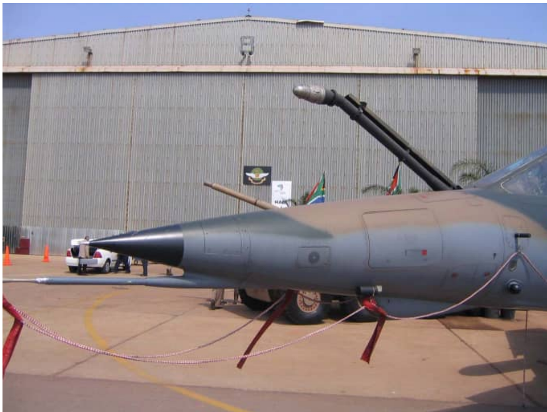
AZ nose panel detail with the refueling probe in the extended position.
