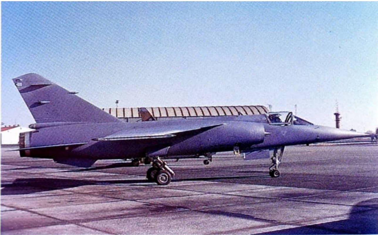
CZ tail number 203 is seen here in August 1984. The relocated UHF antenna is visible aft of the canopy on the upper fuselage, the CD/DF antenna on the underside of the nose and the spiral antennas replacing the rear facing BF RWR antenna on the upper vertical stabilizer trailing edge can also be seen. (Photo: Dave Becker)
