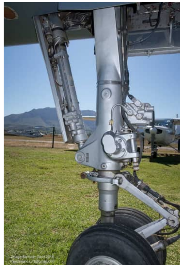
Note the asymmetric arrangement of hydraulic tubes on the sides of the nose gear retraction piston.
