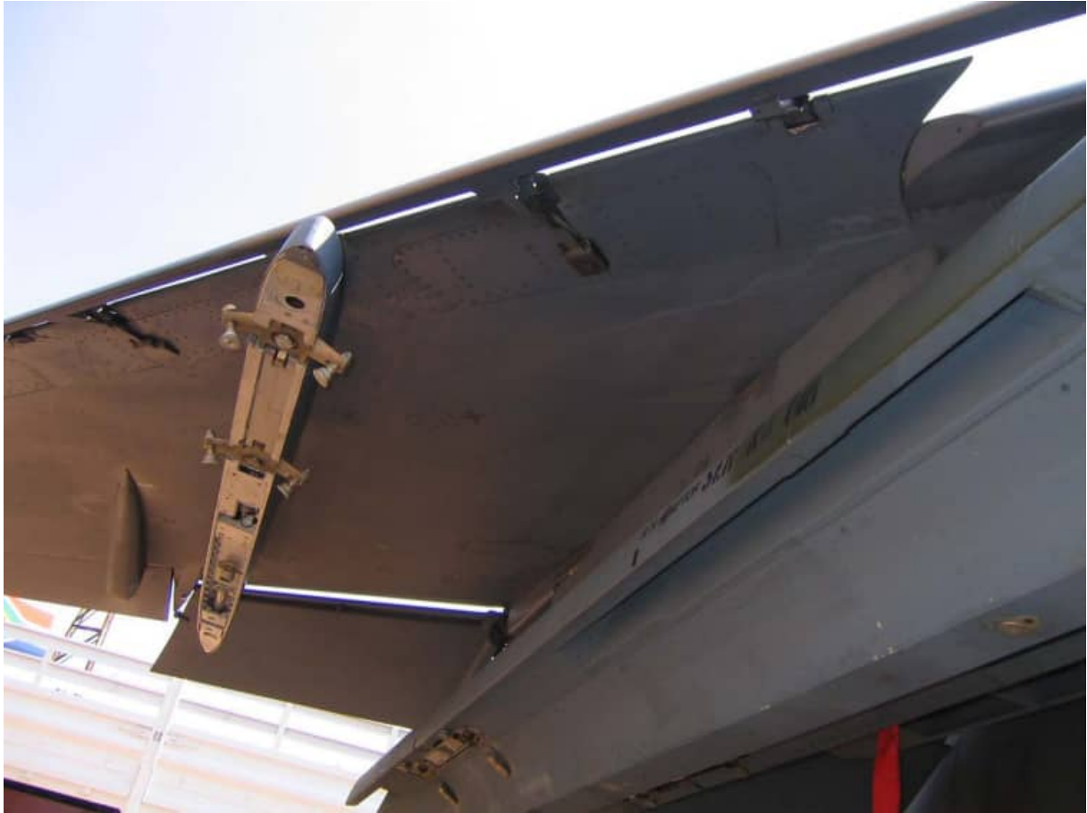
Outboard wing leading edge slat in extended position showing the aerodynamic slot. The outboard pylon is equipped to carry bombs – note the bomb sway braces. This station could also be used for the carriage of the V3S Snake air to air missile.
