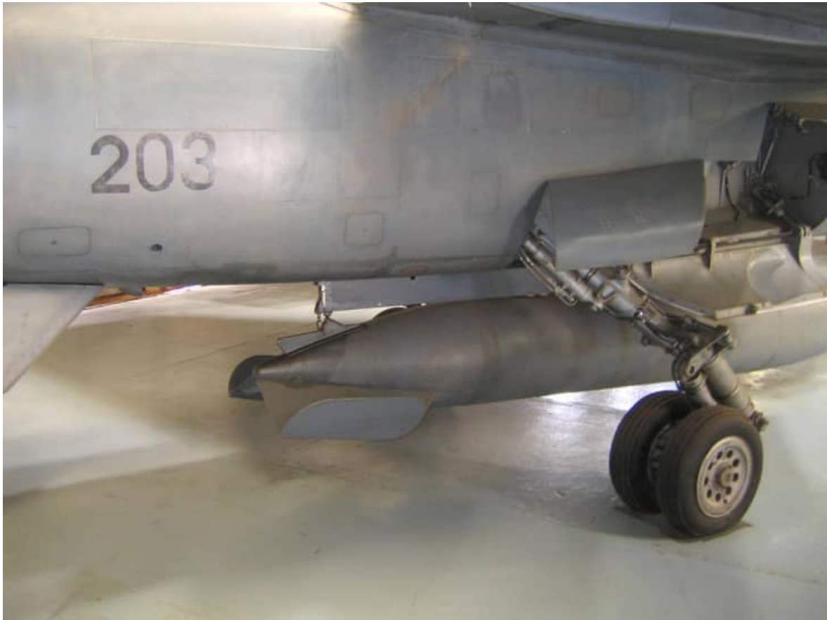
Aircraft tail number is in the standard location on the lower rear fuselage (black, 8" high.) This is typical for ALL SAAF F1s in any of the colour schemes. In this case, it has been lightly over sprayed with the base camouflage. The external fuel tank is an RP35 of 1,200 liter capacity.
