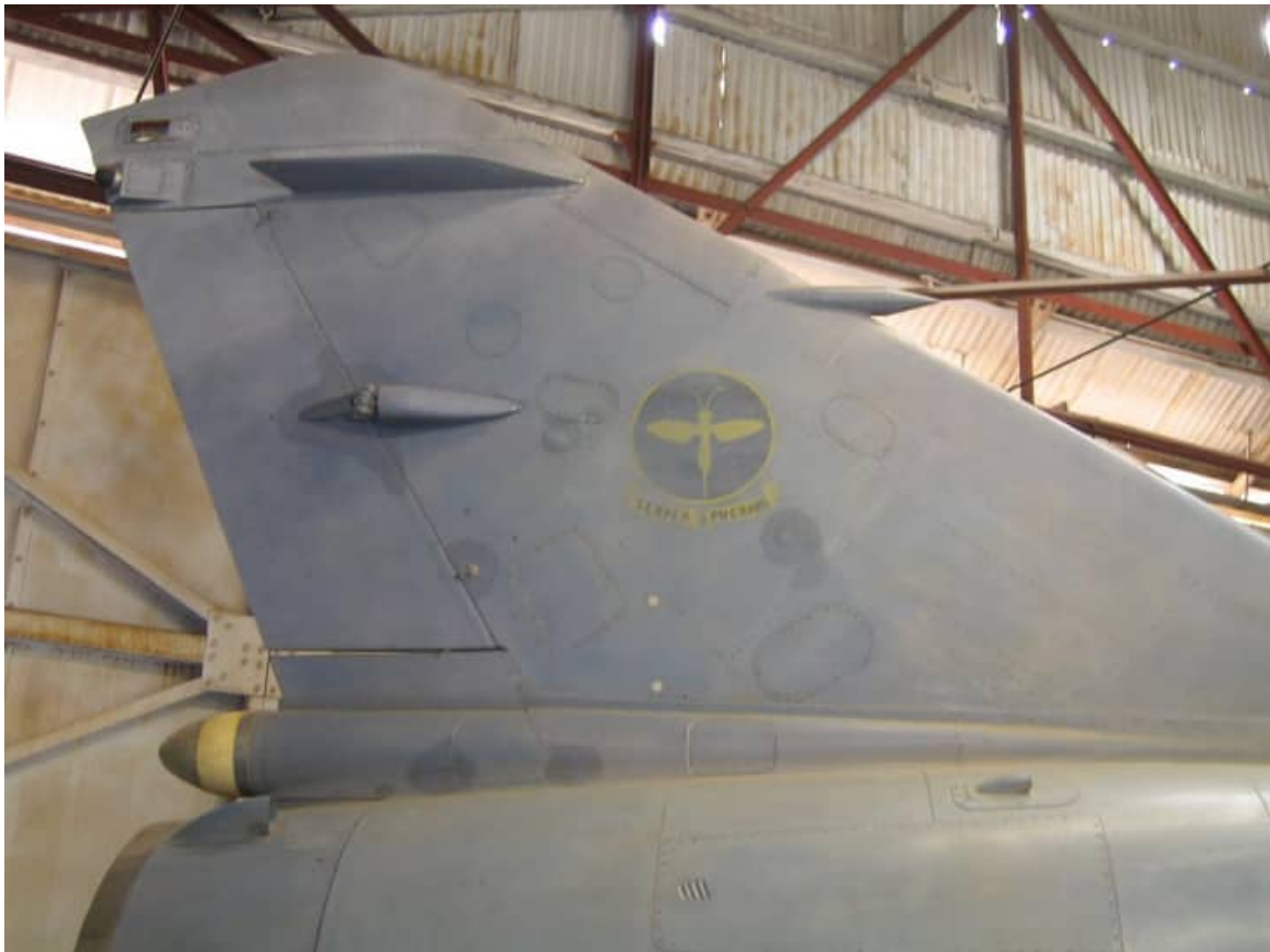
3 Squadron badge on vertical stabilizer, oversprayed with the base camouflage. One of the RWS antennas can be seen at the top left of the vertical stabilizer. Note the afterburner cooling intake at bottom left of the photo just beneath the drag chute cone. This is present on both sides of the fuselage and is common to both the AZ and CZ. The other smaller vent to the right was only present on the starboard fuselage.
