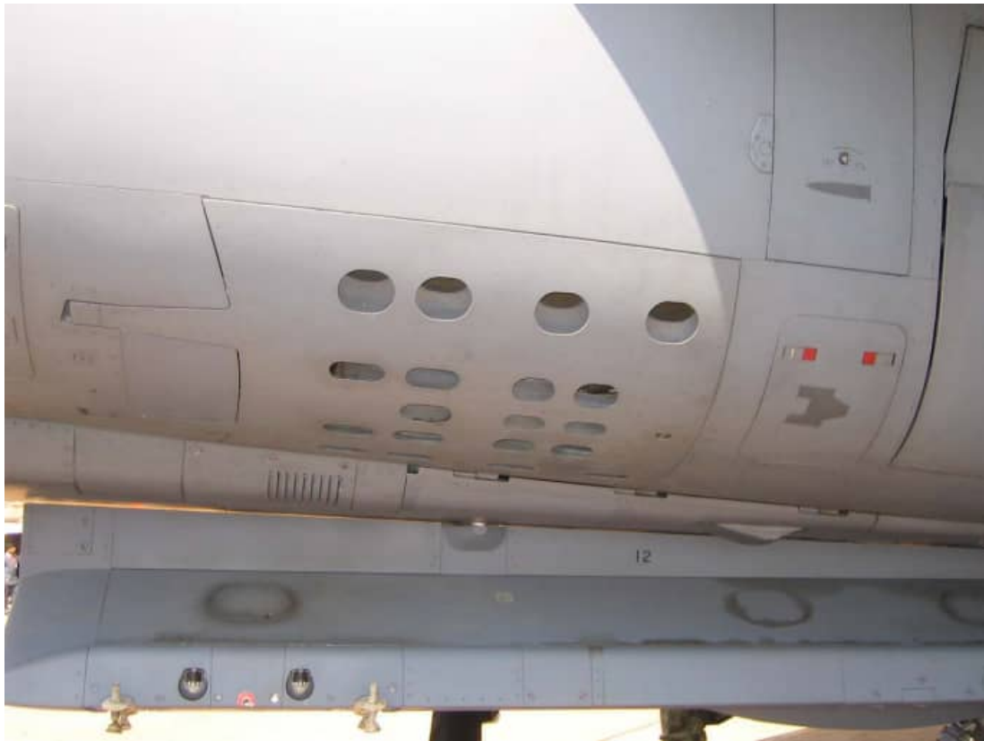
Forward end of centerline CLB4 bomb carrier showing the bomb sway braces. Bombs were carried symmetrically, unlike the configuration of the wing CLB8 / A26 4-bomb carriers shown in the image below where the bombs were staggered. Note the standard NATO symbology in dark grey.
