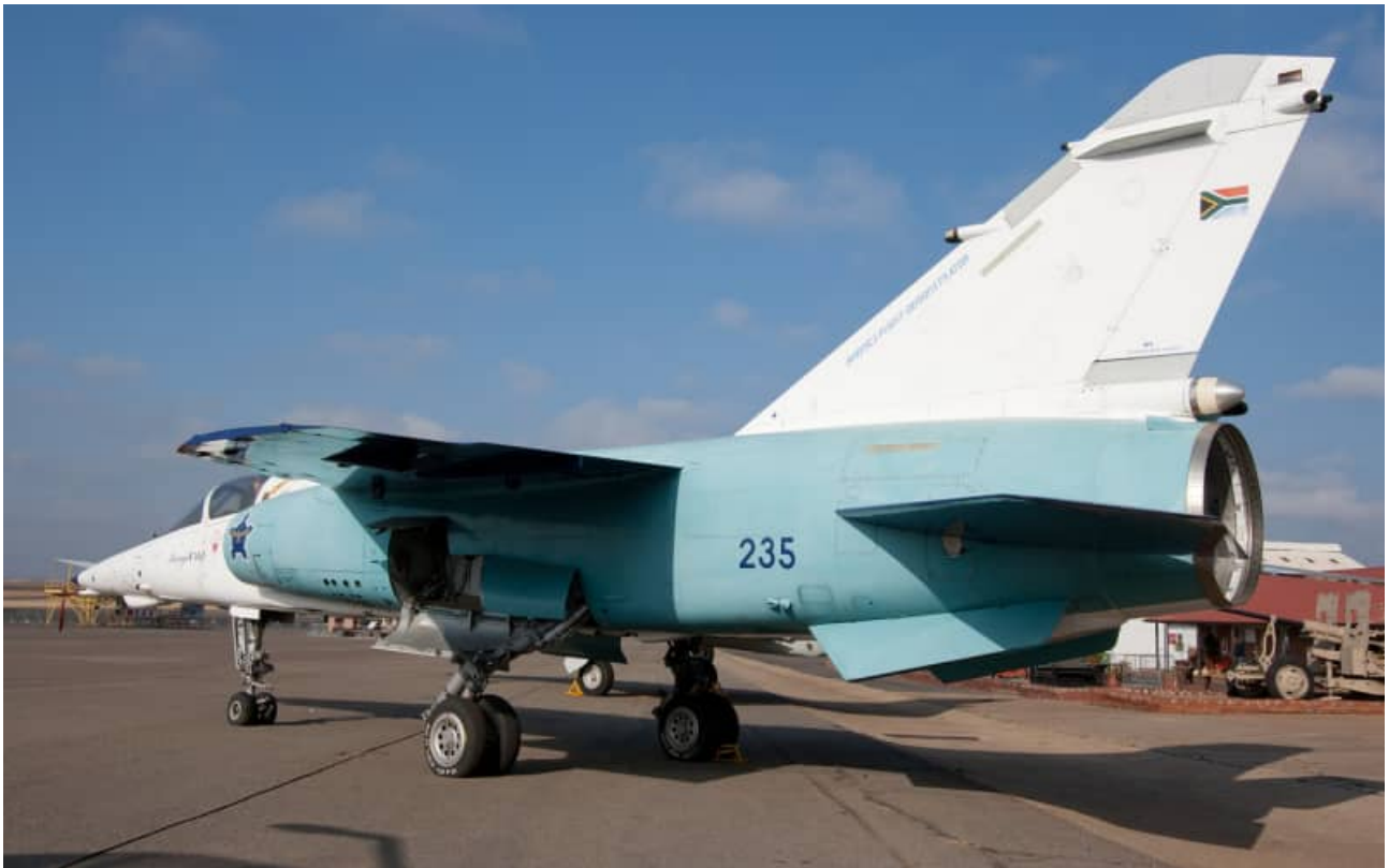
Note the angular shape of the ventral fins equipped with the RIMS chaff/flare cartridges. The two antennas on the leading edge of the vertical stabilizer are not standard for SAAF F1AZs. The same applies to the center small black antenna on the upper trailing edge above the rudder. The two larger black antennas either side of this appear to be similar to the standard RWS antennas fitted to SAAF F1AZs and CZs.
