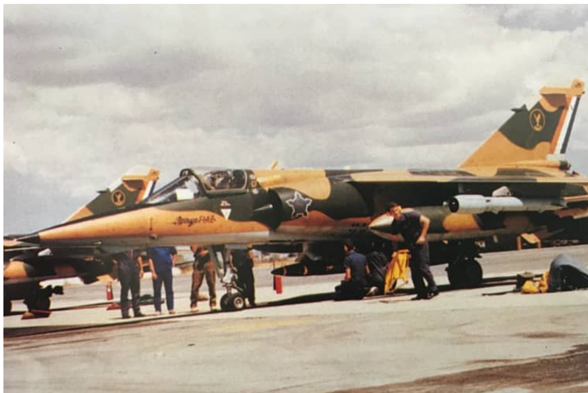
An AZ equipped with a deception ACS pod at AFB Grootfontein during the final phases of the border war. AZ's typically flew with a single deception ACS pod mounted on the port station 2 hardpoint as seen here.
