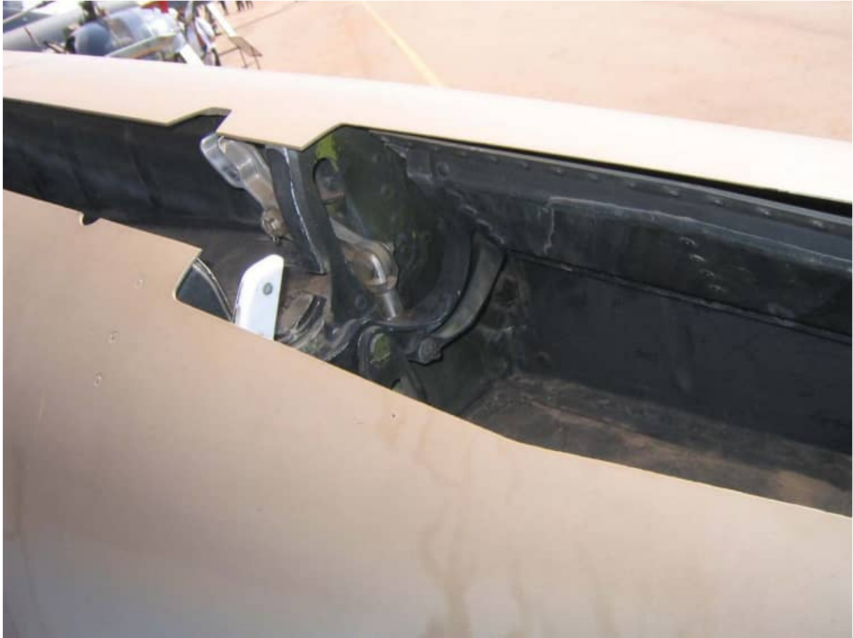
Details of the retractable refueling probe bay which is offset to starboard on the AZ nose. The bay aft cover is fixed to the probe itself. The forward bay door (to the right in the image above) rotates to the left.
