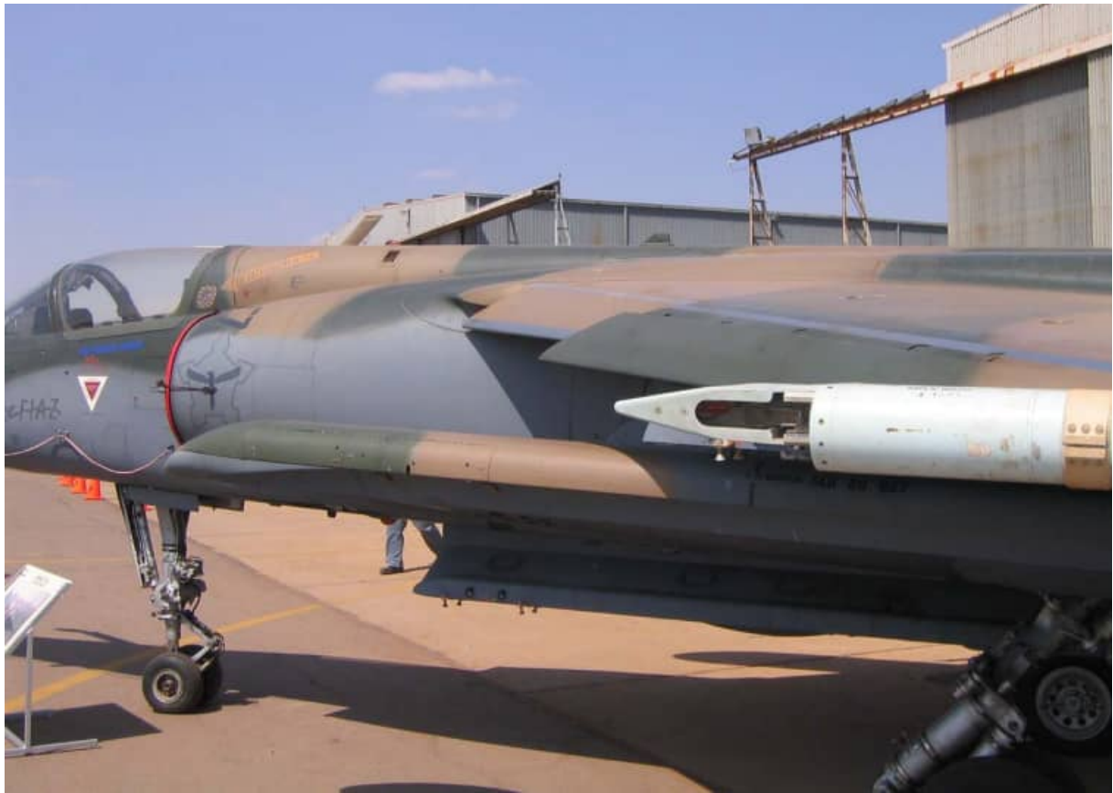
Note the grey area aft of the extended slat and the drooped flap. Note also that the grey is applied to the leading edge of the inboard flap and not the slat.
