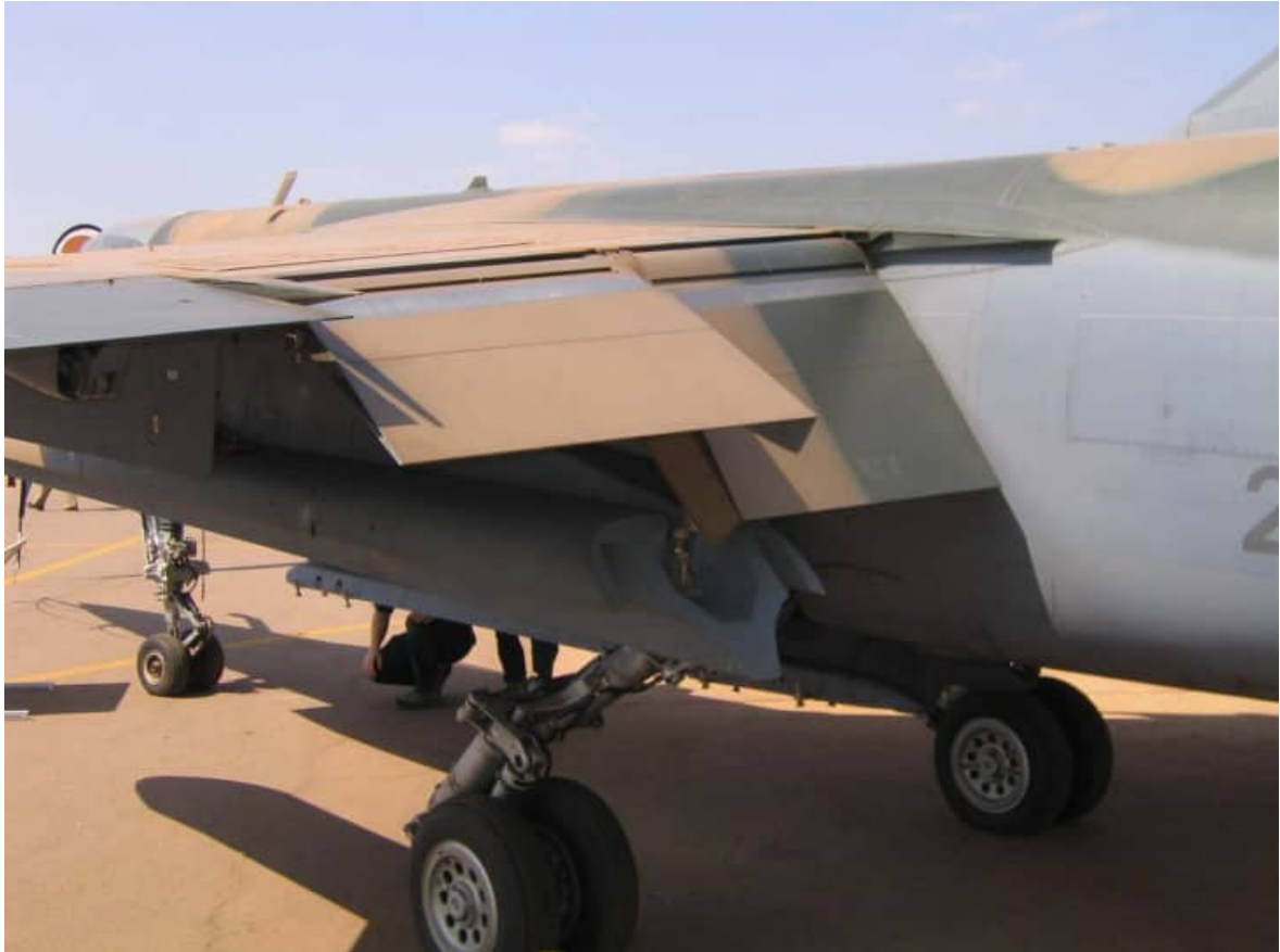
Variable droop angles of inboard and outboard double slotted landing flaps. Note the grey painted wear area on the flaps.
