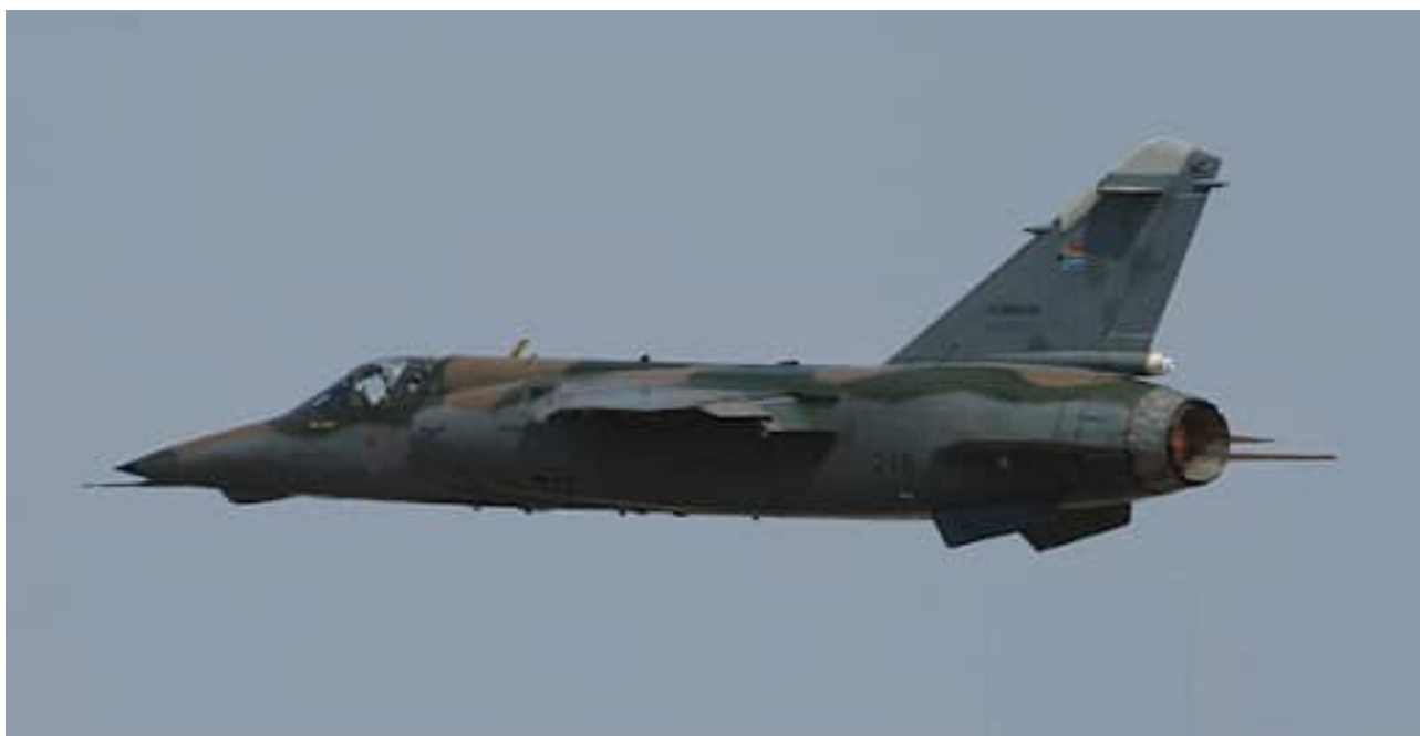
AZ #216 with Russian SMR-95 engine installed – note the different exhaust arrangement from the Atar 09K50 in the image above. #216 was the only Mirage F1 so equipped.
