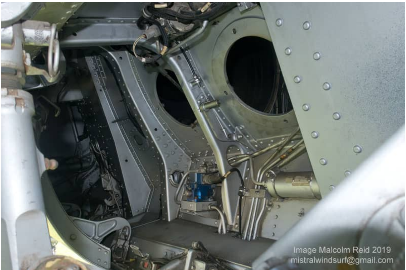
Details to note – structural ribbing and access holes between the undercarriage bay and engine bay. The covers over these access holes have been removed.
