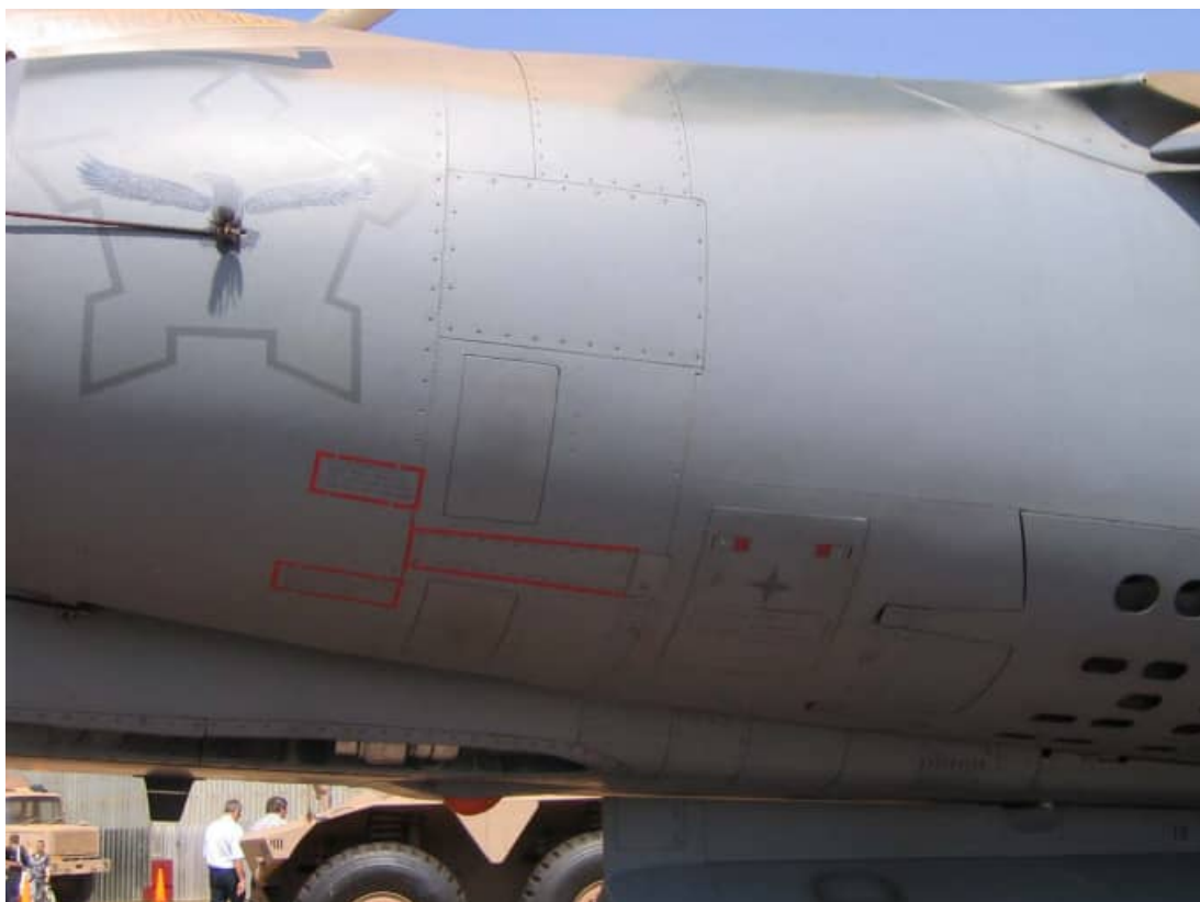
AZ nose panel detail with the refueling probe in the extended position.
