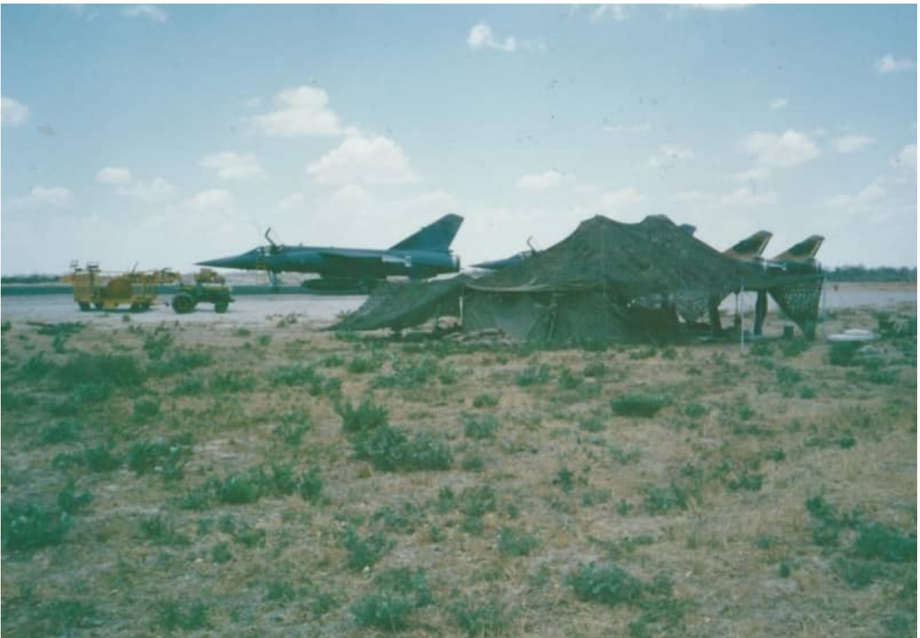
F1CZs deployed to AFB Rundu in the latter end of 1987. While not very clear, the relocated UHF antenna on the spine and the just visible “Cake Tin” antenna under the nose indicates that the aircraft has been fitted with the RWS. The rounded profile of the ventral fins however indicates that the aircraft does not have the RIMS fins installed.
