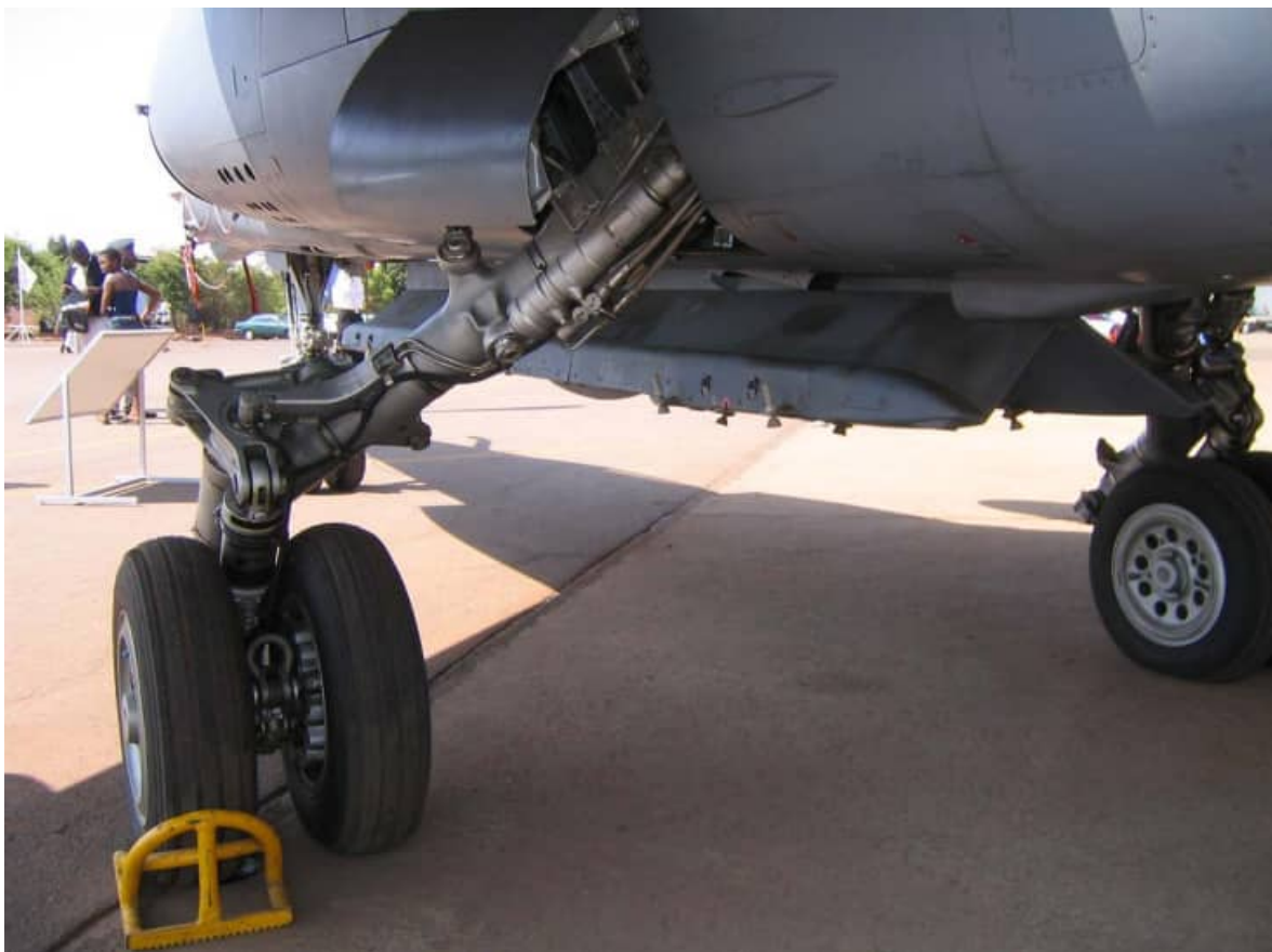
The rear end of the centerline CLB4 bomb carrier. The rear two bomb shackles were angled differently to the front two, with the rear bombs having a slightly more nose down attitude.
