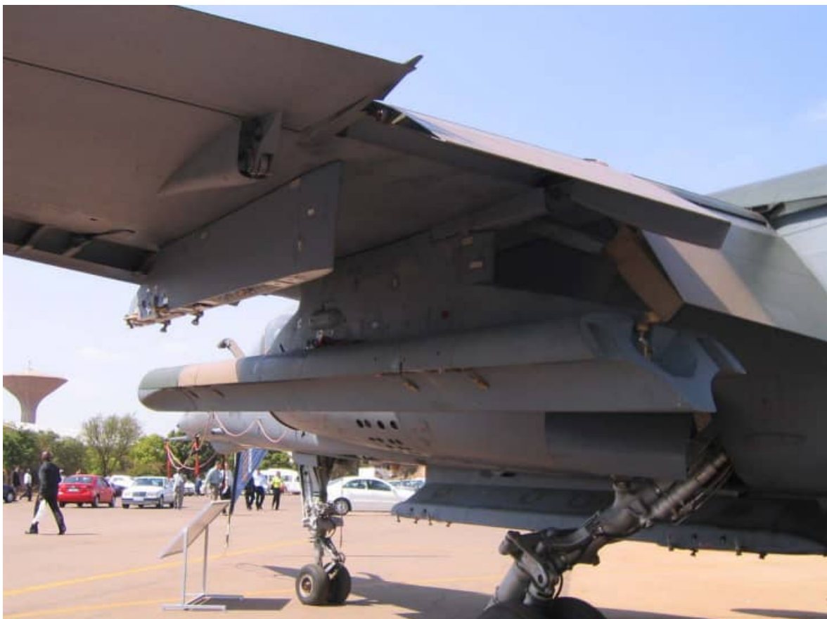
Details of the CLB8 / A26 4-bomb carrier on the wing. These are fitted to the standard F1 inboard pylon. The drooped flaps are of the double slotted type. Note the vertical strakes on the outboard edges of the flaps.
