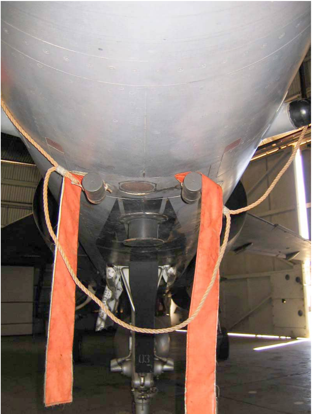
The black false canopy painted on underside is visible in this image. The cylindrical black object is the RWS CD/DF direction finding antenna fitted to the CZ. To the top right can be seen another of the RWS antennas, which are located symmetrically on the port and starboard forward fuselage. The last two digits of aircraft tail number are painted on the lower forward undercarriage door in light grey. Note that this door is slightly offset to port in relation to the nose landing gear leg.
