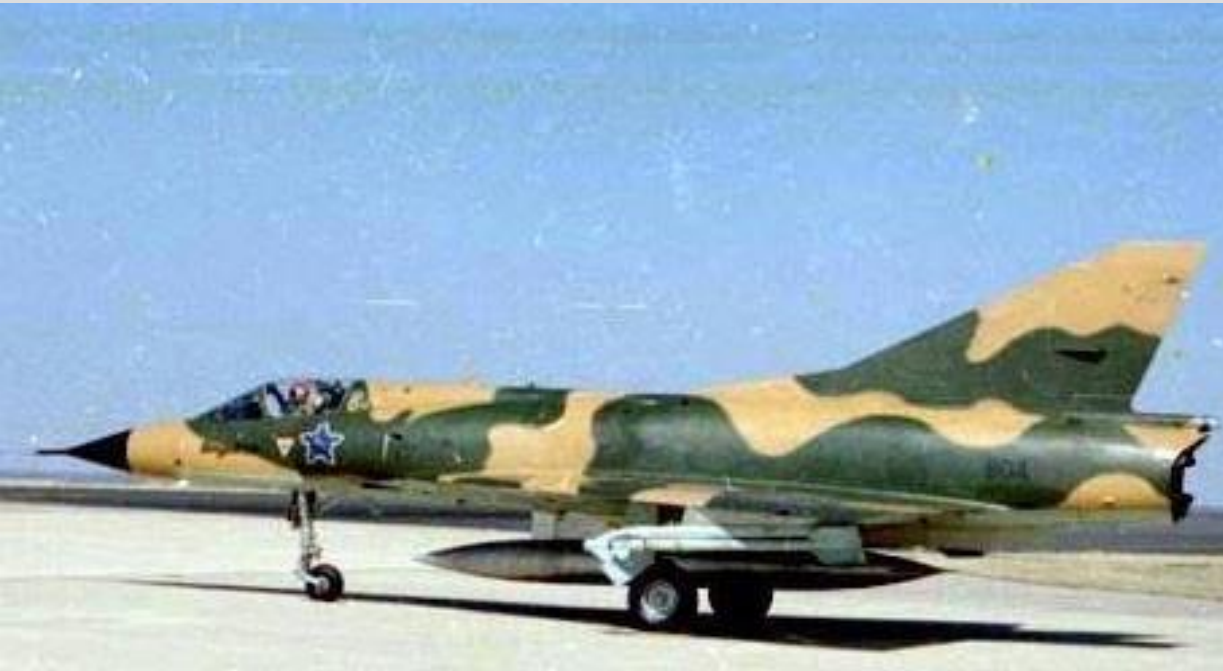
Dassault Mirage IIICZ circa 1990, stationed at Air Force Base Hoedspruit along with Dassault Mirage IIIBZs and FIAZs prior to a training sortie. This is the standard SAAF Mirage III interceptor configuration of 1 x RP825 on the centreline and a pair of V3B AAMs on the wingtips, being a blue colour denotes the V3Bs as training rounds.
