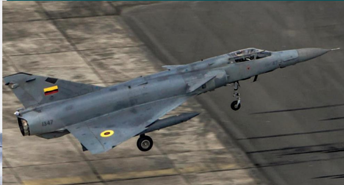
Ecuadorian Atlas Cheetah C carrying RP18R's.. Note the different style of In-Flight refuelling probe immediately behind the cockpit on this aircraft which is unique to the Atlas Cheetah C.
