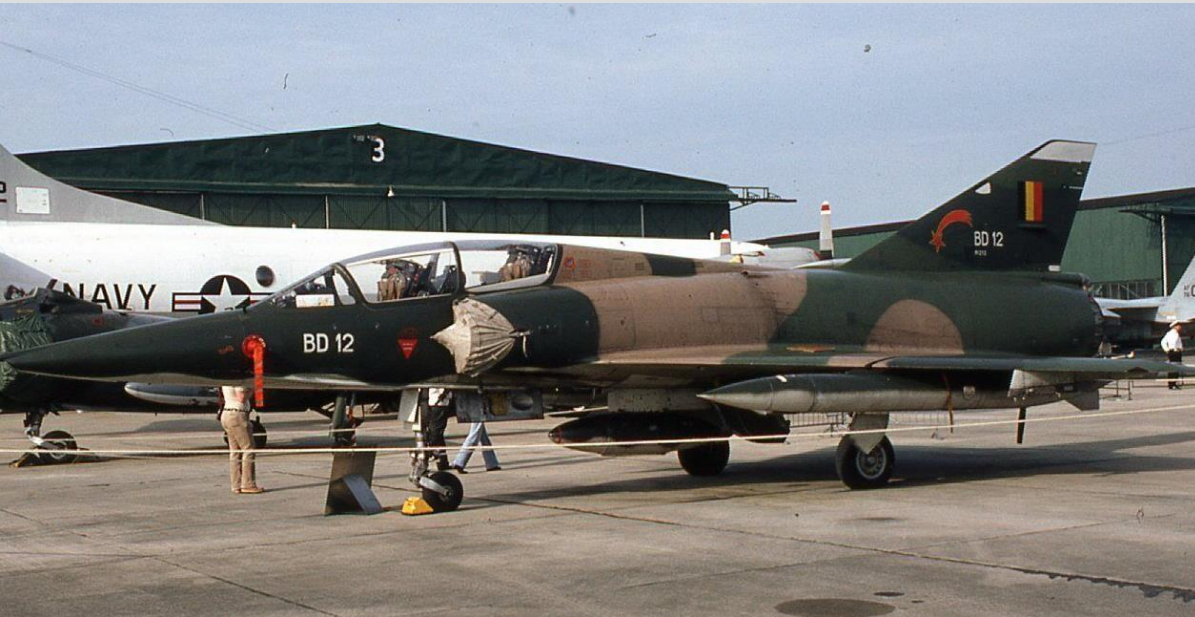
A Belgian Mirage 5BD training aircraft carrying RP18R underwing and what appears to be a "luggage" pod on the centreline pylon.
