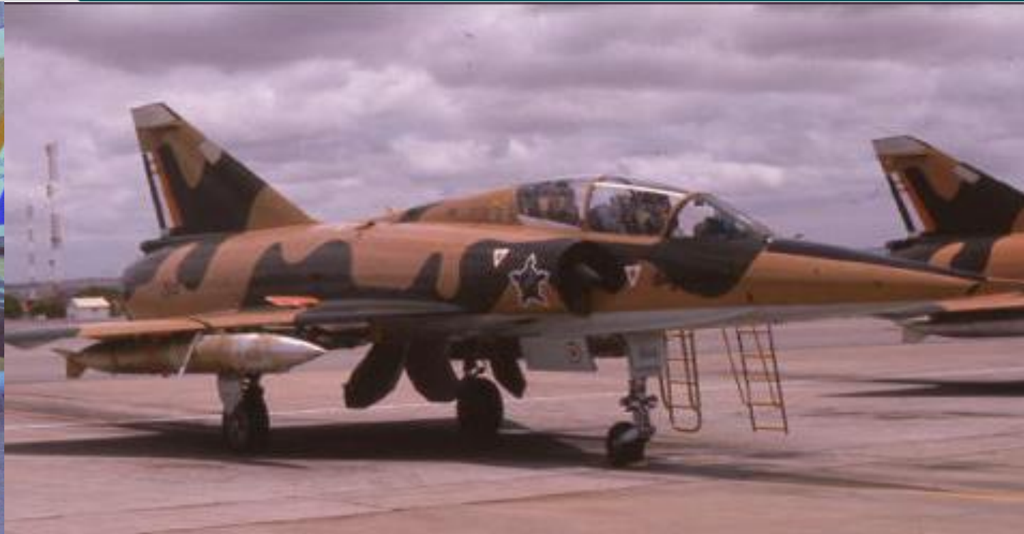
Another glossy South African Mirage, this time a IIIDZZ of 85 Air Combat School carrying a pair of RPI8R's on each inner wing station. Note the yellow/orange colour on the tank, this was a protective coat.
