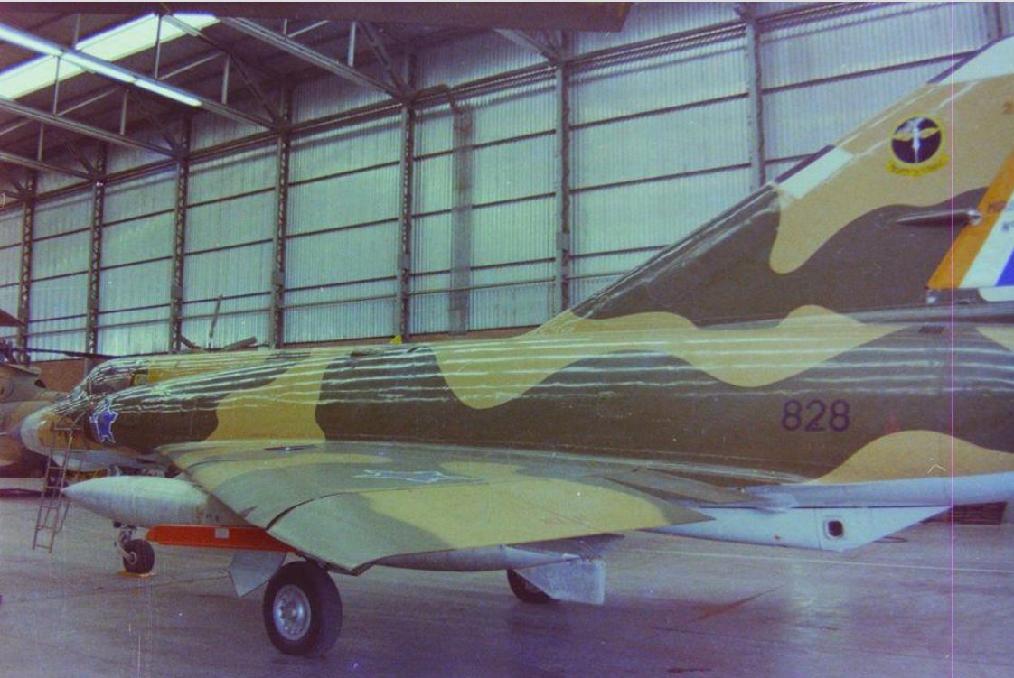
A very glossy South African Mirage IIIIEZ with RPI8R and brightly coloured AAM launch rail.
