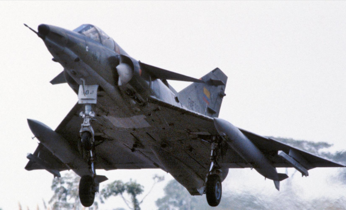
Ecuadorian IAI Kfir C2 with RP18R's and a pair of empty Python 3 Launch Rails on the outer wing stations.
