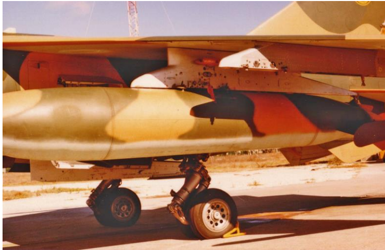
The Alkan 915/6 and CLB-30 pylons of the Mirage F1AZ.
