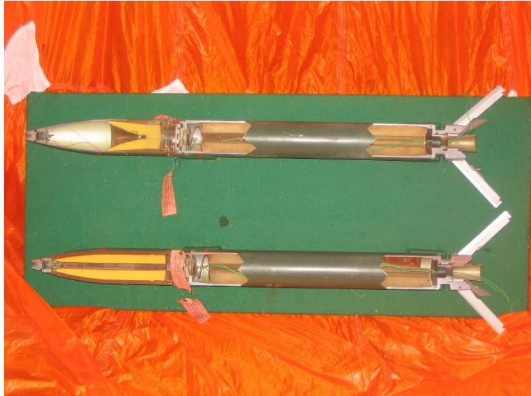
A cut through display of the 68mm rockets used in the Matra 155 pods.
