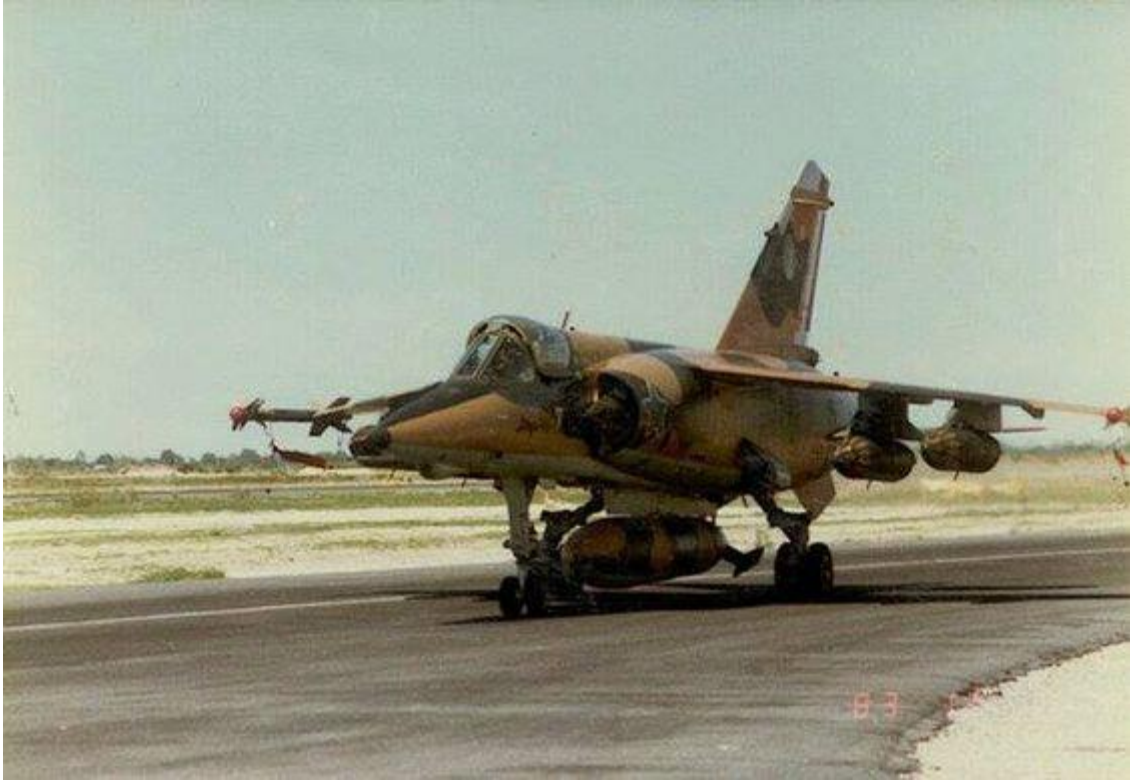
A Mirage F1AZ at AFB Ondangwa, armed with four Matra 155 rocket pods below the wings. Note the cones that cover the front of the pods.
