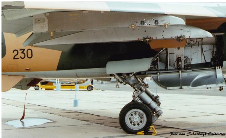
The Alkan 915/6 and CLB-30 pylons of the Mirage F1AZ.
