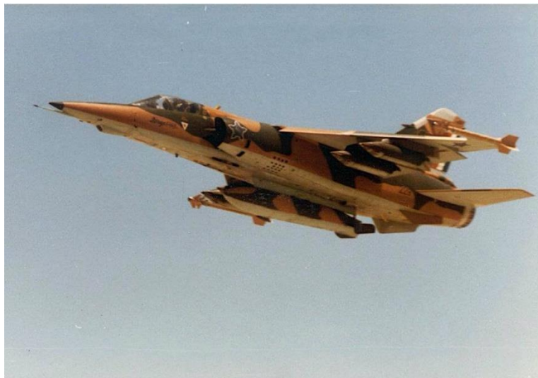
A Mirage F1AZ armed with four 68mm Matra 155 rocket pods below the wings.
