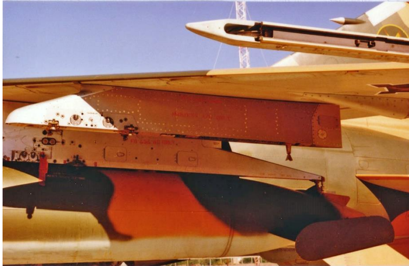
The CLB-30 pylon as used on the outboard stations of the Mirage F1AZ.
