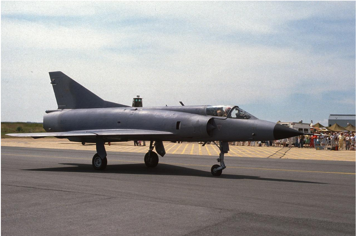
Starboard view CZ #807. In this instance, the nose cone is similar in colour to the lighter blue camouflage colour. The toned down intake Castle and ejection warning triangle are visible. However, it appears that the 2 Squadron badge is not present on the vertical stabilizer. #807 has the Compact Radar Warning System (CRWS) installed as can be seen in this image by the round antennae on the nose and atop the vertical stabilizer.
