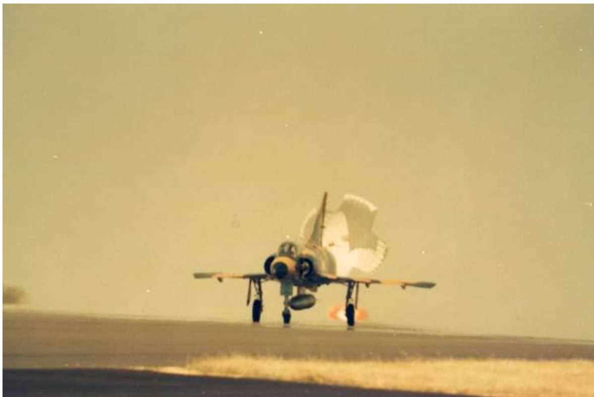
This is not the best quality image but it's rather an evocative image of a CZ trailing its drag chute. It is equipped with the 1,100 liter RP825 fuel tank. The protuberances beneath the wings are the aerodynamic fairing for the elevon actuators.
