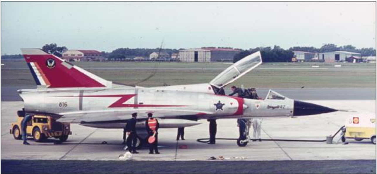
Another image of BZ #816 in delivery scheme. RP18R 500 liter fuel tanks are carried on the wings.
