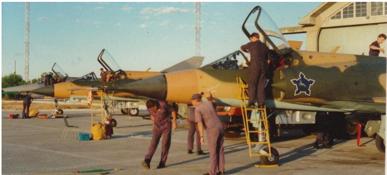
CZ forward fuselage showing soft edge matt camouflage (original pattern). Details to note include : weathered dark grey radome with gloss black backing ring; solid buff nose cone (a distinct darker hue than the fuselage buff); Castle well forward on the air intake. Note that the intake bullet is painted green and that the camouflage wraps into the leading edge of the intake and the splitter plate. Mirage III CZ no longer appears on the forward fuselage. The white text just above the ground crewmember's hand is unidentified and is not standard. The CZ in the background appears not to have the Castle on the intake. In this case, the buff on the nose cone is similar in hue to the buff on the rest of the aircraft. Both CZs have the blade antenna on the fuselage spine aft of the canopy. The grey aircraft in the background is an RZ as denoted by the camera windows and the doppler fairing beneath the nose.
