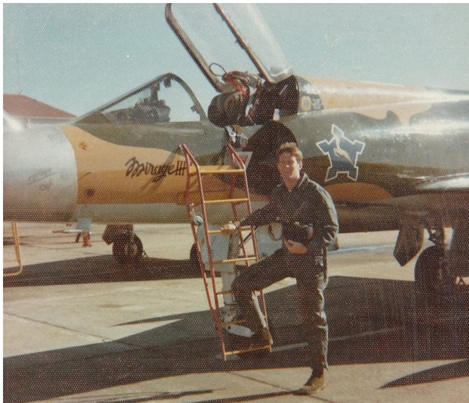
This CZ in hard edge buff/green camouflage has an unpainted natural metal nose cone installed. The text "Cyrano CSF" on the nose cone indicates that the radar nose is fitted. Note the revised location of the ejection seat warning triangle when compared to the previous image.
