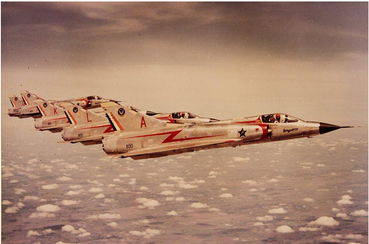
A magnificent image of a flight of CZs showing the complete set of markings over unpainted natural metal. The ejection seat warning triangles are still present on the engine intakes.
