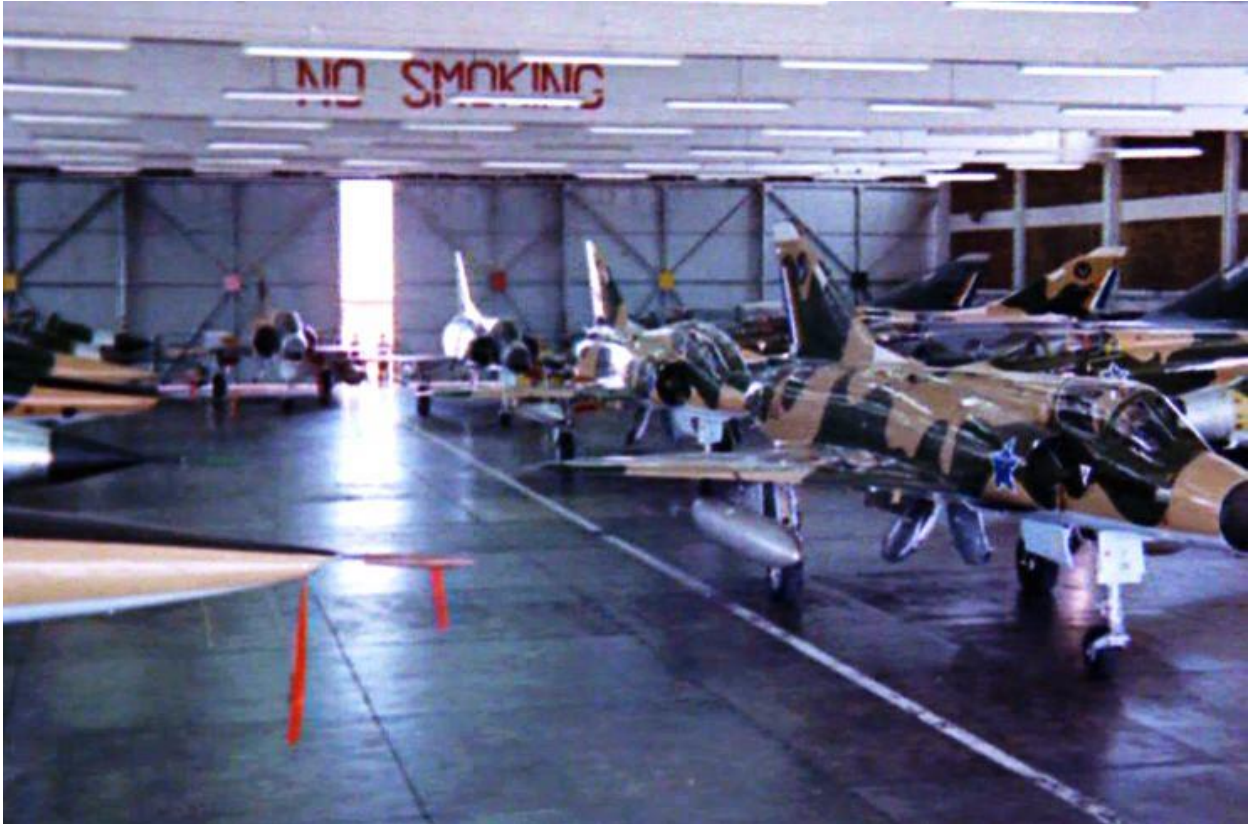
A hangar full of Mirages. The CZ in the right foreground has the camouflaged radar nose cone in buff / blue with a hard edge between the two colours. The aircraft behind this is a BZ (filleted vertical stabilizer), with another CZ behind that. The aircraft at the front left is a DZ or DZZ as depicted by the chisel shaped tip to the nose. Behind this is either a CZ or an EZ with unpainted nose cone. Behind this either an RZ or RZZ as identified by the camera window on the nose.
