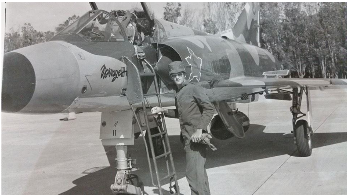
CZ #811 in hard edge buff/green camouflage with radar nose and full buff nose cone which is darker than the buff on the rest of the aircraft. Text on the upper air brake appears to be "BLY AF". The store on the centerline hard point is unidentified but may be a target-towing pod. Note the little yellow/black-striped door beneath the wing indicating that ground crew have manually opened the main gear doors.
