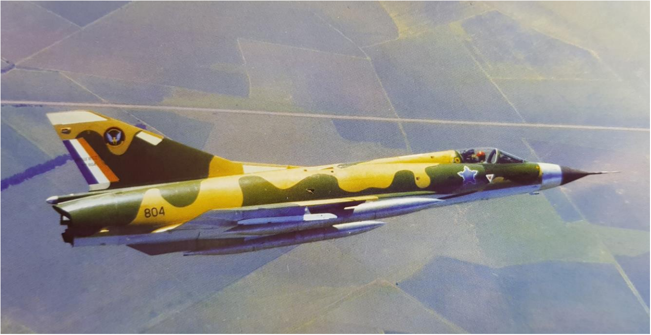
CZ #804 in gloss hard edge buff/green camouflage with full markings. The radar is installed with an unpainted natural metal nose cone. #804 has RP18R fuel tanks on the inboard wing hard points and missile launch rails on the outboard wing pylons.
