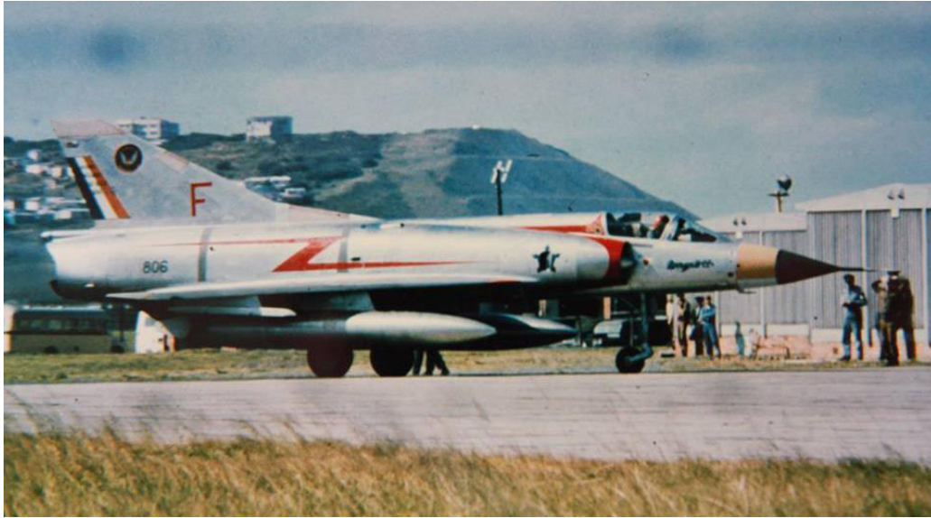
CZ #806 with a radar nose with nose cone painted in the later gloss buff upper/grey lower colours. Note how faded the black leading edges to the various antennae panels on the vertical stabilizer are.
