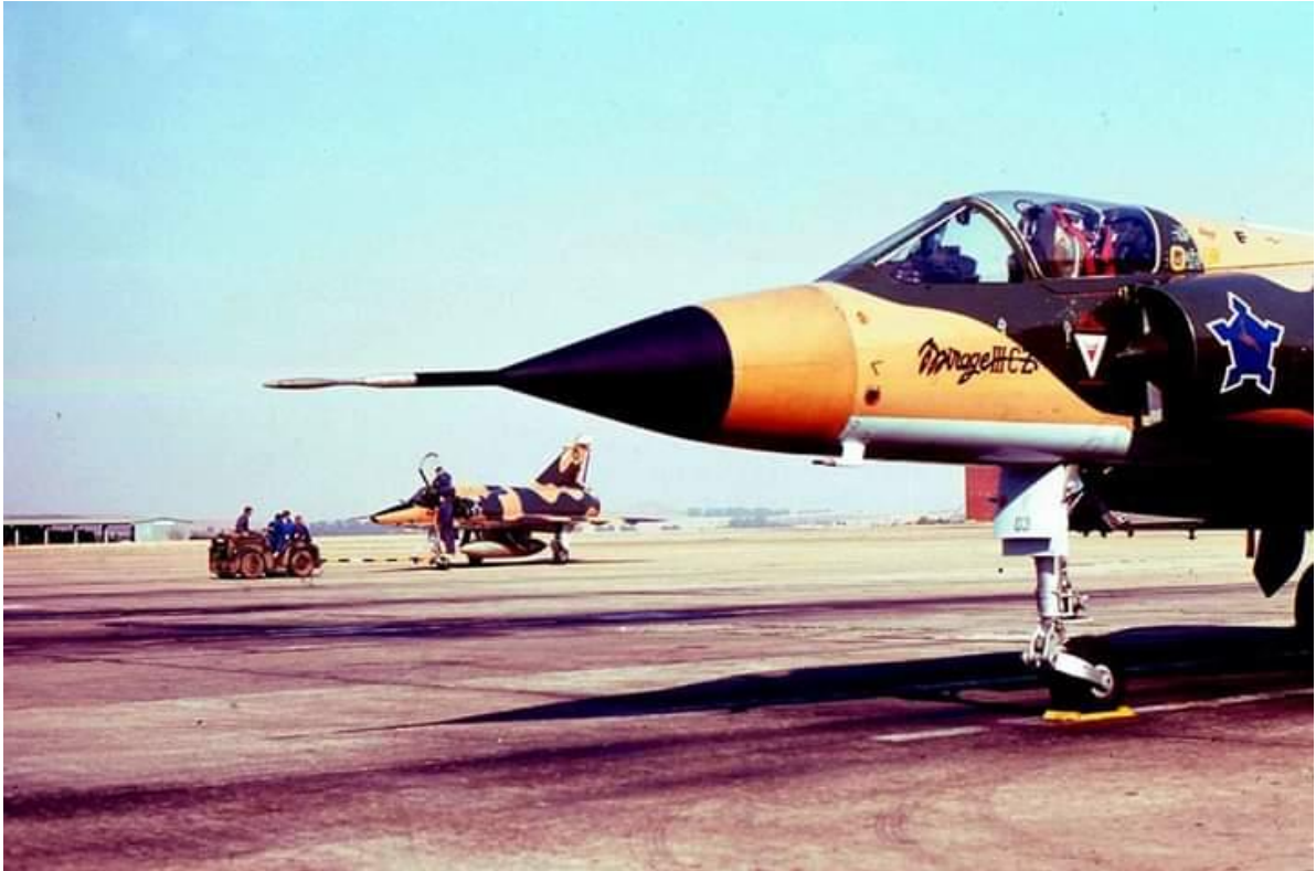
CZ in hard edge buff/green camouflage fitted with radar. In this case, the nose cone has been painted entirely in buff, which is a darker hue than the rest of the airframe. The text "Cyrano CSF" does not appear on the nose cone. Note the extension of the black onto the forward part of the pitot probe. The aircraft in the background is an R2Z
