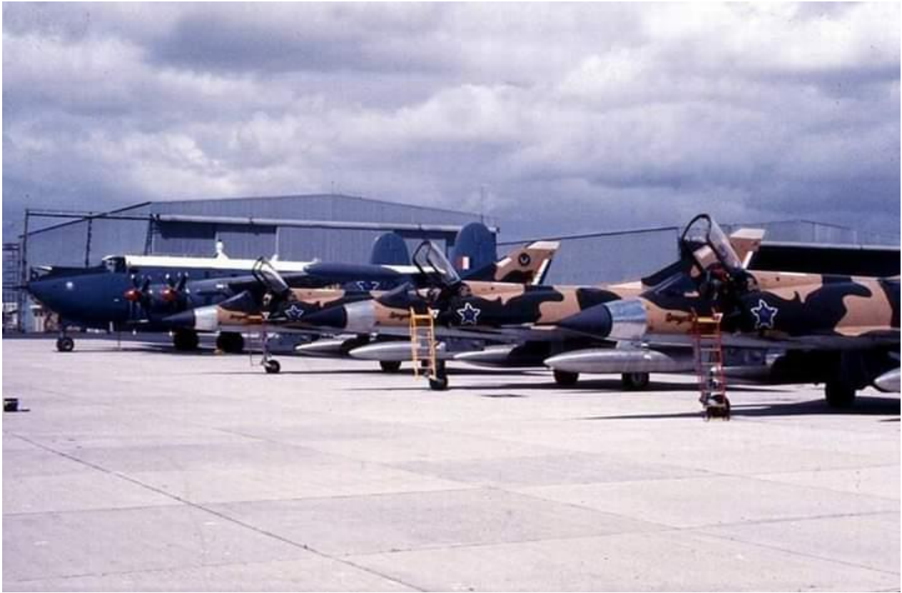
Neat line up of three CZs, possibly at Ysterplaat Air Base based on the presence of the Shackleton MR.3 in the background. Note how shiny the natural metal nose cones are – they appear to have been polished. All three CZs are in the hard-edged buff/green camouflage with what appear to be full markings. All three are carrying the 1,300 liter RP62 wing tanks.
