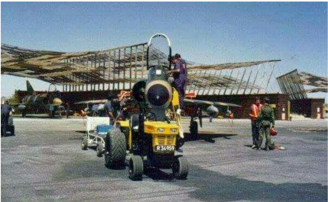
Two Mirage IIICZs at Ondangwa Air Base. Note the black radome on the aircraft in the foreground and the camouflaged nose of the aircraft under the shelter, likely indicating that the latter CZ has a "ballast" nose fitted. The aircraft in the foreground is fitted with air to air IR missiles (likely AIM-9B Sidewinders) on the outboard wing pylons and what look to be 110G wing tanks which were equipped with shackles for two bombs which could be carried in tandem beneath the tank.
