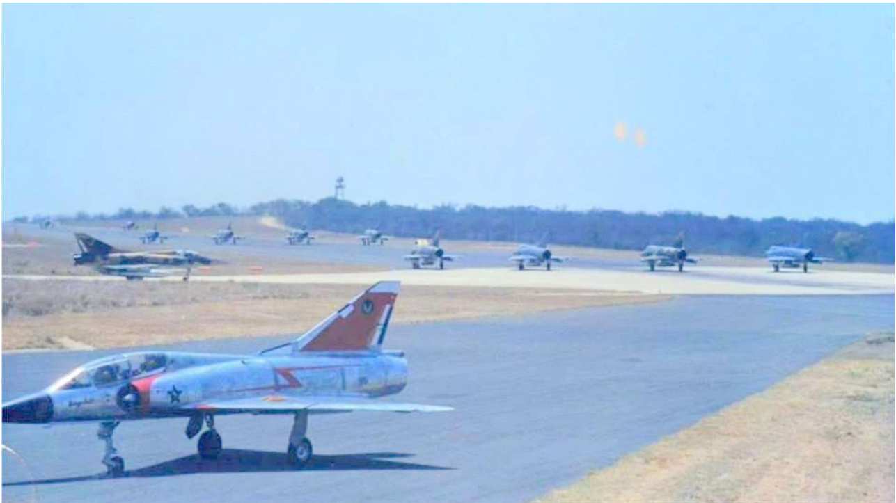
This is a really interesting image of a gaggle of Mirage IIIs. In the foreground is BZ#816 in unpainted natural metal delivery scheme seemingly going in the opposite direction to all the others. #816 shows the black nose cone. The aircraft at left (above #816) is either a two seat DZ or D2Z in early gloss hard edge buff/green camouflage. It carries RP62 wing tanks. To the right of this (from left to right) are a camouflaged CZ or EZ , a blue/grey CZ, another camouflaged CZ or EZ and another blue/grey CZ. All four aircraft carry the RP825 centerline fuel tank.
