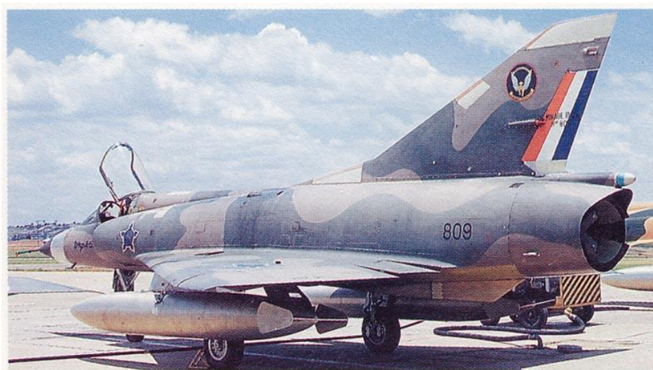
CZ #809 in the experimental dark brown / green camouflage. Note that this appears to wrap around the forward and rear fuselage underside. The ventral fin and ventral fairing seem to be painted in the yellow chromate primer. The presence of Castles on the upper wing would indicate that these have likely also been applied to the lower wing.
